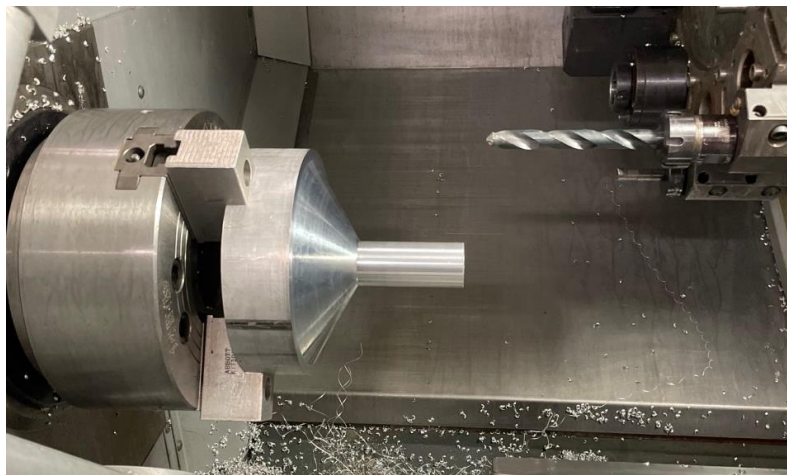
Figure 17: Operation 2: Final Funnel Exterior
