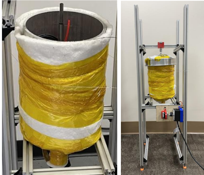
Figures 23 and 24: Completed Oven Assembly
