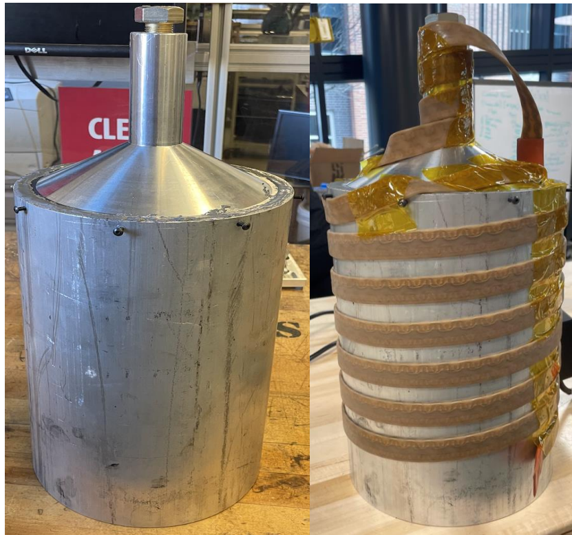
Figures 21 and 22: Beginning of Oven Assembly (left) and applied resistive wire (right)
