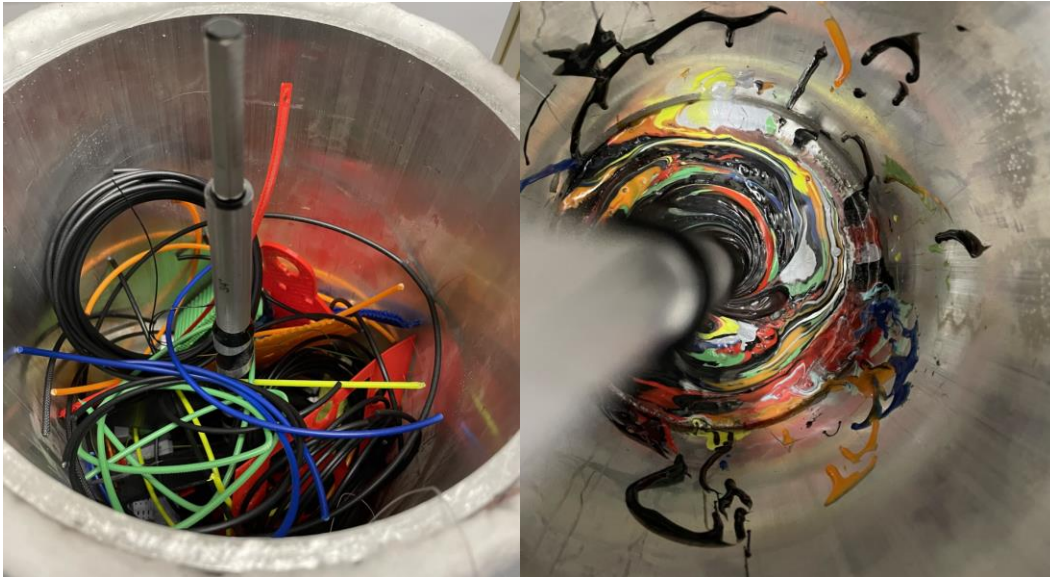
Figures 41 and 42: Before and After of Plastic in the Oven in Extrusion Test 1
