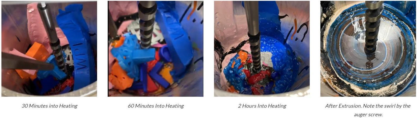
Figure 47: Pictures from within the oven during Extrusion Test 2's melting (pictures 1 and 2) and Extrusion Test 3's melting (pictures 3 and 4). The swirl in the final picture indicates that mixing was occurring within the oven.
