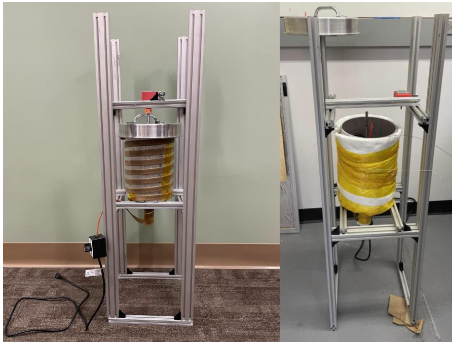
Figures 39 and 40: The machine before (left) and during (right) the first extrusion test. Between the two pictures, the insulation was wrapped over the resistive wire.
