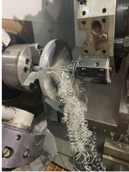
Figure 19: Interior Funnel Machining Progress Picture
