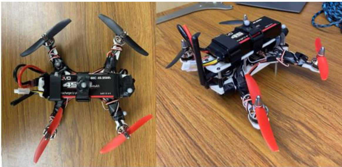
Figure 10: Fully Assembled MAV (without ODROID microcontroller)
