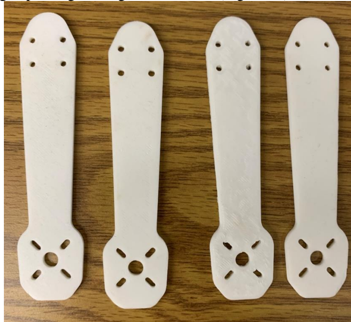
Figure 22: 3D Printed Motor Arms
