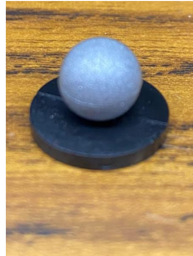
Figure 27: Vicon Reflective Tracking Marker
