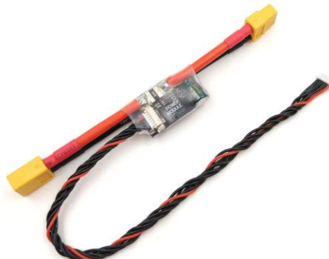
Figure 15: Pixhawk 5.3V Power Module
