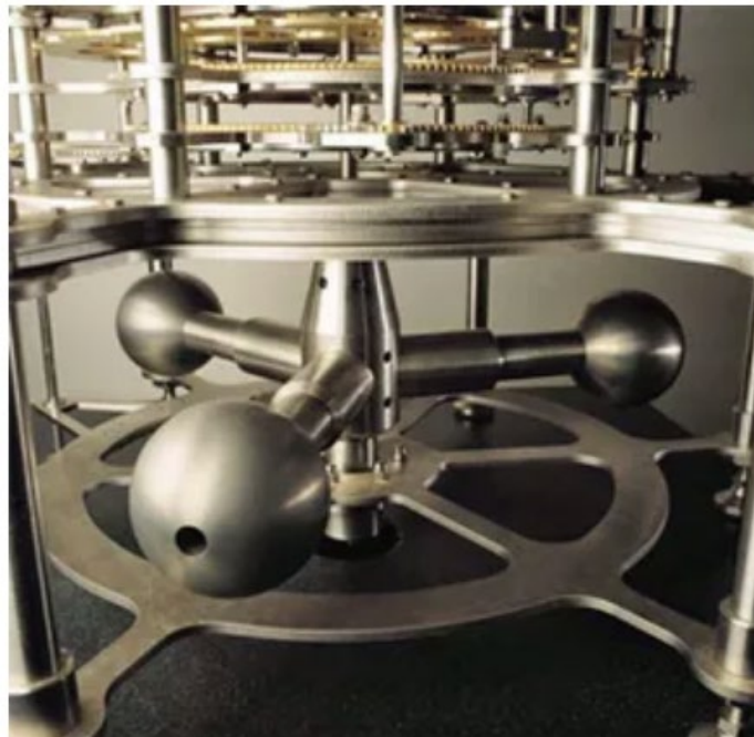
Figure 37. The torsional pendulum that will maintain the timing of the 10,000 Year Clock. Source: URL .
