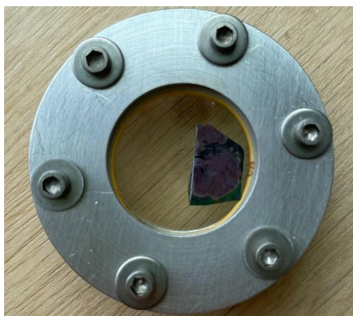
Figure 17. Thin film sample sealed between quartz rounds.
