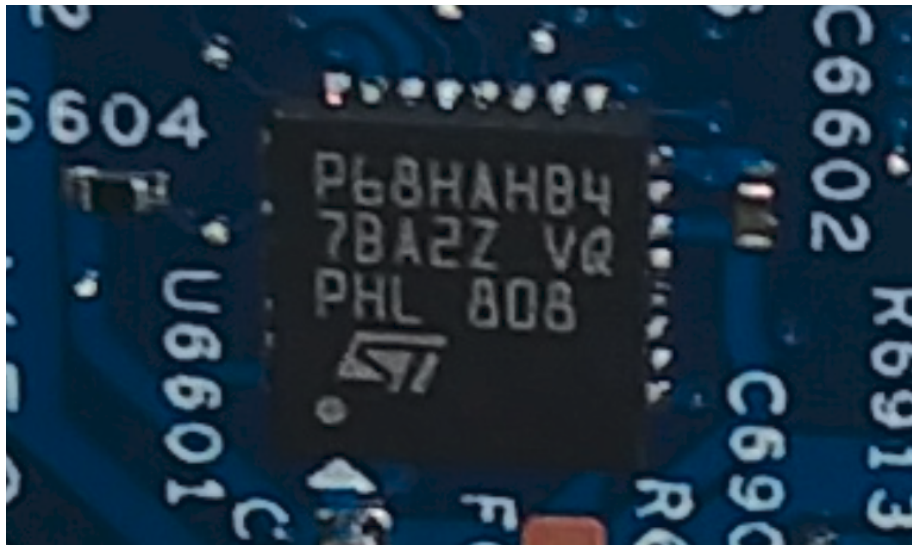
Figure 5.15: The layout of the vulnerable TPM chip on the Lenovo T580 mainboard.
