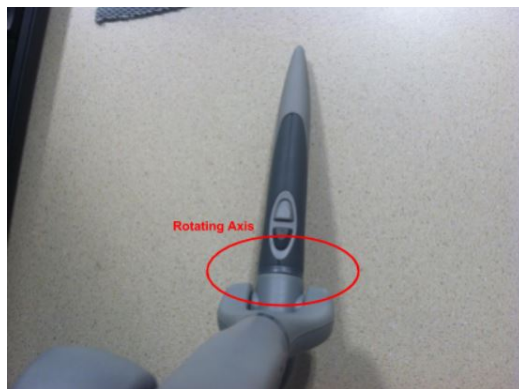
Figure 40: Haptic device tool, buttons, and rotating axis
