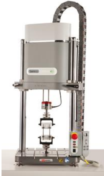
Figure 11: ElectroPuls E1000 All-Electric Test Instrument ("Testers & Stands | Chatillon Force Measurement," 2014)
