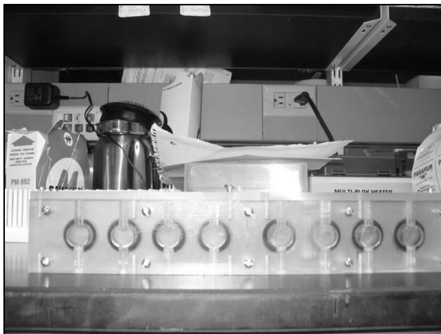
Figure 4: Equilibrium dialysis apparatus (EDA)
