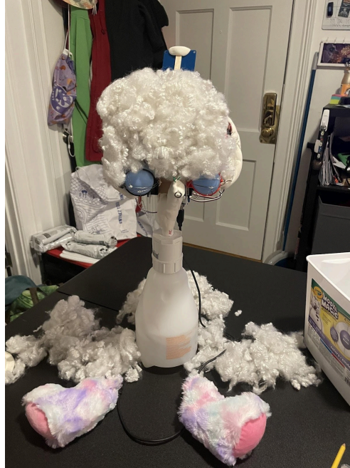
Figure 24. The animatronic during the process of shaping and attaching the skin. The stuffing was used to give the robot the desired shape while still allowing the servos to move without interference.
