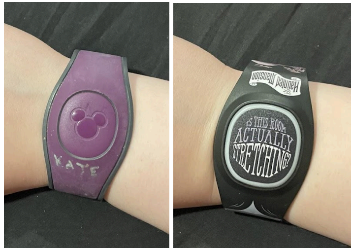
Figures 15 & 16. A MagicBand v2 and a MagicBand+. The MagicBand+ is larger and thicker than the v2, and also possesses the ability to light up in the center.
