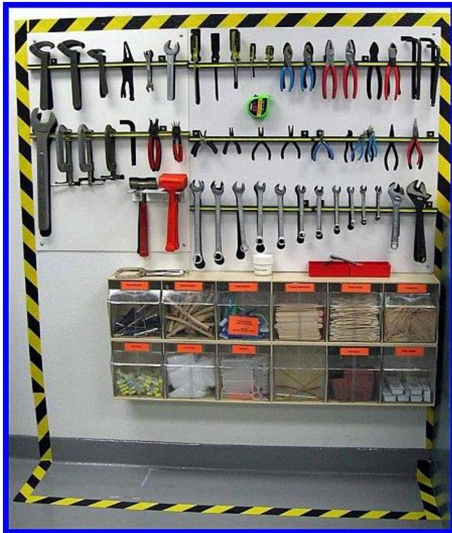
Figure 41: An example of a shadow board in a workplace (Superfactory, 2008)
