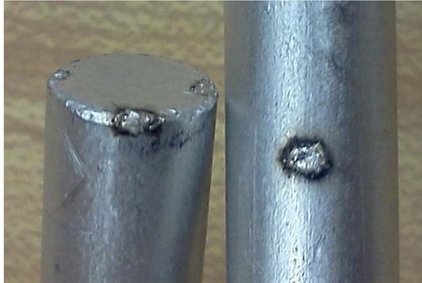
Figure 5.10 - Aluminum bars welding marks
