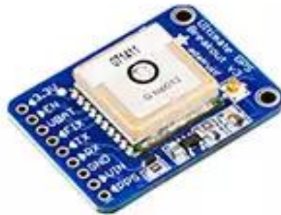
Figure 14: FGPMMPA6H GPS with Adafruit Breakout
