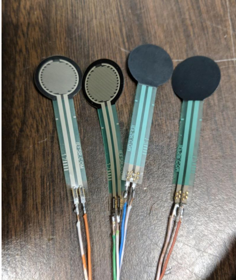
Figure 21: FSRs soldered to leads of a Cat 5 cable
