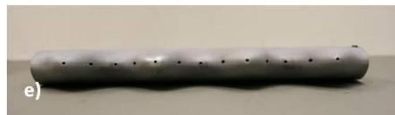
**Figure 12: a) Dye injection system; b) dye valve connected to baseline foil; c) dye valve connected to 4L foil; d) leading edge of baseline foil with dye ports; e) leading edge of 4L foil with dye ports.**
