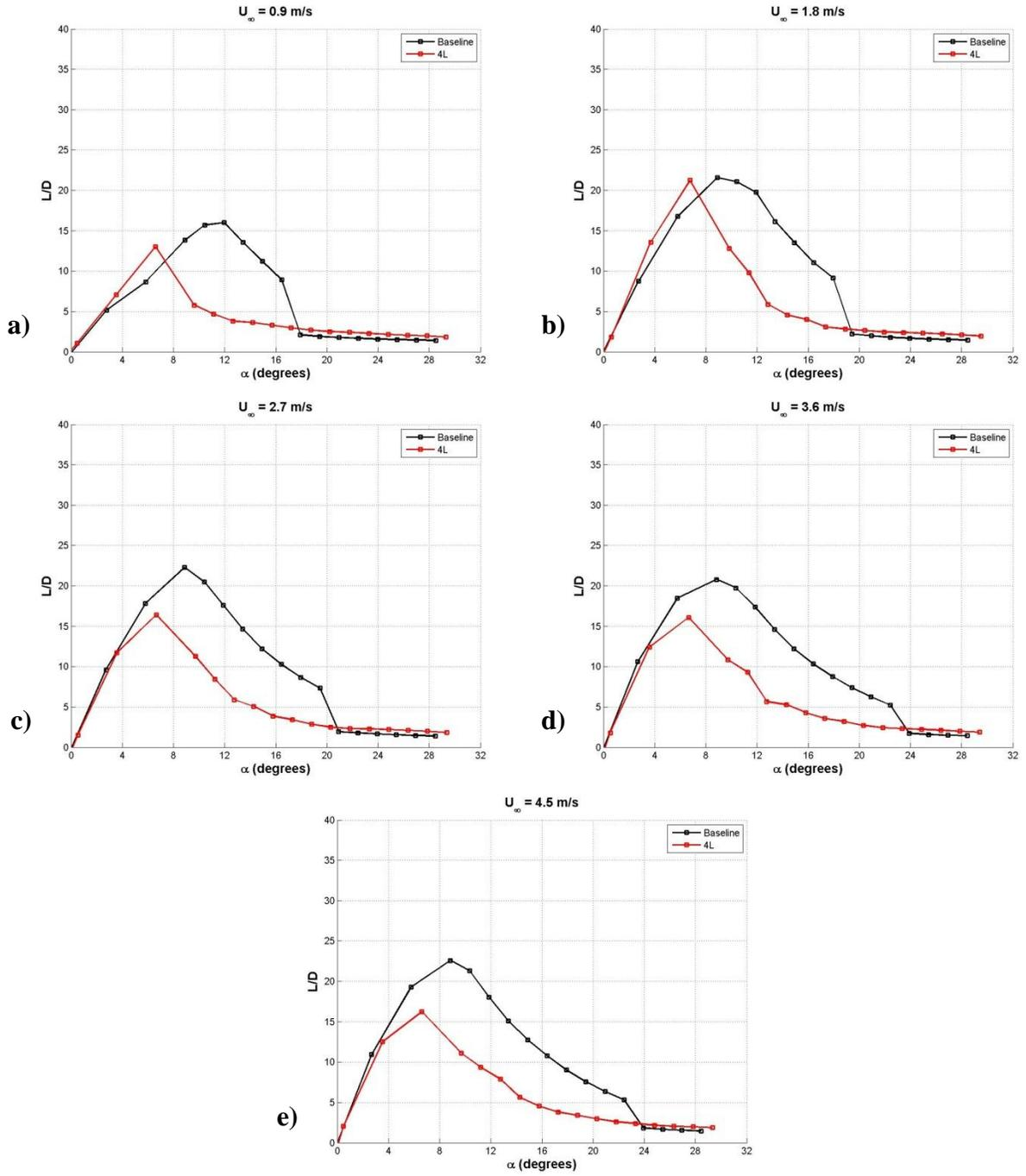
**Figure 23: Infinite-span planform L/D ratio. a)  $Re_c = 9.0 \times 10^4$ , b)  $Re_c = 1.8 \times 10^5$ , c)  $Re_c = 2.7 \times 10^5$ , d)  $Re_c = 3.6 \times 10^5$ , e)  $Re_c = 4.5 \times 10^5$ .**
