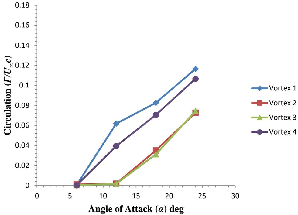
Figure 71:  $\Gamma$  as a function of  $\alpha$  at a chordwise spatial location of  $x/c = 0.36c$ .  $U_\infty = 1.8$  m/s.
