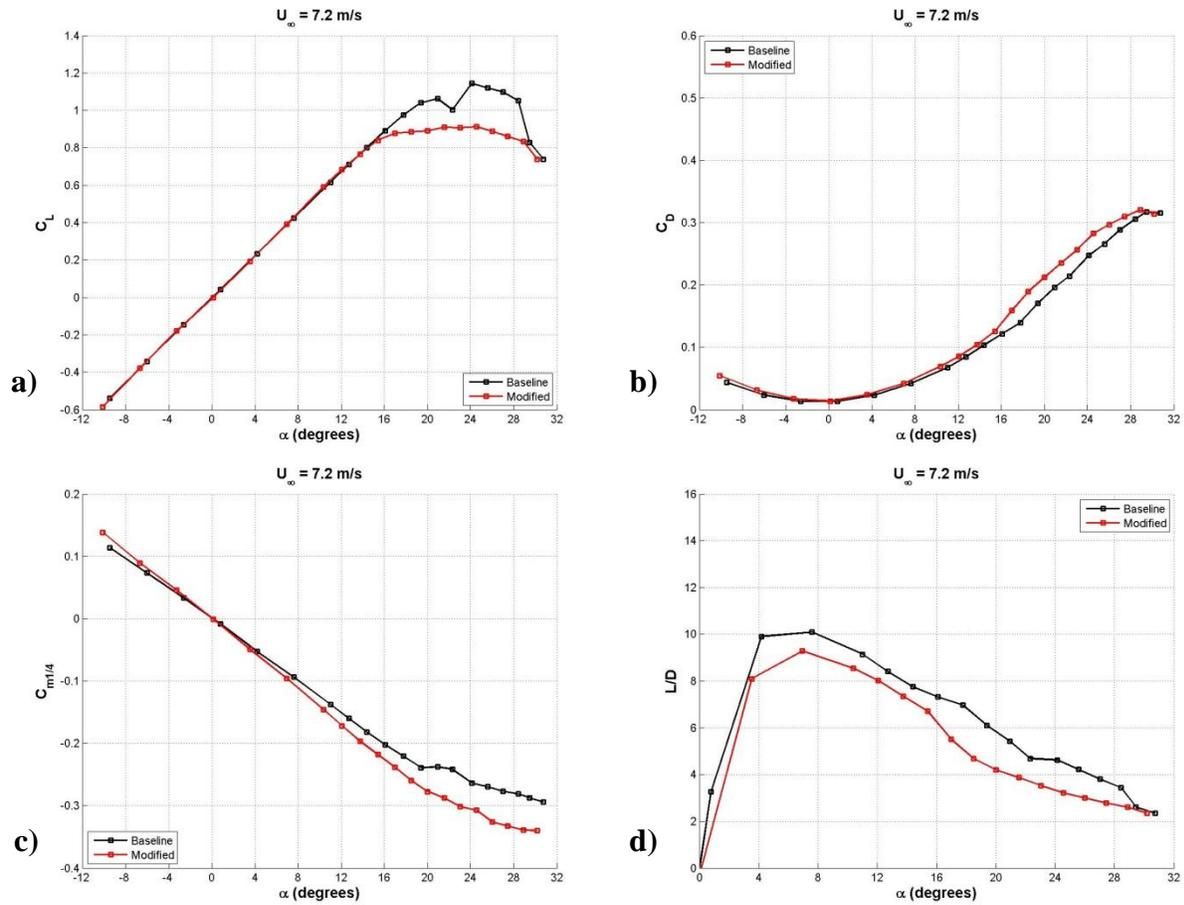
**Figure 99: Effect of protuberances on the load characteristics of cavitating swept hydrofoils; a) lift coefficient, b) drag coefficient, c) quarter chord moment coefficient, d) lift-to-drag ratio.**
