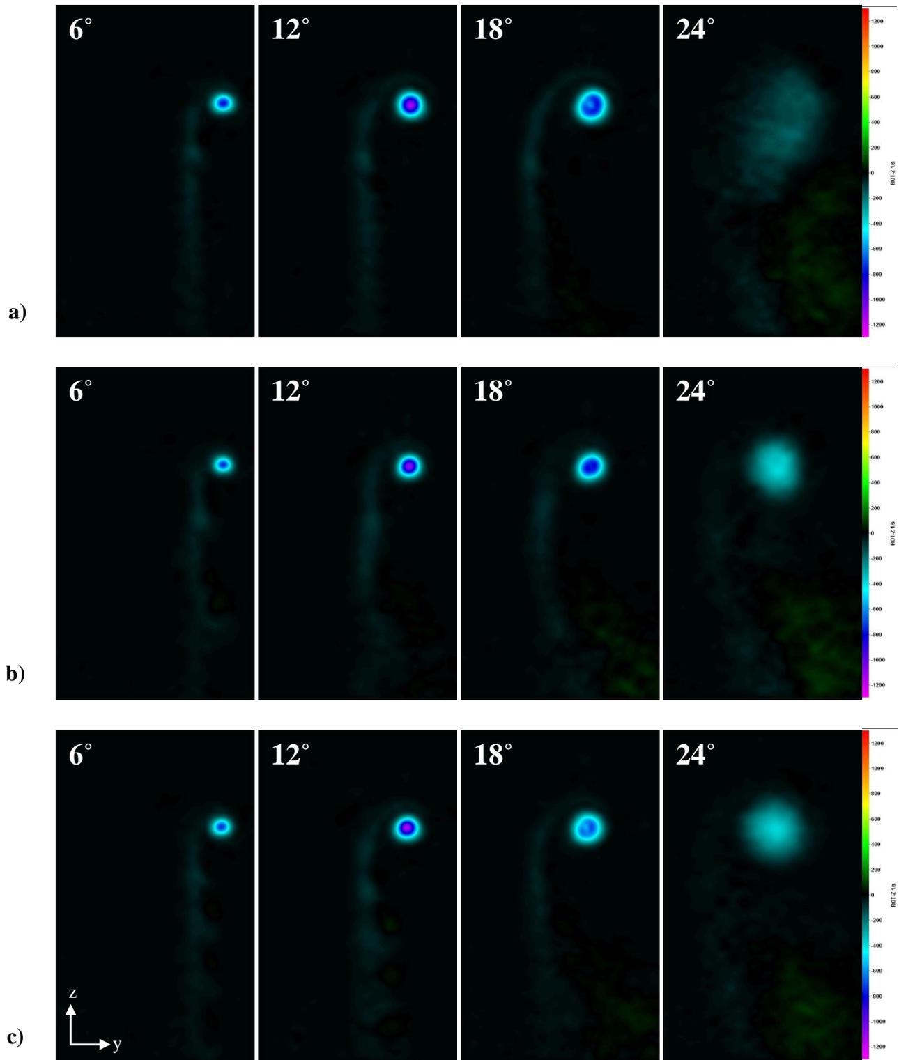
**Figure 78: Streamwise vorticity contours of the tip vortex on finite-span rectangular hydrofoils 1.50c downstream of baseline hydrofoil leading edge.  $U_{\infty} = 1.8$  m/s. a) Baseline b) 4L c) 8M.**
