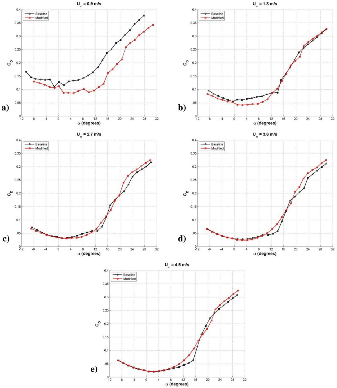
**Figure 58: Flipper model drag coefficient. a)  $Re_c = 9.0 \times 10^4$ , b)  $Re_c = 1.8 \times 10^5$ , c)  $Re_c = 2.7 \times 10^5$ , d)  $Re_c = 3.6 \times 10^5$ , e)  $Re_c = 4.5 \times 10^5$ .**
