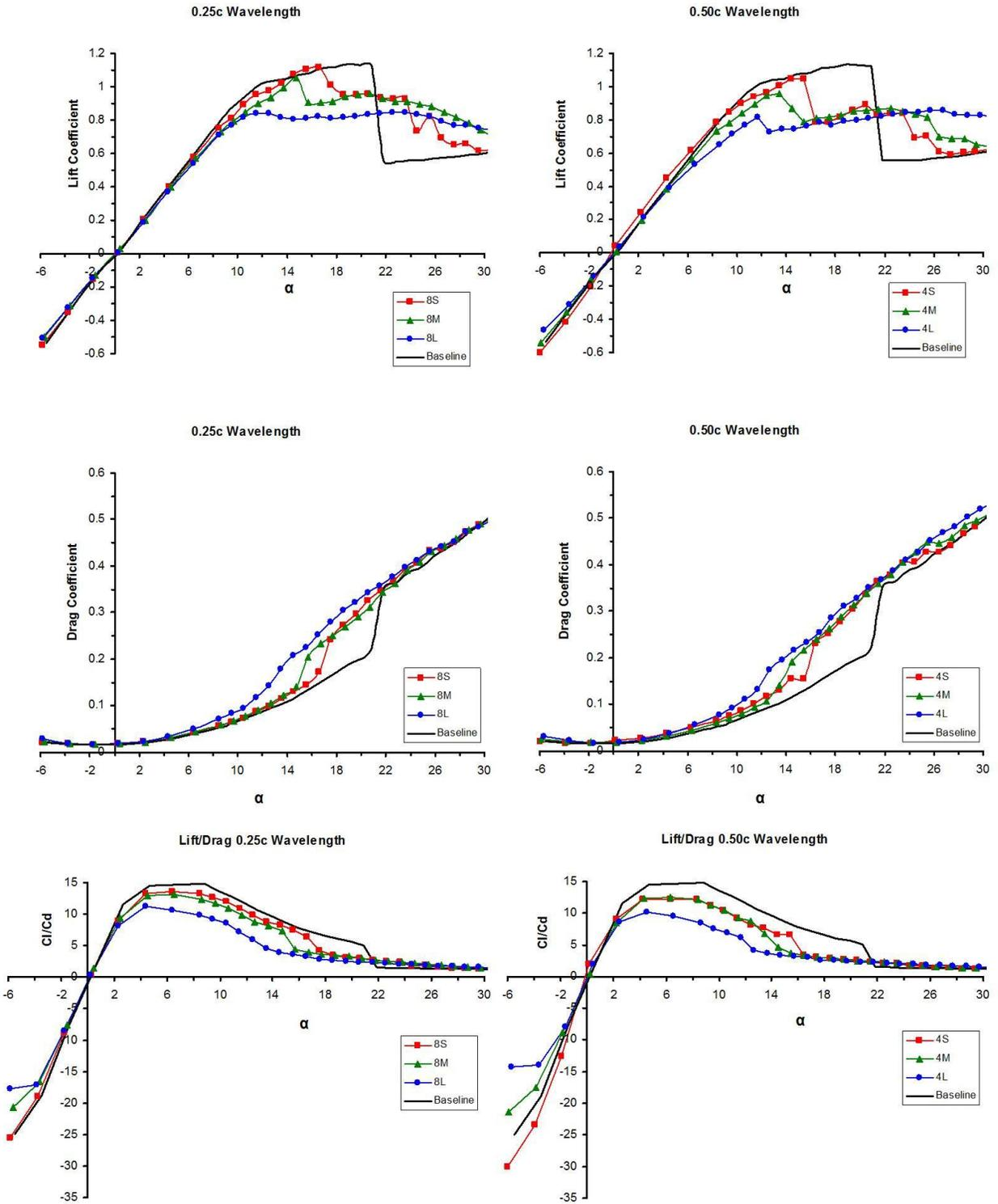
Figure 4: Lift and drag performance of hydrofoils tested by Johari et al.<sup>7</sup>
