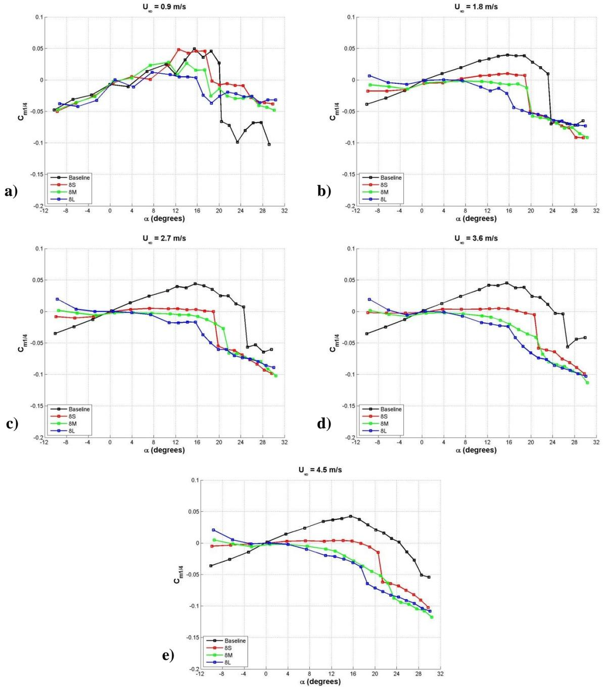
**Figure 35: Effect of protuberance amplitude on the quarter chord moment coefficient of finite-span rectangular planform hydrofoils,  $\lambda = 0.25c$ . a)  $Re_c = 9.0 \times 10^4$ , b)  $Re_c = 1.8 \times 10^5$ , c)  $Re_c = 2.7 \times 10^5$ , d)  $Re_c = 3.6 \times 10^5$ , e)  $Re_c = 4.5 \times 10^5$ .**
