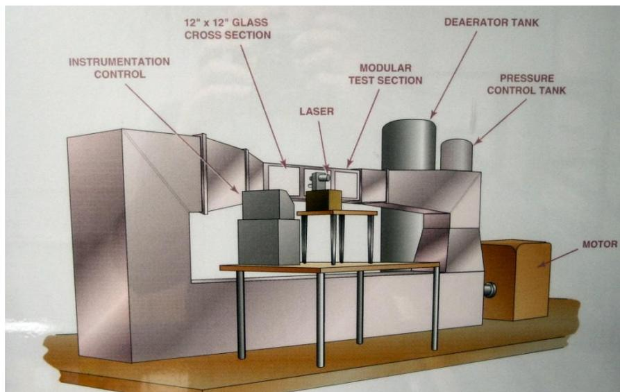
**Figure 5: Schematic of the NUWC water Tunnel**
