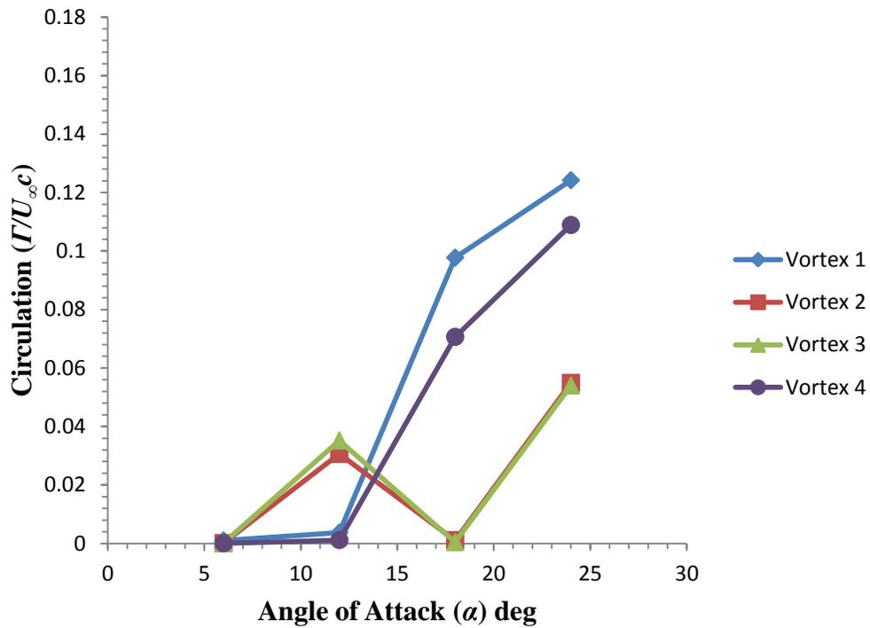
Figure 72:  $\Gamma$  as a function of  $\alpha$  at a chordwise spatial location of  $x/c = 0.36c$ .  $U_\infty = 4.5$  m/s.
