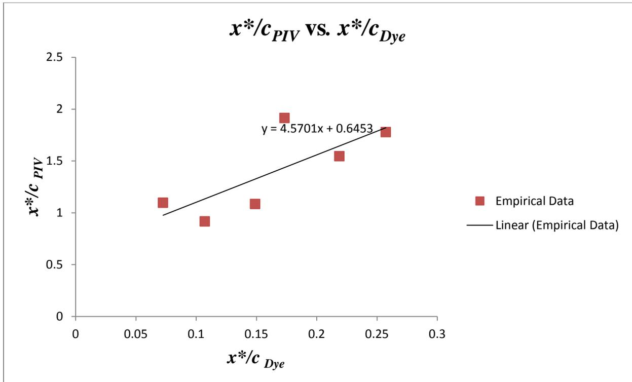
Figure 105: Comparison of the observed vortex interaction point seen in dye images to the calculated interaction point,  $\frac{x_{PIV}^*}{c}$ , using Equation (6).
