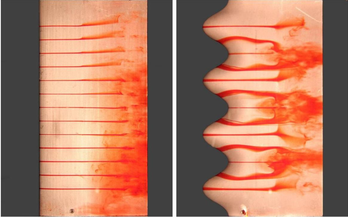
**Figure 82: Dye flow visualization  $\alpha = 0^\circ$ .**
