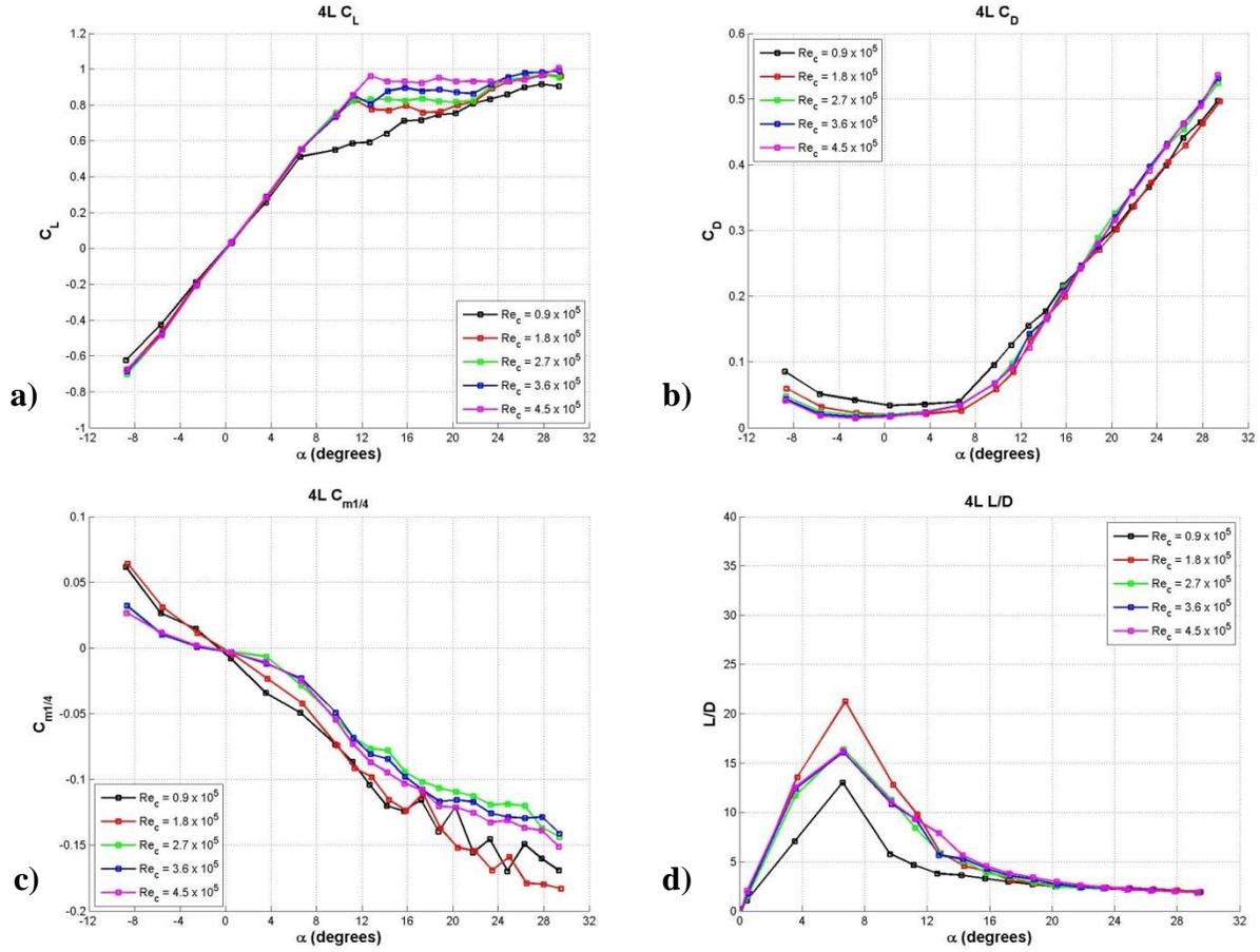
Figure 19: Infinite-span 4L hydrofoil load characteristics at multiple Reynolds numbers. a) lift coefficient, b) drag coefficient, c) quarter chord moment coefficient, d) L/D ratio.
