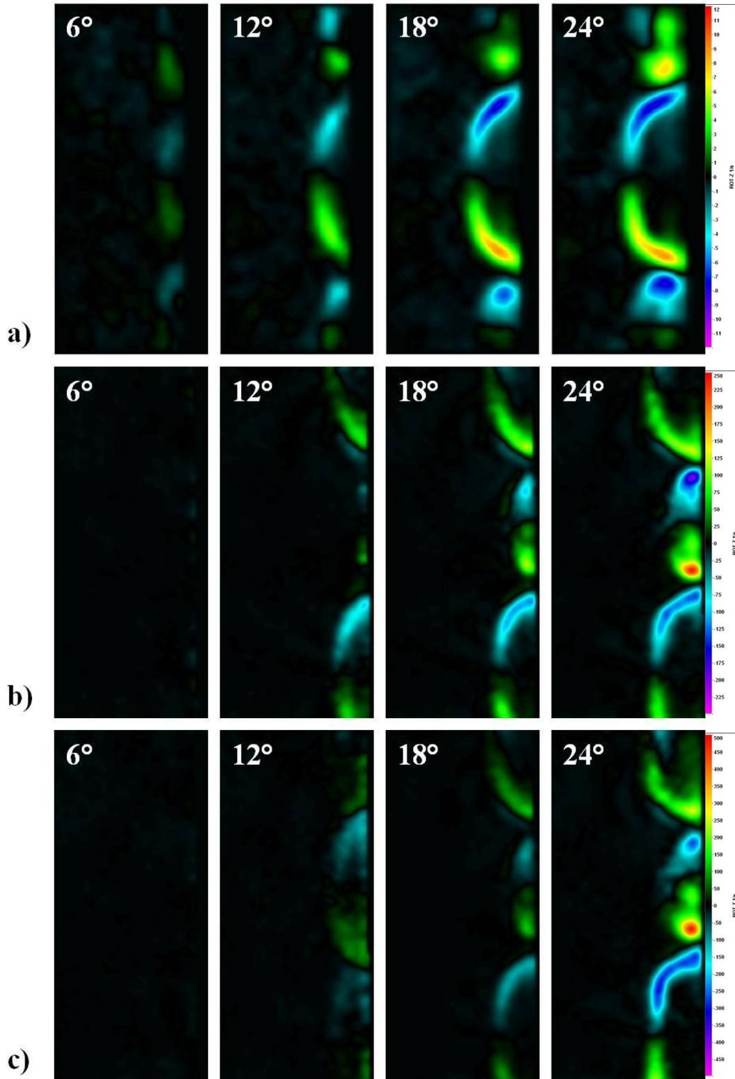
Figure 65: Streamwise vorticity,  $\omega$ , contours on 4L hydrofoil as a function of angle of attack at a chordwise spatial location of  $0.36c$ . a)  $U_\infty = 0.15$  m/s, b)  $U_\infty = 1.80$  m/s, c)  $U_\infty = 4.50$  m/s.
