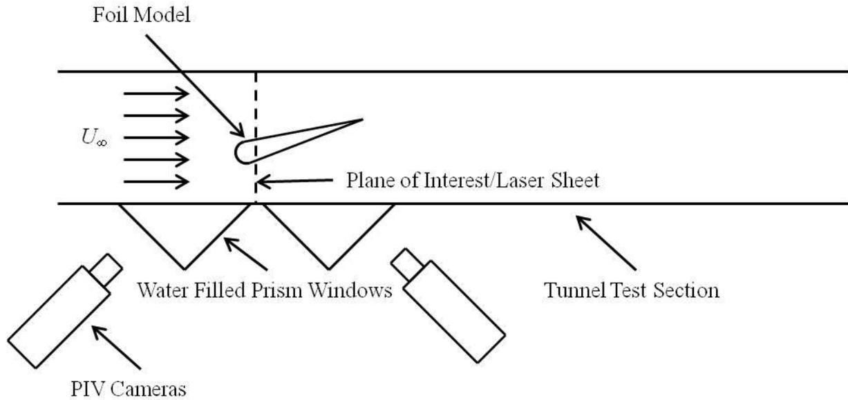
**Figure 15: Schematic of full-span high-speed SPIV system and water tunnel.**
