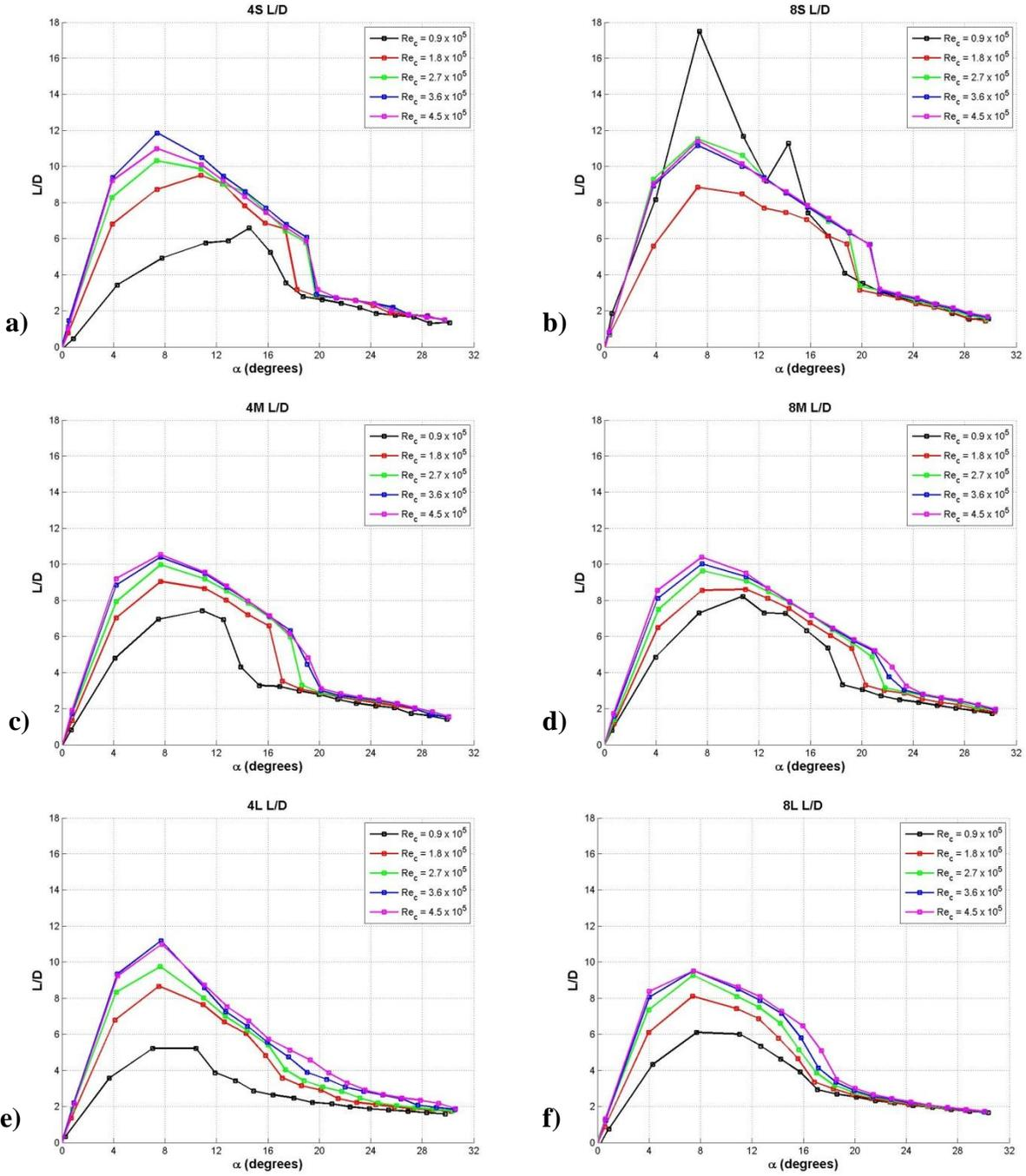
**Figure 28: Effect of Reynolds number on the lift-to-drag ratio of finite-span rectangular planform modified hydrofoils. a) 4S, b) 8S, c) 4M, d) 8M, e) 4L, f) 8L.**
