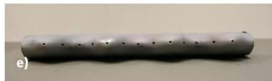
**Figure 12: a) Dye injection system; b) dye valve connected to baseline foil; c) dye valve connected to 4L foil; d) leading edge of baseline foil with dye ports; e) leading edge of 4L foil with dye ports.**
