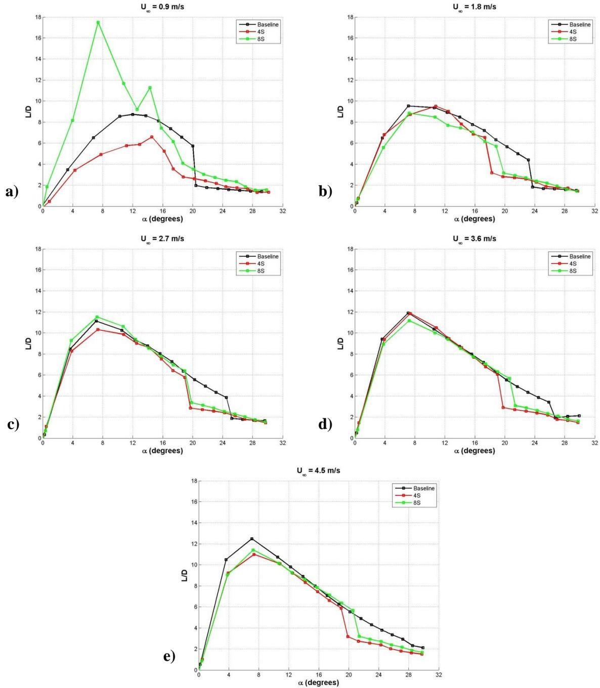
Figure 40: Effect of protuberance wavelength on the lift-to-drag ratio of finite-span rectangular planform hydrofoils,  $A = 0.025c$ . a)  $Re_c = 9.0 \times 10^4$ , b)  $Re_c = 1.8 \times 10^5$ , c)  $Re_c = 2.7 \times 10^5$ , d)  $Re_c = 3.6 \times 10^5$ , e)  $Re_c = 4.5 \times 10^5$ .
