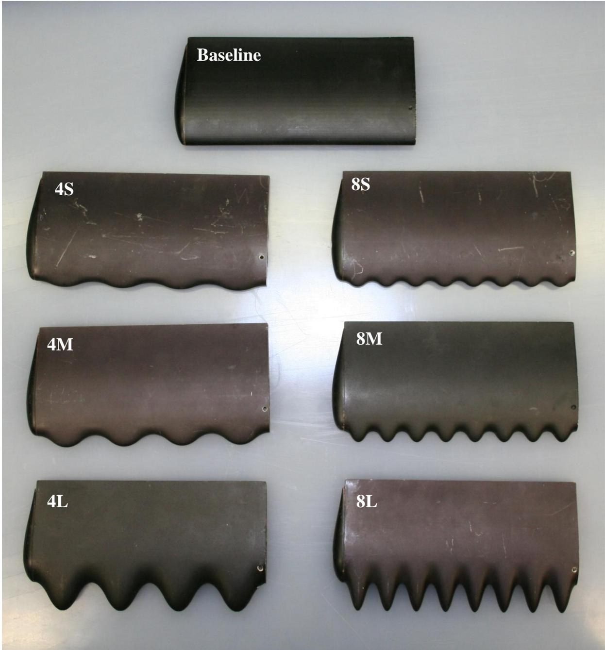
**Figure 8: Hydrofoils of 219 mm span with endcaps attached.**
