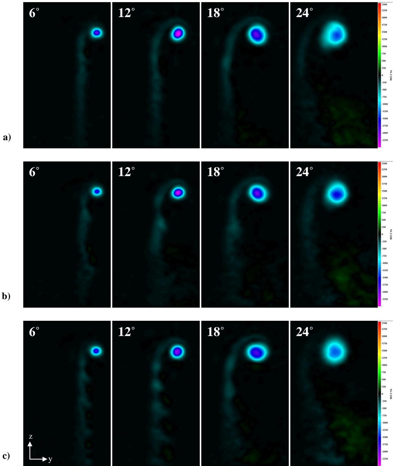
**Figure 80: Streamwise vorticity contours of the tip vortex on finite-span rectangular hydrofoils 1.50c downstream of baseline hydrofoil leading edge.  $U_\infty = 4.5$  m/s. a) Baseline b) 4L c) 8M.**
