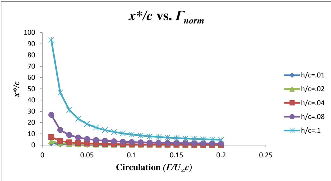
**Figure 103: Effect of  $\Gamma$  on  $\frac{x^*}{c}$**
