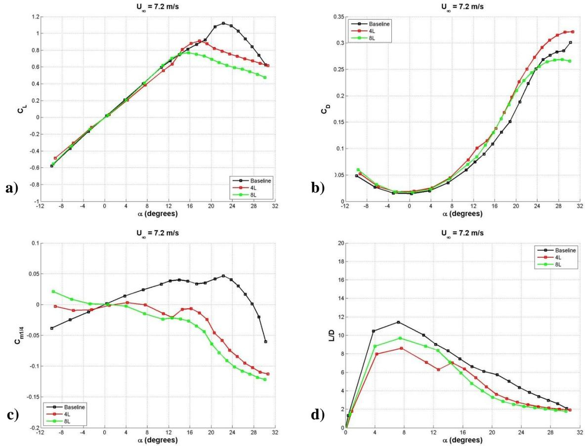
Figure 98: Effect of protuberance wavelength on the load characteristics of cavitating hydrofoils with a protuberance amplitude of  $A = 0.12c$ ; a) lift coefficient, b) drag coefficient, c) quarter chord moment coefficient, d) lift-to-drag ratio.
