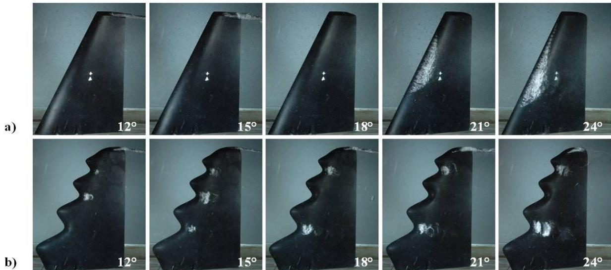
**Figure 93: Vaporous cavitation on the leading edge and tip vortex of finite-span swept hydrofoils; a) baseline, b) modified.**
