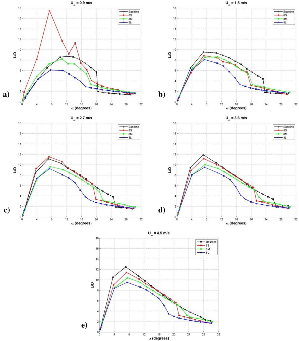
**Figure 36: Effect of protuberance amplitude on the lift-to-drag ratio of finite-span rectangular planform hydrofoils,  $\lambda = 0.25c$ . a)  $Re_c = 9.0 \times 10^4$ , b)  $Re_c = 1.8 \times 10^5$ , c)  $Re_c = 2.7 \times 10^5$ , d)  $Re_c = 3.6 \times 10^5$ , e)  $Re_c = 4.5 \times 10^5$ .**
