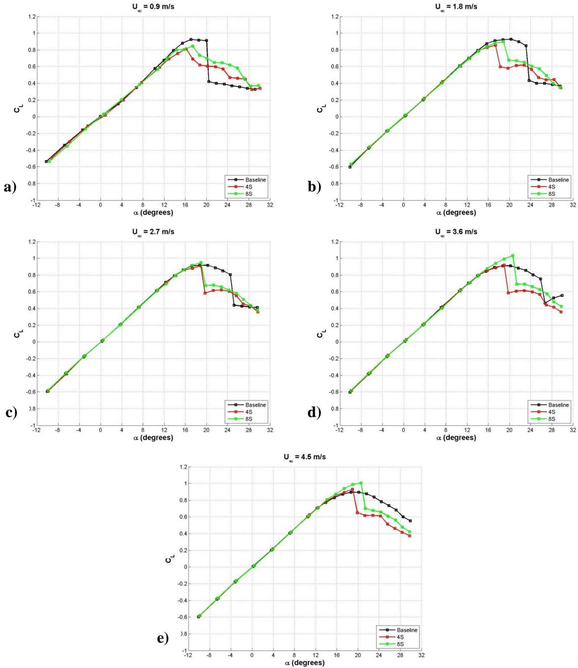
**Figure 37: Effect of protuberance wavelength on the lift coefficient of finite-span rectangular planform hydrofoils,  $A = 0.025c$ . a)  $Re_c = 9.0 \times 10^4$ , b)  $Re_c = 1.8 \times 10^5$ , c)  $Re_c = 2.7 \times 10^5$ , d)  $Re_c = 3.6 \times 10^5$ , e)  $Re_c = 4.5 \times 10^5$ .**
