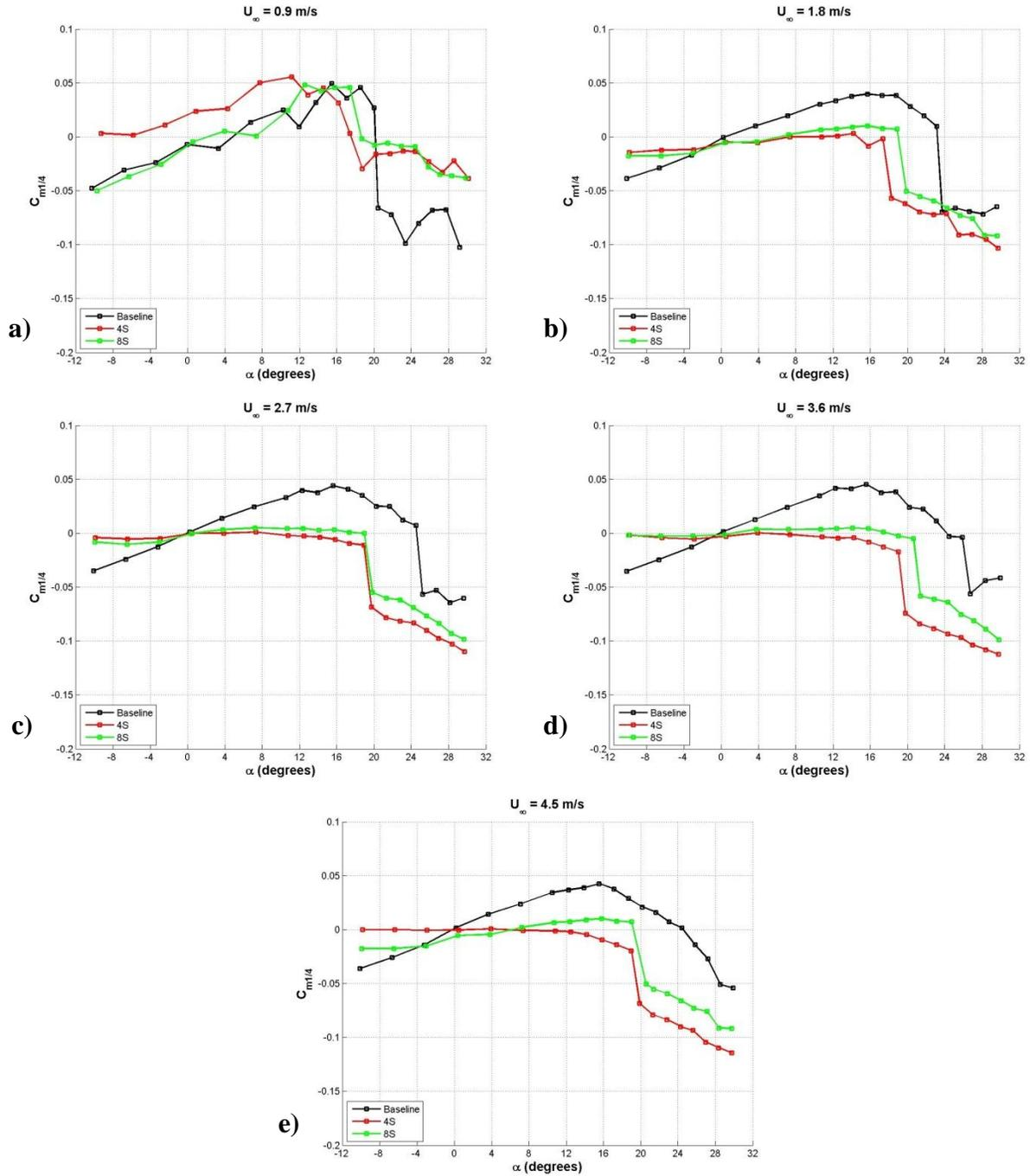
**Figure 39: Effect of protuberance wavelength on the quarter chord moment coefficient of finite-span rectangular planform hydrofoils,  $A = 0.025c$ . a)  $Re_c = 9.0 \times 10^4$ , b)  $Re_c = 1.8 \times 10^5$ , c)  $Re_c = 2.7 \times 10^5$ , d)  $Re_c = 3.6 \times 10^5$ , e)  $Re_c = 4.5 \times 10^5$ .**
