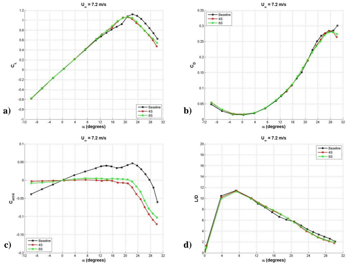
Figure 96: Effect of protuberance wavelength on the load characteristics of cavitating hydrofoils with a protuberance amplitude of  $A = 0.025c$ ; a) lift coefficient, b) drag coefficient, c) quarter chord moment coefficient, d) lift-to-drag ratio.
