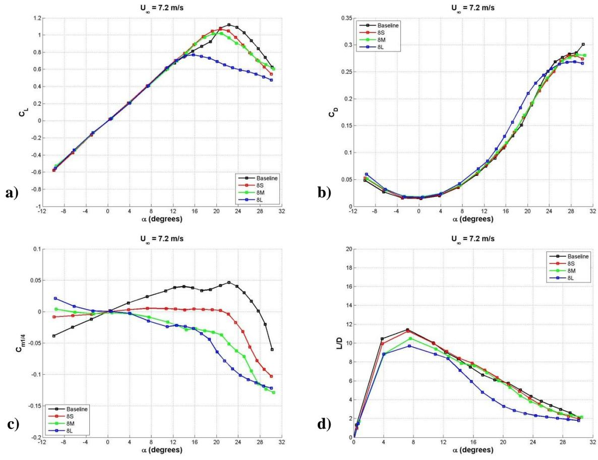
**Figure 95: Effect of protuberance amplitude on the load characteristics of cavitating hydrofoils with a protuberance wavelength of  $\lambda = 0.25c$ ; a) lift coefficient, b) drag coefficient, c) quarter chord moment coefficient, d) lift-to-drag ratio.**
