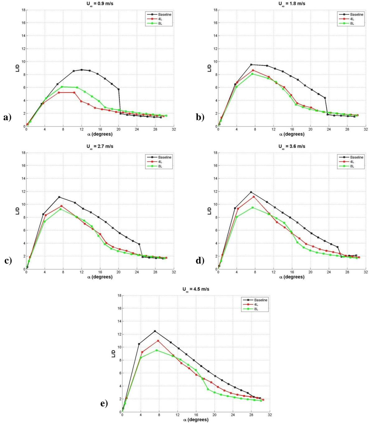
**Figure 48: Effect of protuberance wavelength on the lift-to-drag ratio of finite-span rectangular planform hydrofoils,  $A = 0.120c$ . a)  $Re_c = 9.0 \times 10^4$ , b)  $Re_c = 1.8 \times 10^5$ , c)  $Re_c = 2.7 \times 10^5$ , d)  $Re_c = 3.6 \times 10^5$ , e)  $Re_c = 4.5 \times 10^5$ .**
