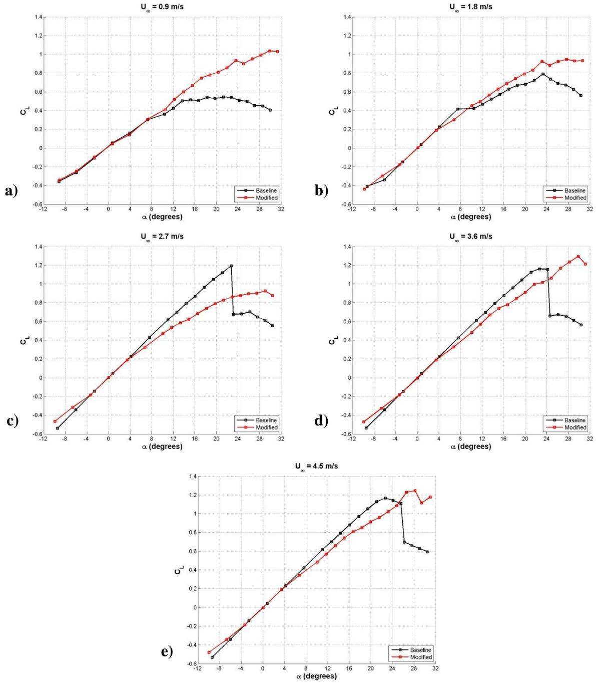
**Figure 51: Swept planform lift coefficient. a)  $Re_c = 9.0 \times 10^4$ , b)  $Re_c = 1.8 \times 10^5$ , c)  $Re_c = 2.7 \times 10^5$ , d)  $Re_c = 3.6 \times 10^5$ , e)  $Re_c = 4.5 \times 10^5$ .**
