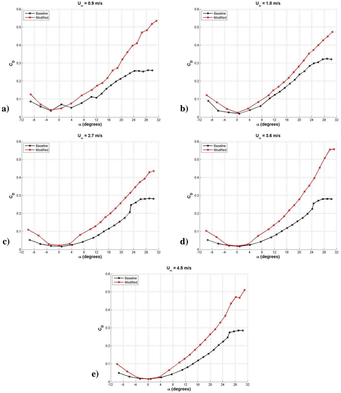
**Figure 52: Swept planform drag coefficient. a)  $Re_c = 9.0 \times 10^4$ , b)  $Re_c = 1.8 \times 10^5$ , c)  $Re_c = 2.7 \times 10^5$ , d)  $Re_c = 3.6 \times 10^5$ , e)  $Re_c = 4.5 \times 10^5$ .**
