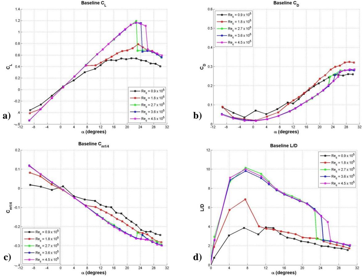
**Figure 49: Effect of Reynolds number on the swept planform baseline hydrofoil load characteristics. a) lift coefficient, b) drag coefficient, c) quarter chord moment coefficient, d) L/D ratio.**
