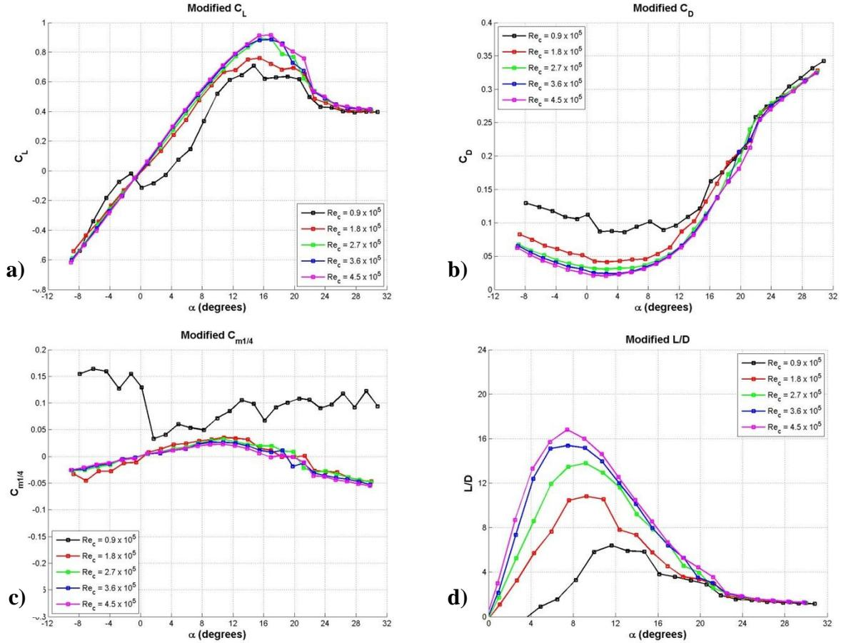
**Figure 56: Effect of Reynolds number on the flipper model modified hydrofoil load characteristics. a) lift coefficient, b) drag coefficient, c) quarter chord moment coefficient, d) L/D ratio.**
