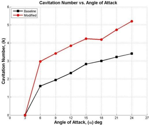
**Figure 101: Incipient cavitation number as a function of angle of attack of the modified swept foil.**
