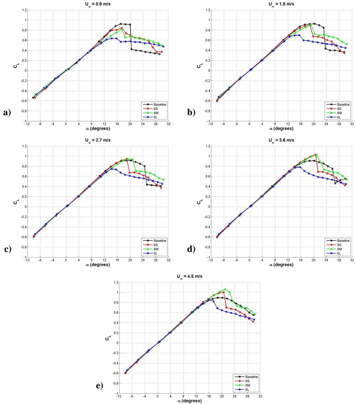
**Figure 33: Effect of protuberance amplitude on the lift coefficient of finite-span rectangular planform hydrofoils,  $\lambda = 0.25c$ . a)  $Re_c = 9.0 \times 10^4$ , b)  $Re_c = 1.8 \times 10^5$ , c)  $Re_c = 2.7 \times 10^5$ , d)  $Re_c = 3.6 \times 10^5$ , e)  $Re_c = 4.5 \times 10^5$ .**
