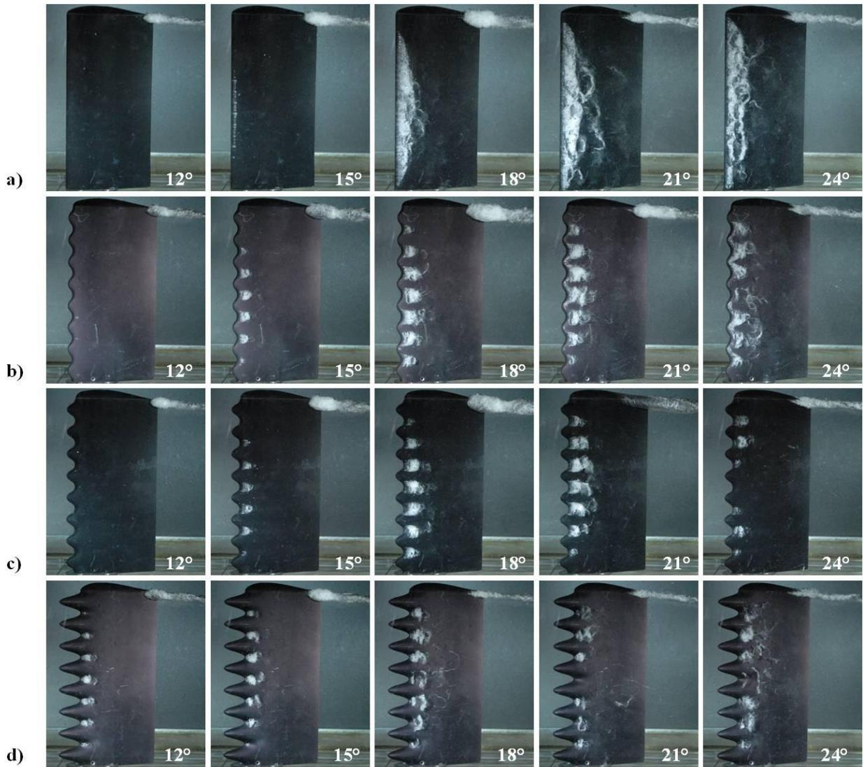
**Figure 92: Vaporous cavitation on the leading edge and tip vortex of finite-span rectangular hydrofoils; a) baseline, b) 8S, c) 8M, and d) 8L.**
