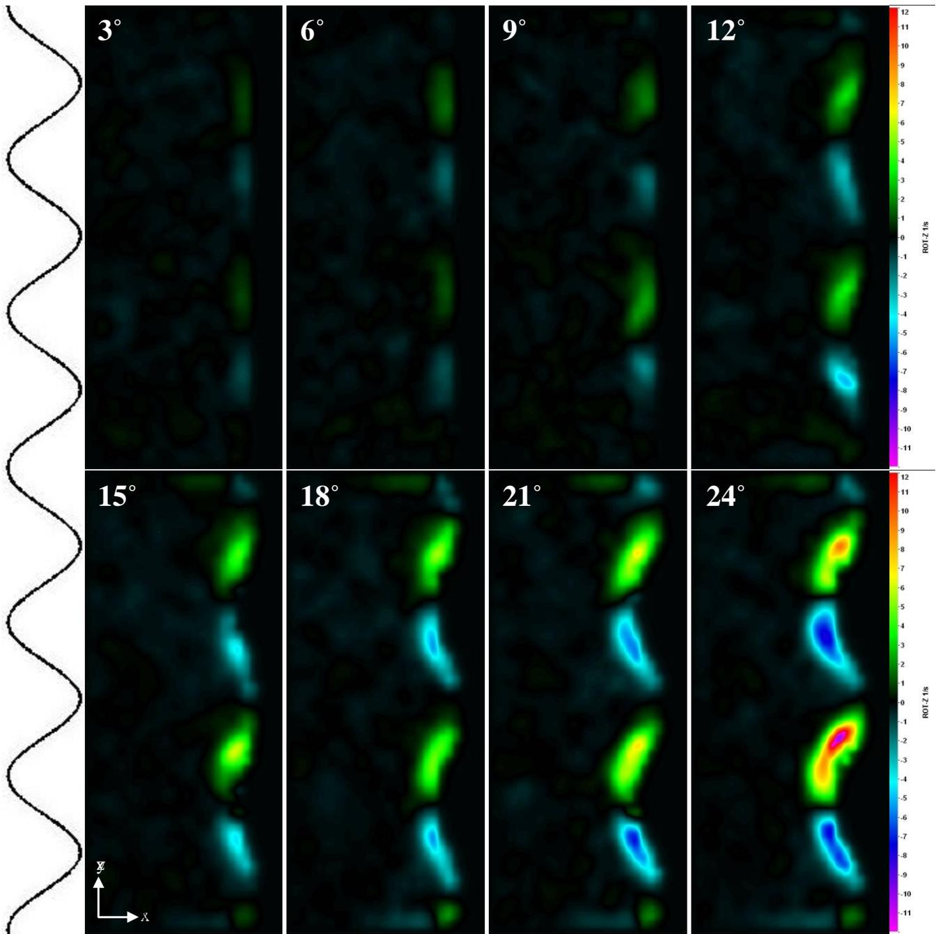
Figure 62: Streamwise vorticity,  $\omega$ , contours on 4L hydrofoil as a function of angle of attack at a chordwise spatial location of  $0.12c$ .
