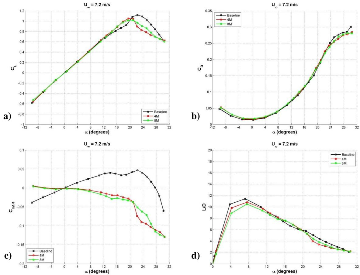
**Figure 97: Effect of protuberance wavelength on the load characteristics of cavitating hydrofoils with a protuberance amplitude of  $A = 0.050c$ ; a) lift coefficient, b) drag coefficient, c) quarter chord moment coefficient, d) lift-to-drag ratio.**
