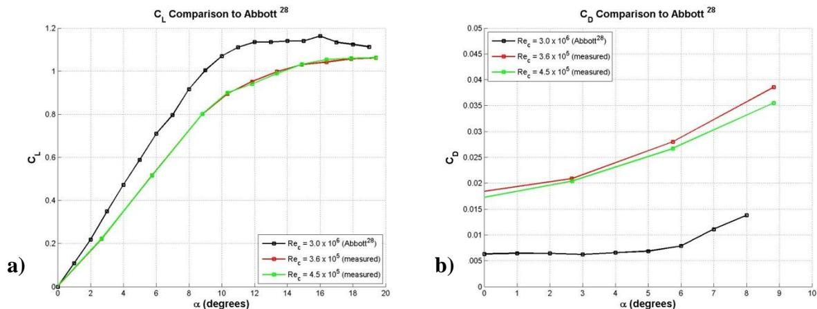
**Figure 18: Comparison of measured full-span data at the highest Reynolds numbers tested to Abbott and Von Doenhoff<sup>28</sup> data for identical cross-sectional profile.**
