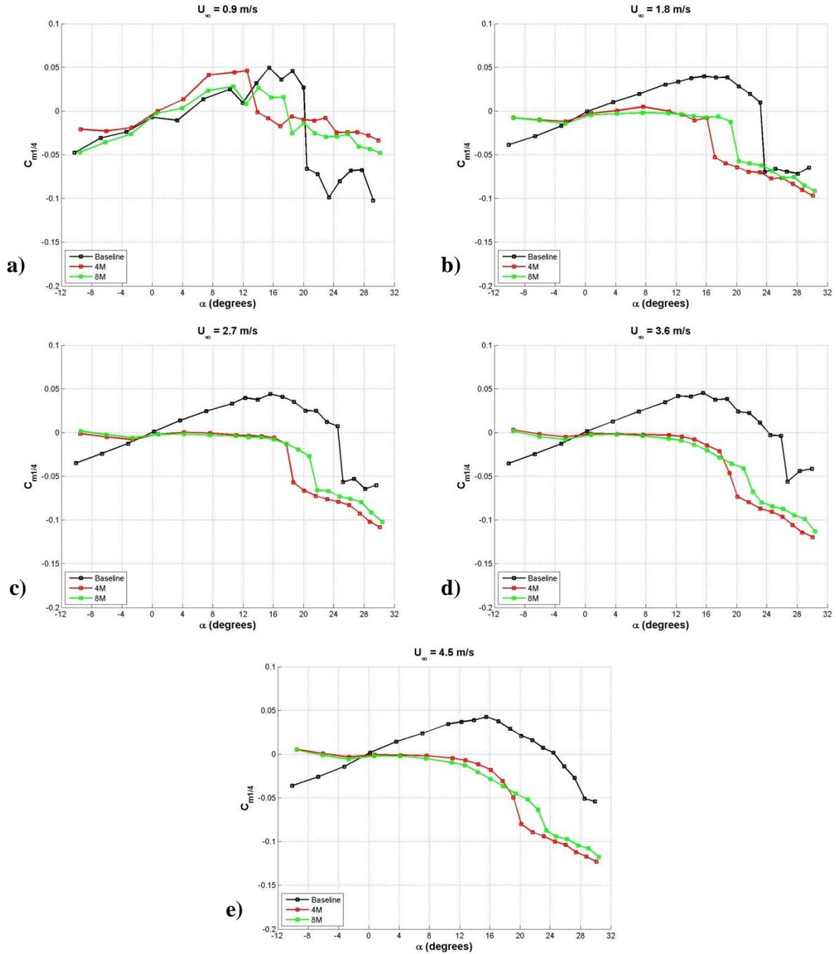
**Figure 43: Effect of protuberance wavelength on the quarter chord moment coefficient of finite-span rectangular planform hydrofoils,  $A = 0.050c$ . a)  $Re_c = 9.0 \times 10^4$ , b)  $Re_c = 1.8 \times 10^5$ , c)  $Re_c = 2.7 \times 10^5$ , d)  $Re_c = 3.6 \times 10^5$ , e)  $Re_c = 4.5 \times 10^5$ .**
