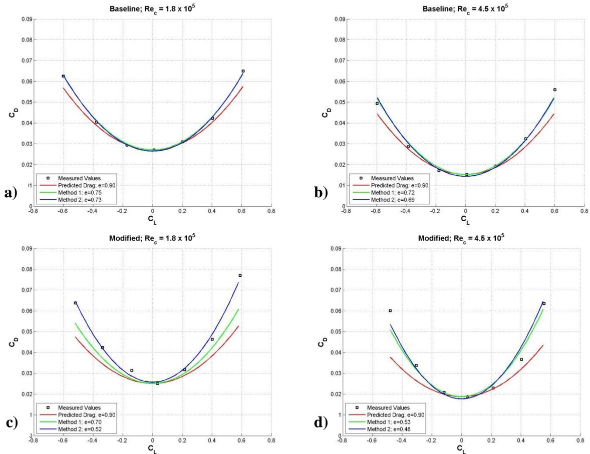
**Figure 106: Drag coefficient predictions using calculated span efficiency factors. a) Baseline foil at low  $Re_c$  b) Baseline foil at high  $Re_c$  c) 4L foil at low  $Re_c$  d) 4L foil at high  $Re_c$ .**
