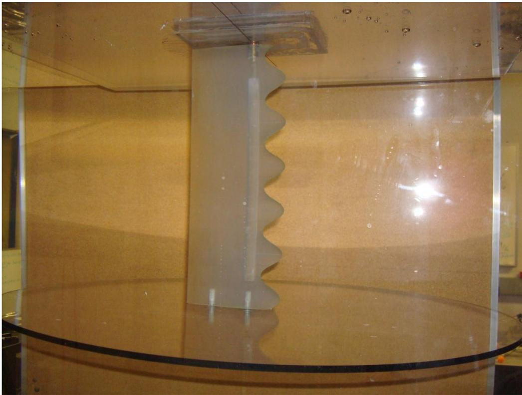
**Figure 13: Low-speed PIV experimental setup.**
