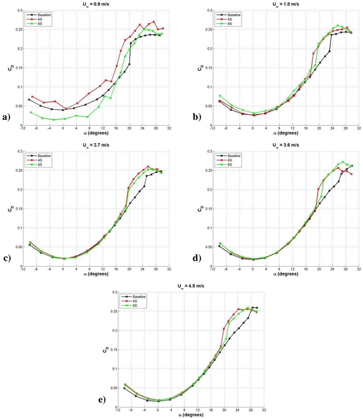
**Figure 38: Effect of protuberance wavelength on the drag coefficient of finite-span rectangular planform hydrofoils,  $A = 0.025c$ . a)  $Re_c = 9.0 \times 10^4$ , b)  $Re_c = 1.8 \times 10^5$ , c)  $Re_c = 2.7 \times 10^5$ , d)  $Re_c = 3.6 \times 10^5$ , e)  $Re_c = 4.5 \times 10^5$ .**
