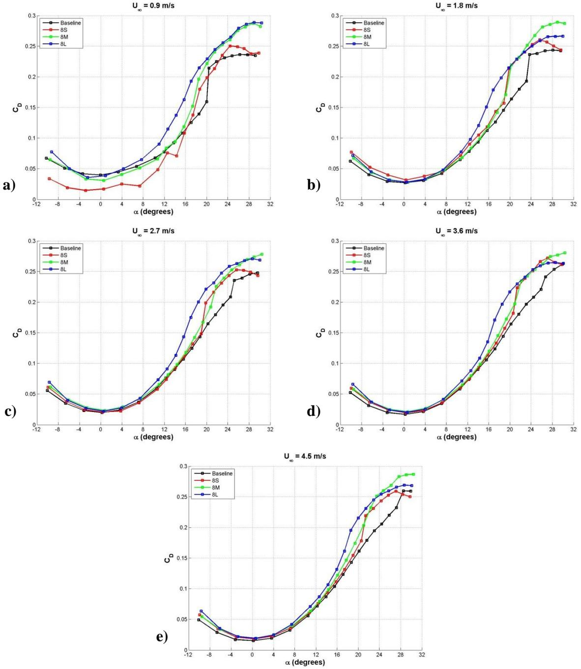
**Figure 34: Effect of protuberance amplitude on the drag coefficient of finite-span rectangular planform hydrofoils,  $\lambda = 0.25c$ . a)  $Re_c = 9.0 \times 10^4$ , b)  $Re_c = 1.8 \times 10^5$ , c)  $Re_c = 2.7 \times 10^5$ , d)  $Re_c = 3.6 \times 10^5$ , e)  $Re_c = 4.5 \times 10^5$ .**
