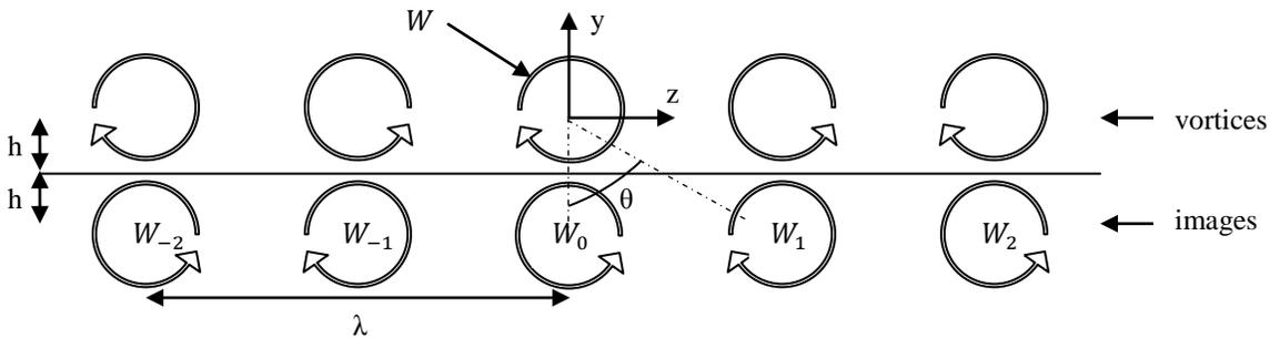
**Figure 102: Counter-rotating vortices with image pairs.**
