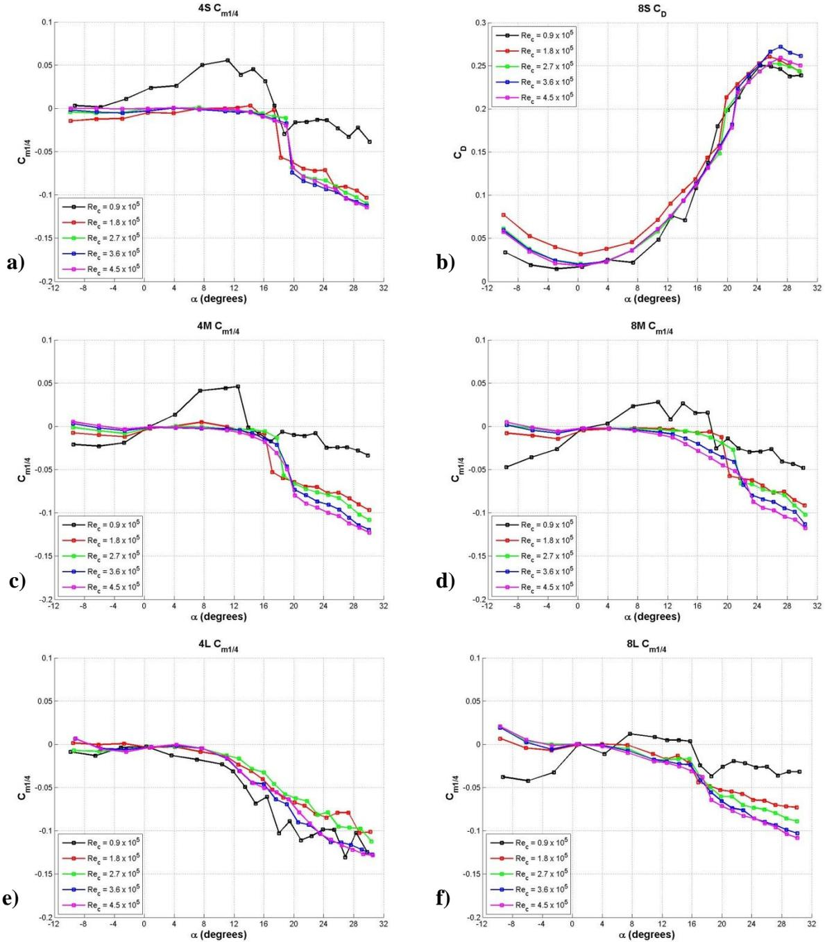
**Figure 27: Effect of Reynolds number on the quarter chord moment coefficient of finite-span rectangular planform modified hydrofoils. a) 4S, b) 8S, c) 4M, d) 8M, e) 4L, f) 8L.**
