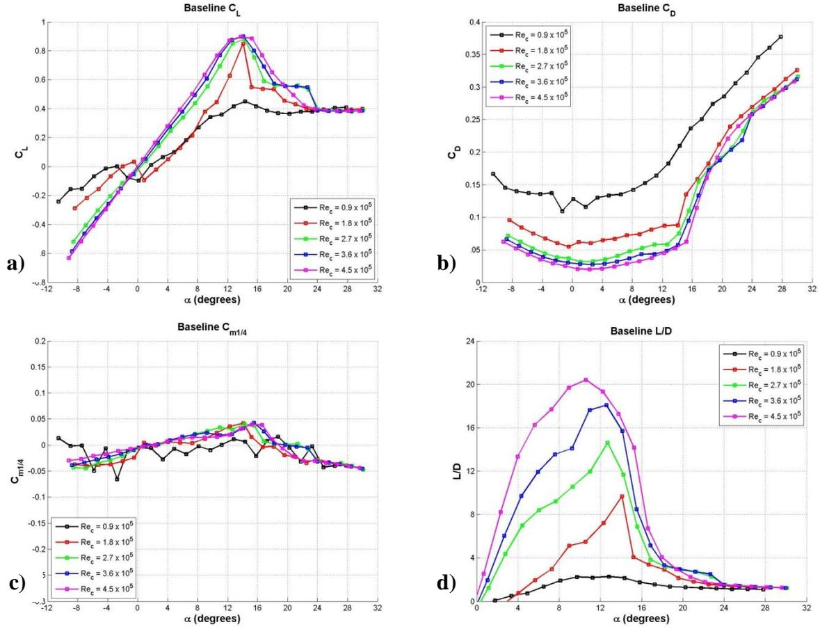
**Figure 55: Effect of Reynolds number on the flipper model baseline hydrofoil load characteristics. a) lift coefficient, b) drag coefficient, c) quarter chord moment coefficient, d) L/D ratio.**
