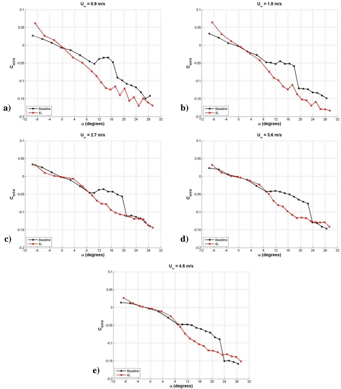
**Figure 22: Infinite-span planform quarter chord moment coefficient. a)  $Re_c = 9.0 \times 10^4$ , b)  $Re_c = 1.8 \times 10^5$ , c)  $Re_c = 2.7 \times 10^5$ , d)  $Re_c = 3.6 \times 10^5$ , e)  $Re_c = 4.5 \times 10^5$ .**
