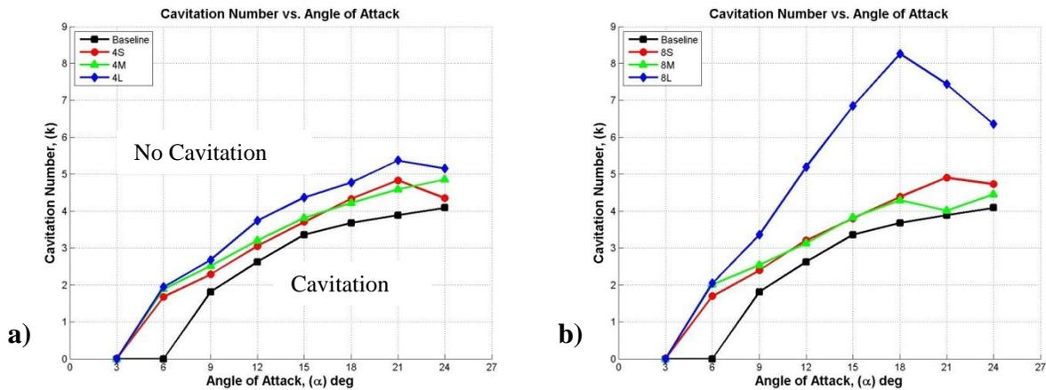
**Figure 100: Incipient cavitation number of finite-span rectangular modified foils as a function of angle of attack; a)  $\lambda = 0.50c$ , and b)  $\lambda = 0.25c$ .**
