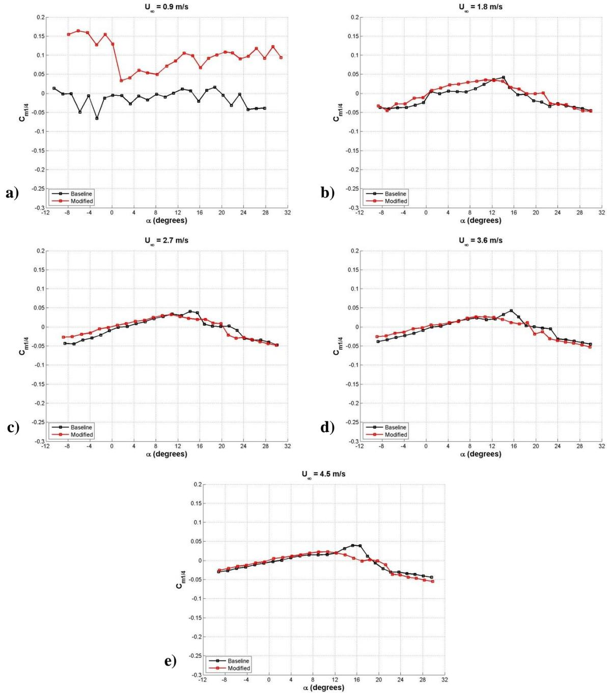
Figure 59: Flipper model quarter chord moment coefficient. a)  $Re_c = 9.0 \times 10^4$ , b)  $Re_c = 1.8 \times 10^5$ , c)  $Re_c = 2.7 \times 10^5$ , d)  $Re_c = 3.6 \times 10^5$ , e)  $Re_c = 4.5 \times 10^5$ .
