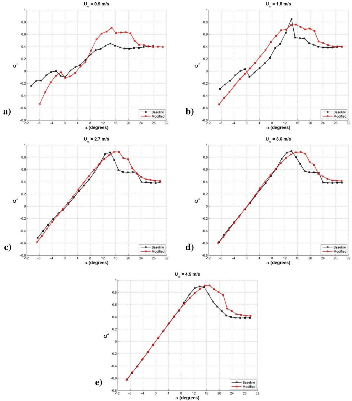
**Figure 57: Flipper model lift coefficient. a)  $Re_c = 9.0 \times 10^4$ , b)  $Re_c = 1.8 \times 10^5$ , c)  $Re_c = 2.7 \times 10^5$ , d)  $Re_c = 3.6 \times 10^5$ , e)  $Re_c = 4.5 \times 10^5$ .**
