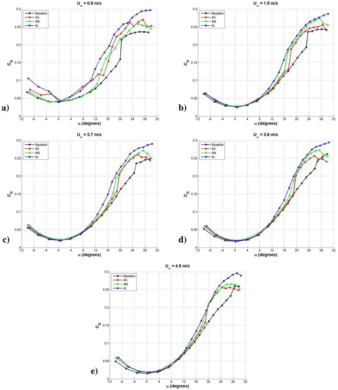
**Figure 30: Effect of protuberance amplitude on the drag coefficient of finite-span rectangular planform hydrofoils,  $\lambda = 0.50c$ . a)  $Re_c = 9.0 \times 10^4$ , b)  $Re_c = 1.8 \times 10^5$ , c)  $Re_c = 2.7 \times 10^5$ , d)  $Re_c = 3.6 \times 10^5$ , e)  $Re_c = 4.5 \times 10^5$ .**
