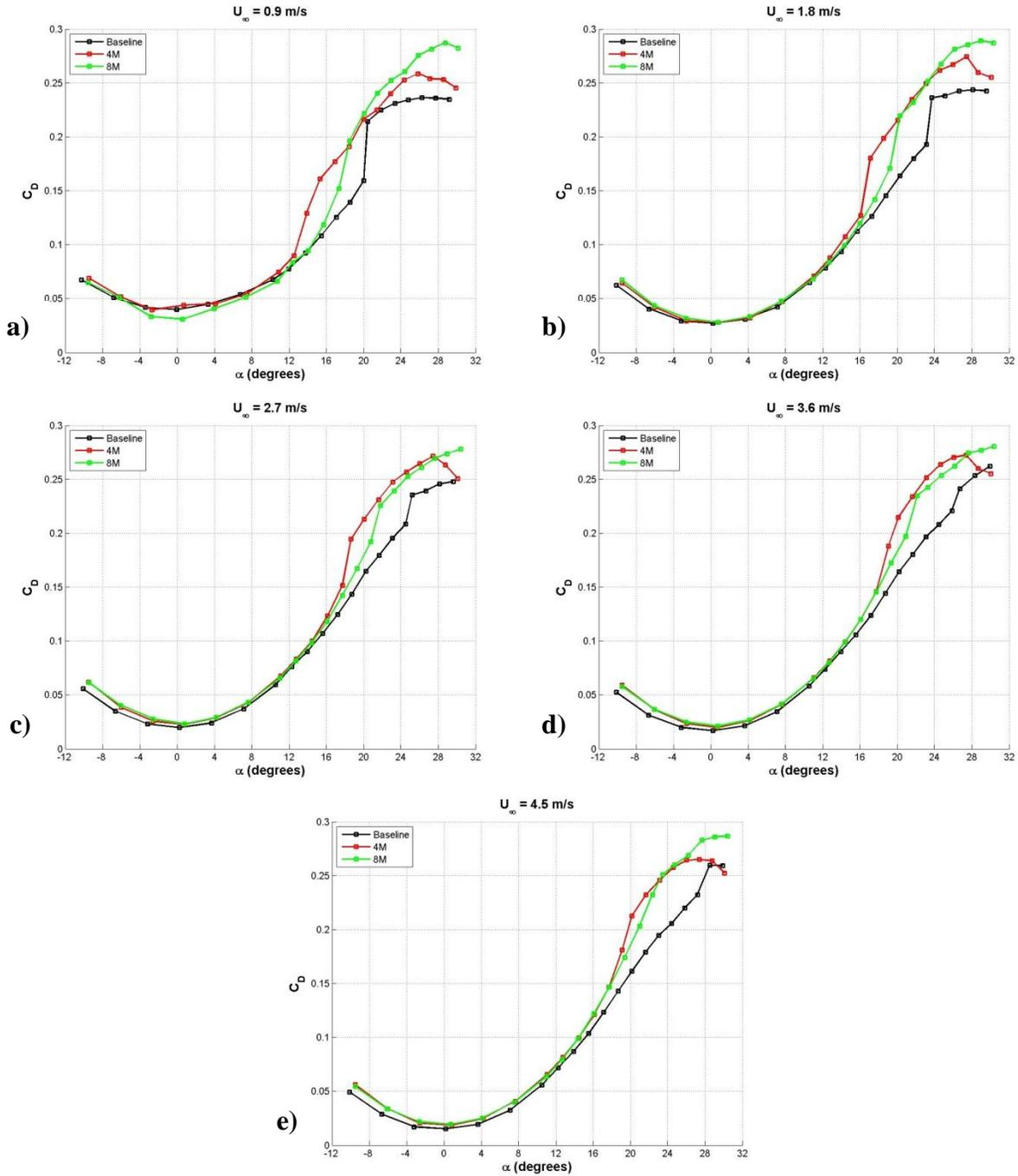
**Figure 42: Effect of protuberance wavelength on the drag coefficient of finite-span rectangular planform hydrofoils,  $A = 0.050c$ . a)  $Re_c = 9.0 \times 10^4$ , b)  $Re_c = 1.8 \times 10^5$ , c)  $Re_c = 2.7 \times 10^5$ , d)  $Re_c = 3.6 \times 10^5$ , e)  $Re_c = 4.5 \times 10^5$ .**
