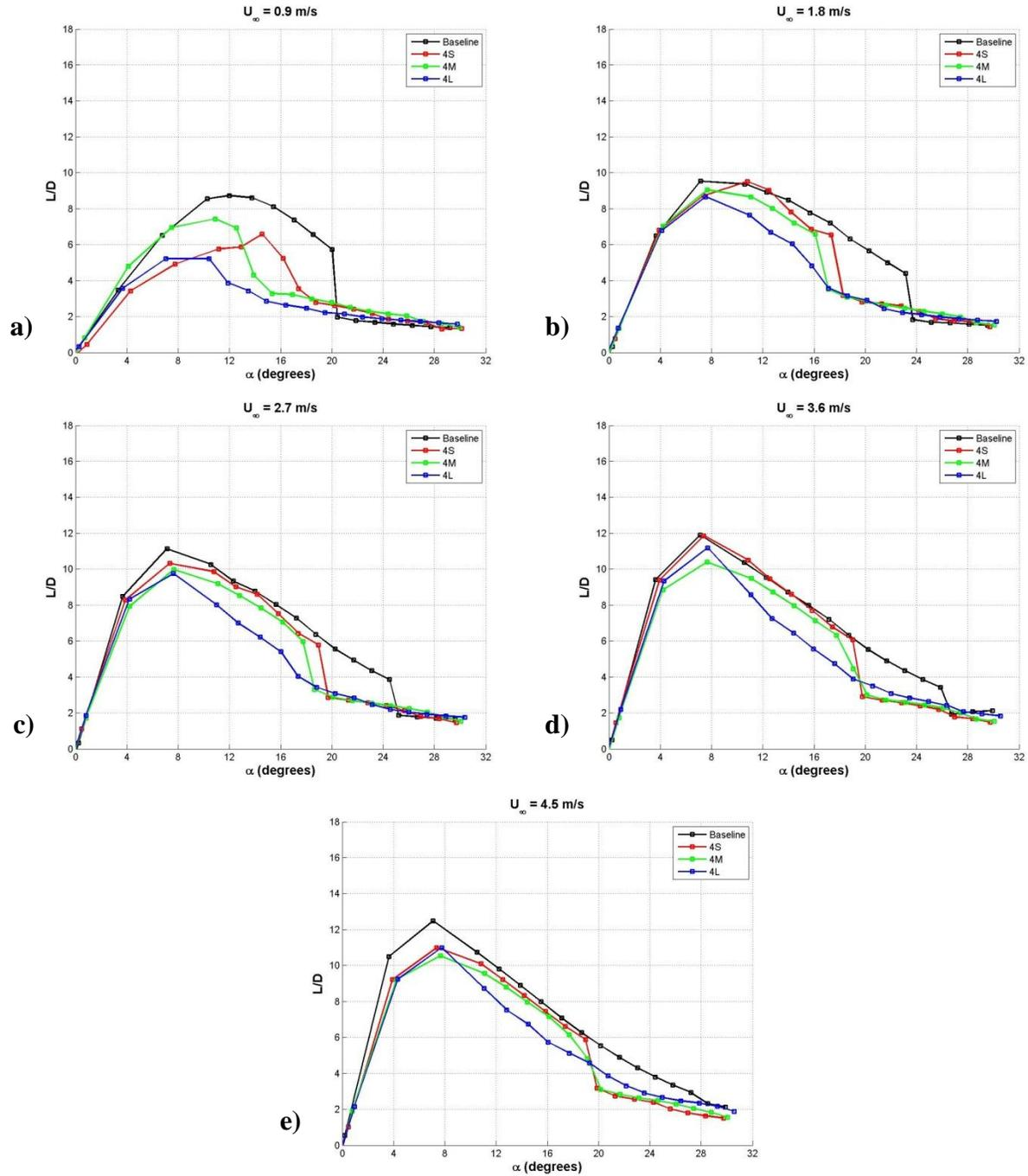
**Figure 32: Effect of protuberance amplitude on the lift-to-drag ratio of finite-span rectangular planform hydrofoils,  $\lambda = 0.50c$ . a)  $Re_c = 9.0 \times 10^4$ , b)  $Re_c = 1.8 \times 10^5$ , c)  $Re_c = 2.7 \times 10^5$ , d)  $Re_c = 3.6 \times 10^5$ , e)  $Re_c = 4.5 \times 10^5$ .**
