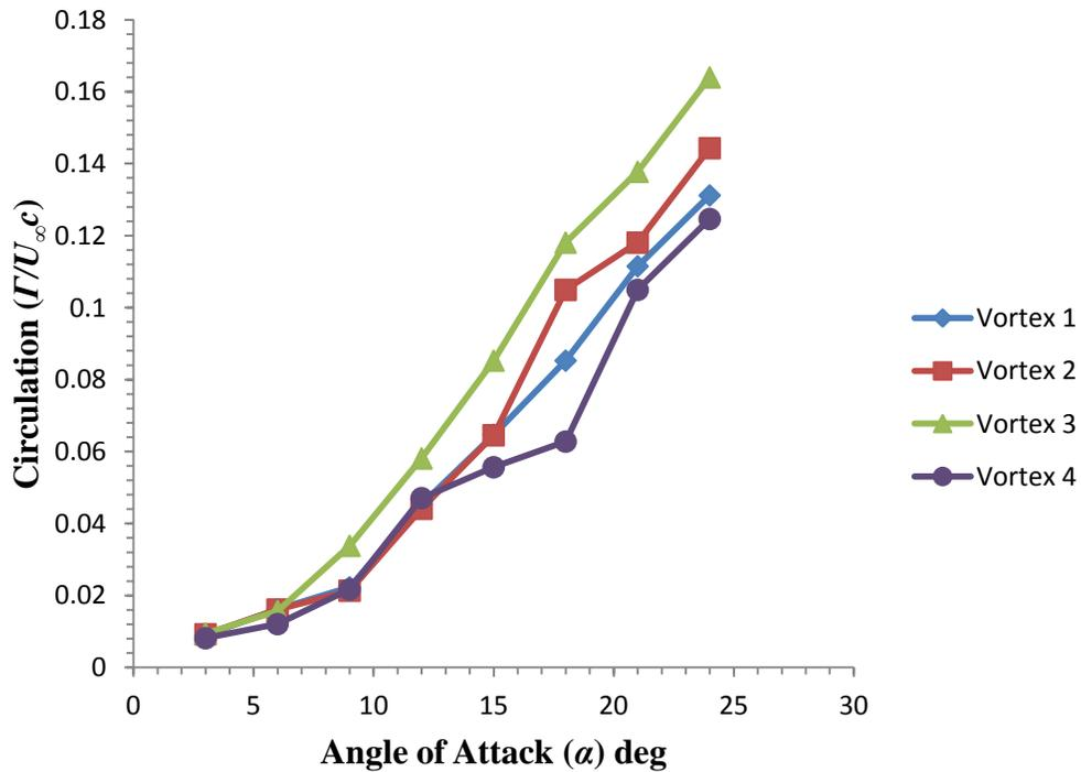
Figure 68:  $\Gamma$  as a function of  $\alpha$  at a chordwise spatial location of  $x/c = 0.12c$ .  $U_\infty = 0.15$  m/s.
