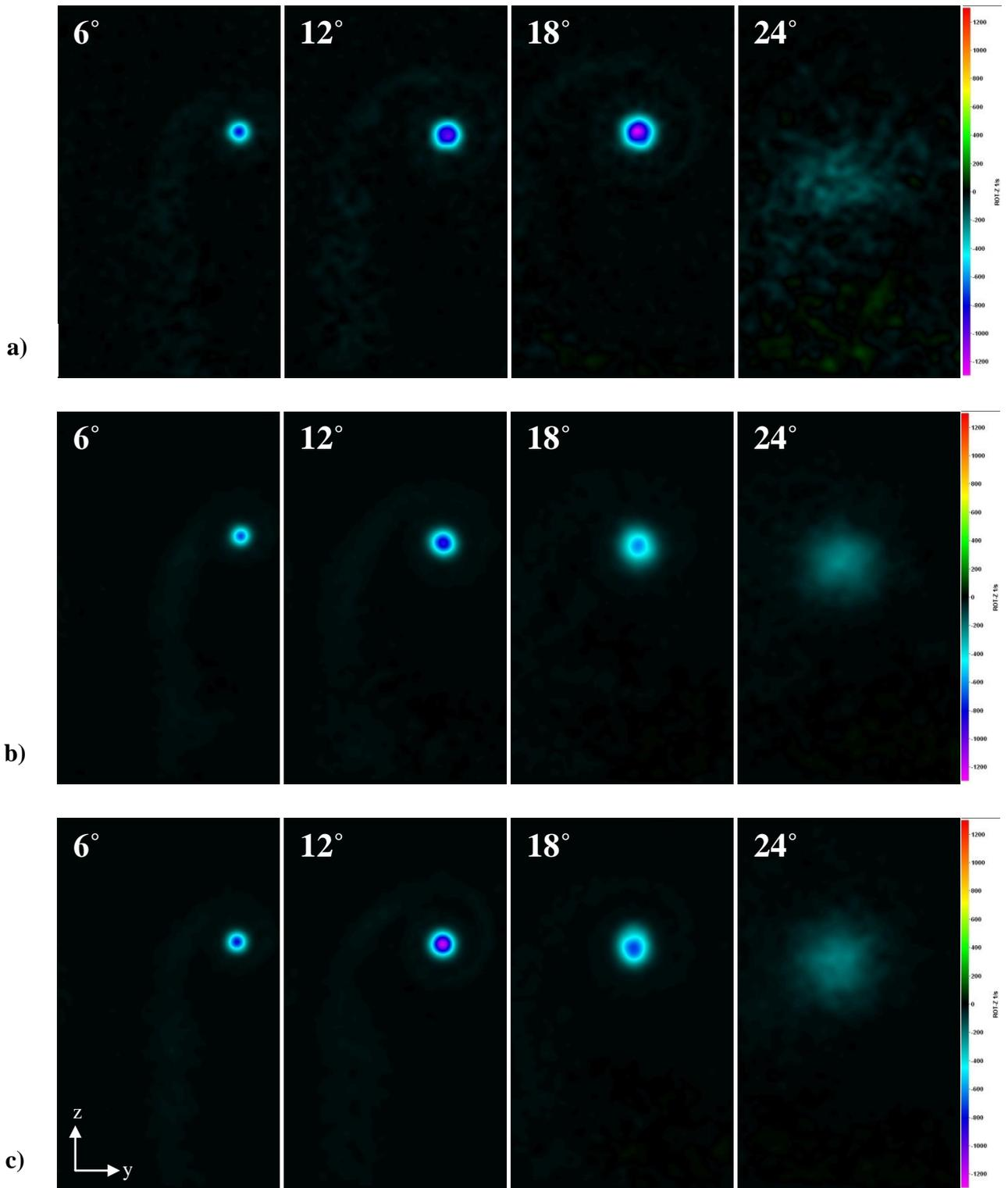
**Figure 79: Streamwise vorticity contours of the tip vortex on finite-span rectangular hydrofoils 3.00c downstream of baseline hydrofoil leading edge.  $U_\infty = 1.8$  m/s. a) Baseline b) 4L c) 8M.**
