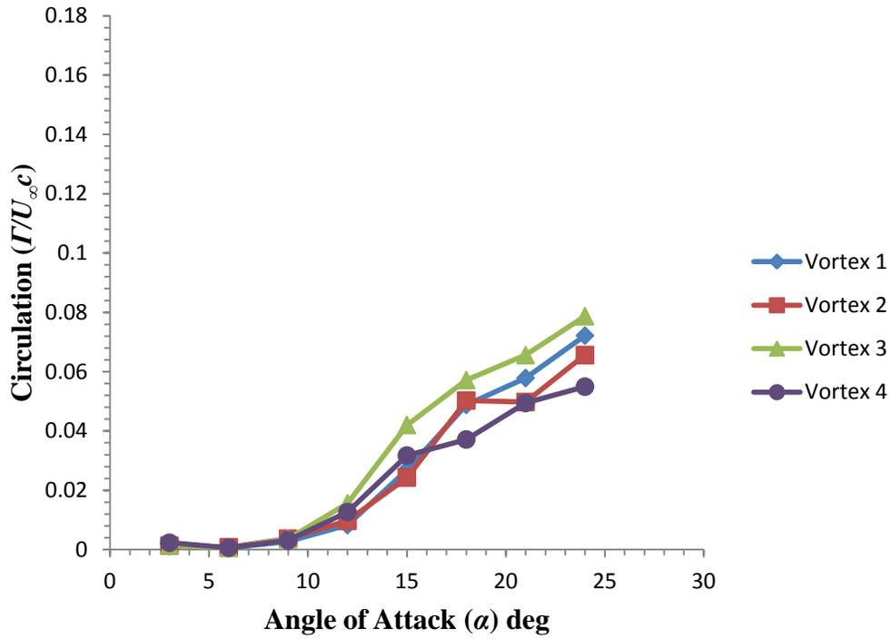
Figure 67:  $\Gamma$  as a function of  $\alpha$  at a chordwise spatial location of  $x/c = 0c$ .  $U_\infty = 0.15$  m/s.
