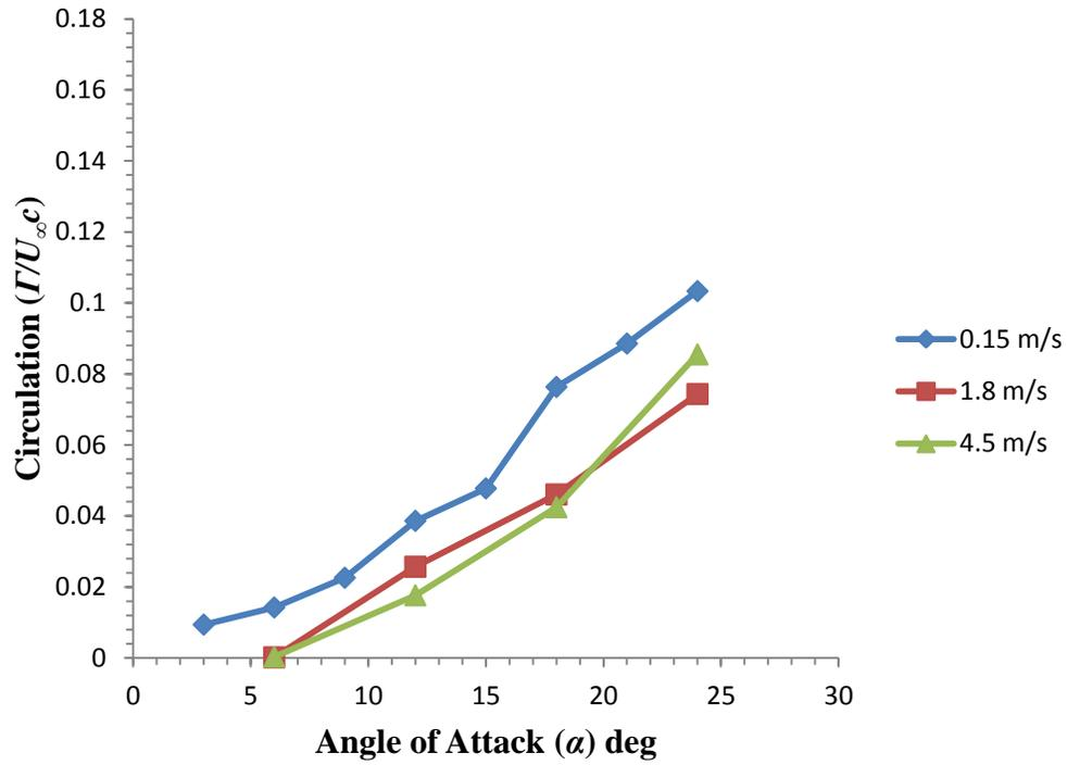
**Figure 77: Averaged  $\Gamma$  of vortices 1-4 shown at multiple freestream velocities as a function of  $\alpha$  at a chordwise spatial location of  $x/c = 0.36c$ .**
