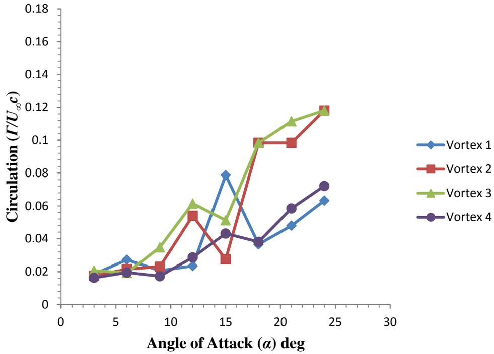
Figure 69:  $\Gamma$  as a function of  $\alpha$  at a chordwise spatial location of  $x/c = 0.25c$ .  $U_\infty = 0.15$  m/s.
