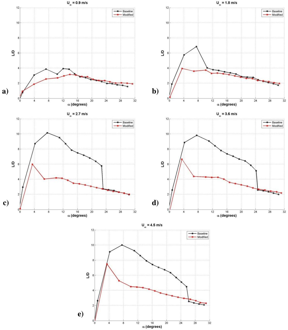
**Figure 54: Swept platform L/D ratio. a)  $Re_c = 9.0 \times 10^4$ , b)  $Re_c = 1.8 \times 10^5$ , c)  $Re_c = 2.7 \times 10^5$ , d)  $Re_c = 3.6 \times 10^5$ , e)  $Re_c = 4.5 \times 10^5$ .**
