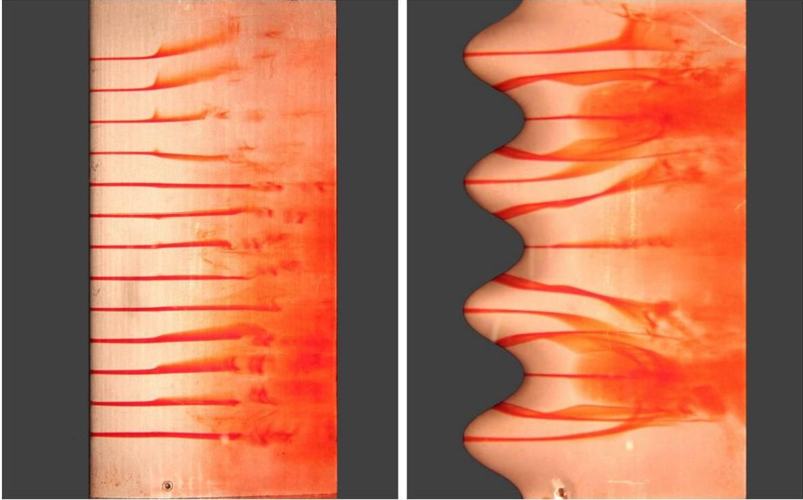
**Figure 84: Dye flow visualization  $\alpha = 6^\circ$ .**
