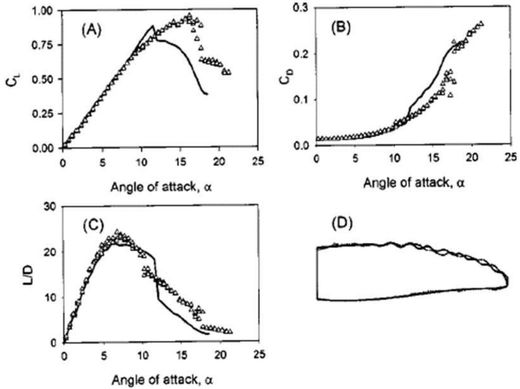
**Figure 3: Top: Flipper models tested by Miklosovic5. Bottom: a) Lift coefficient b) Drag coefficient c) Lift-to-drag ratio d) flipper model design.**
