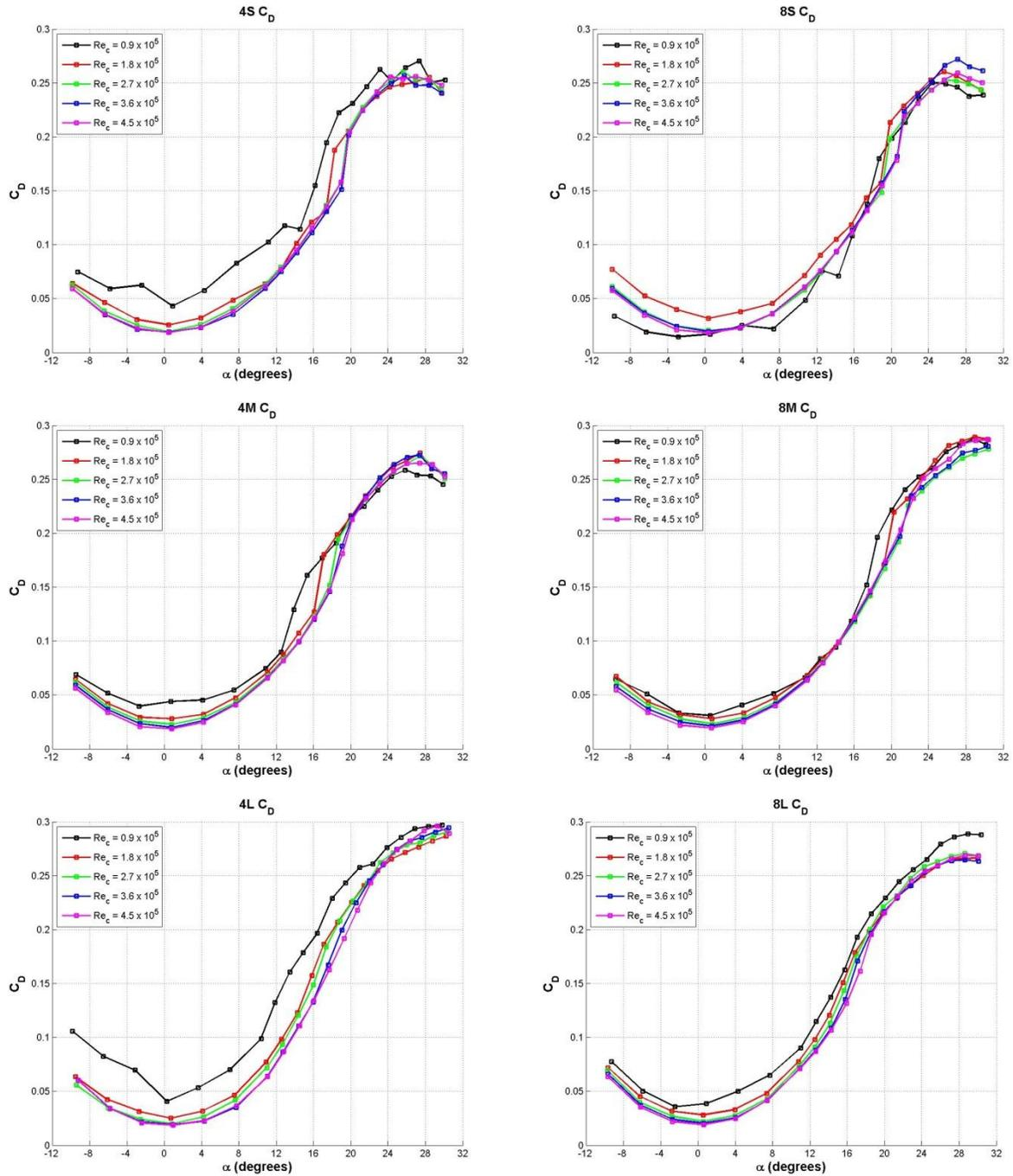
**Figure 26: Effect of Reynolds number on the drag coefficient of finite-span rectangular planform modified hydrofoils. a) 4S, b) 8S, c) 4M, d) 8M, e) 4L, f) 8L.**
