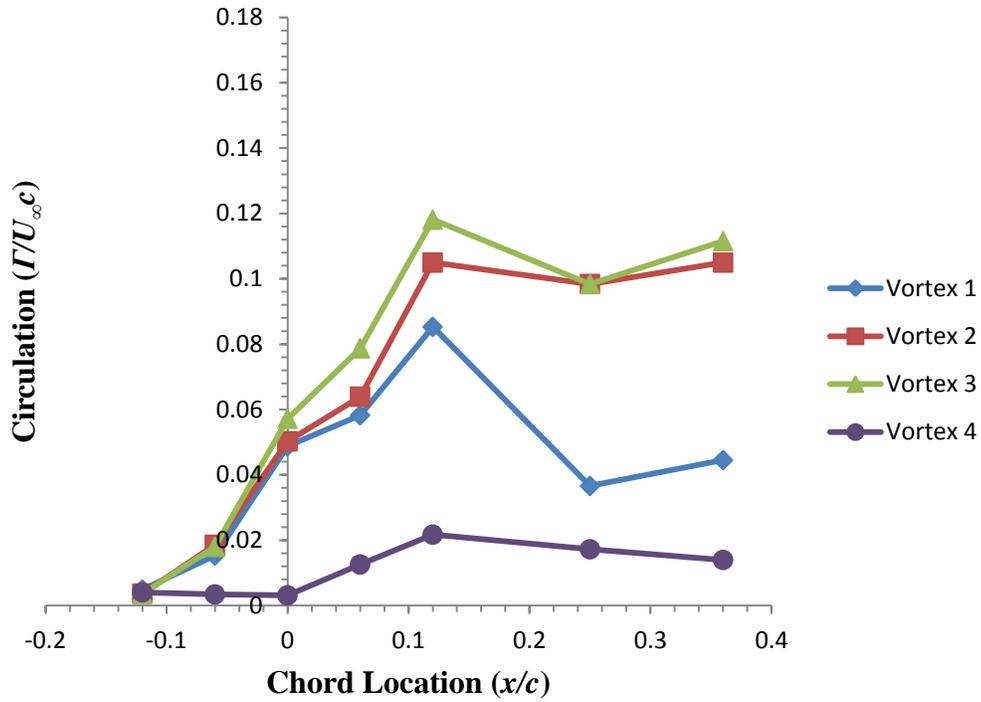
Figure 75:  $\Gamma$  as a function of chordwise spatial location for  $\alpha = 18^\circ$ .  $U_\infty = 0.15$  m/s.
