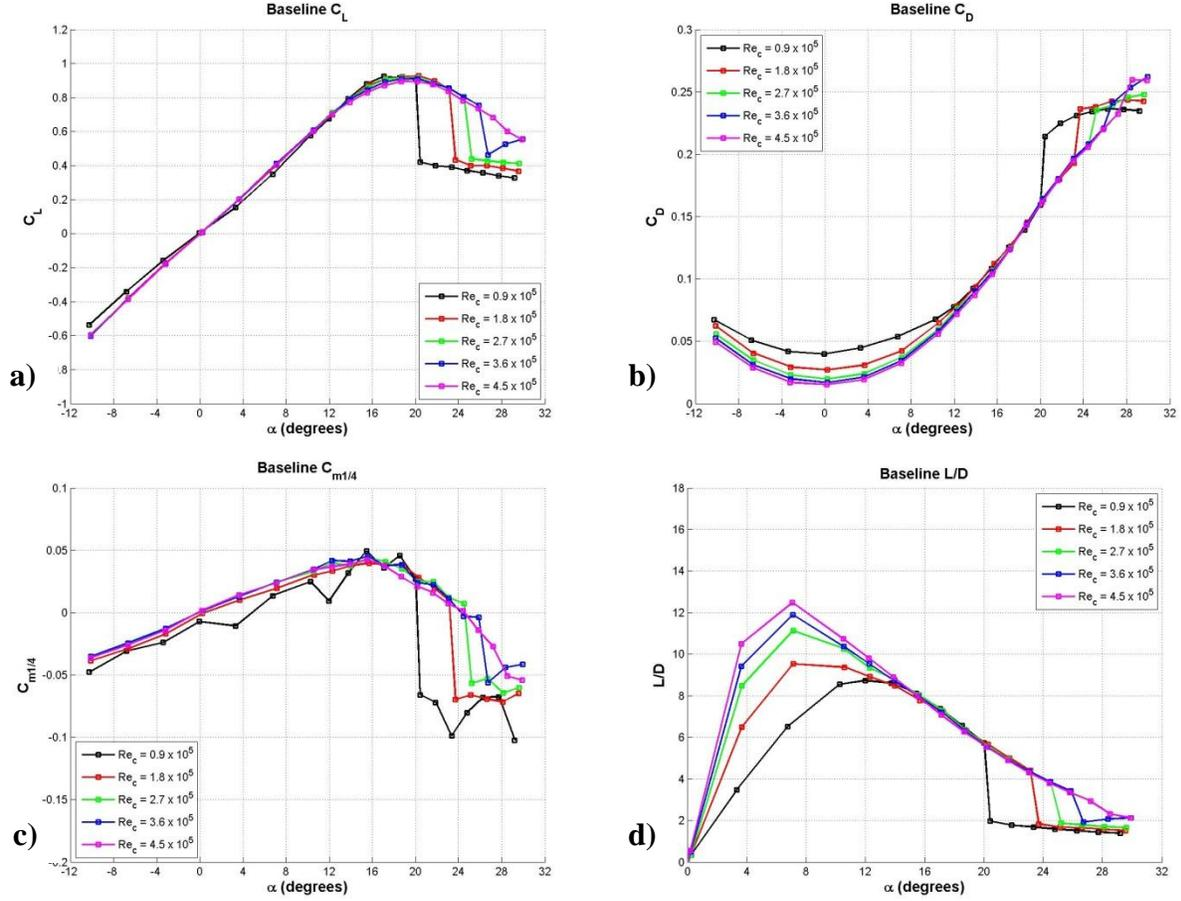
**Figure 24: Effect of Reynolds number on the finite-span rectangular planform baseline hydrofoil load characteristics. a) lift coefficient, b) drag coefficient, c) quarter chord moment coefficient, d)  $L/D$  ratio.**
