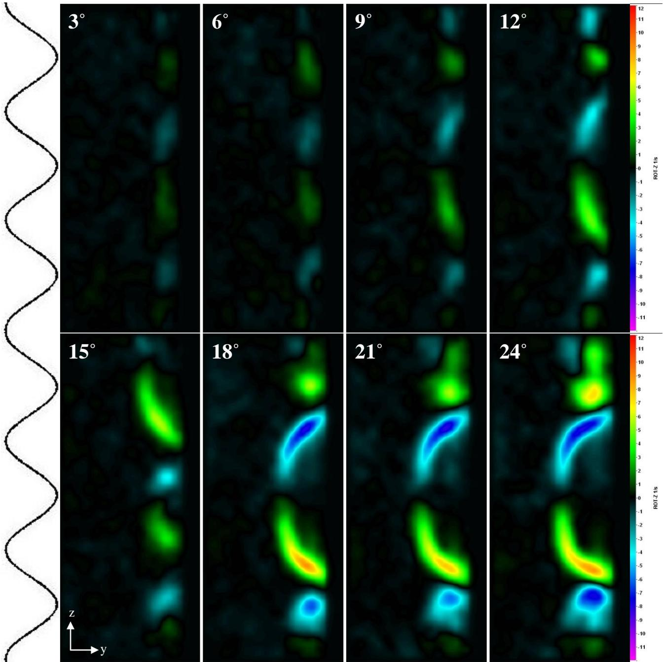
Figure 64: Streamwise vorticity,  $\omega$ , contours on 4L hydrofoil as a function of angle of attack at a chordwise spatial location of  $0.36c$ .
