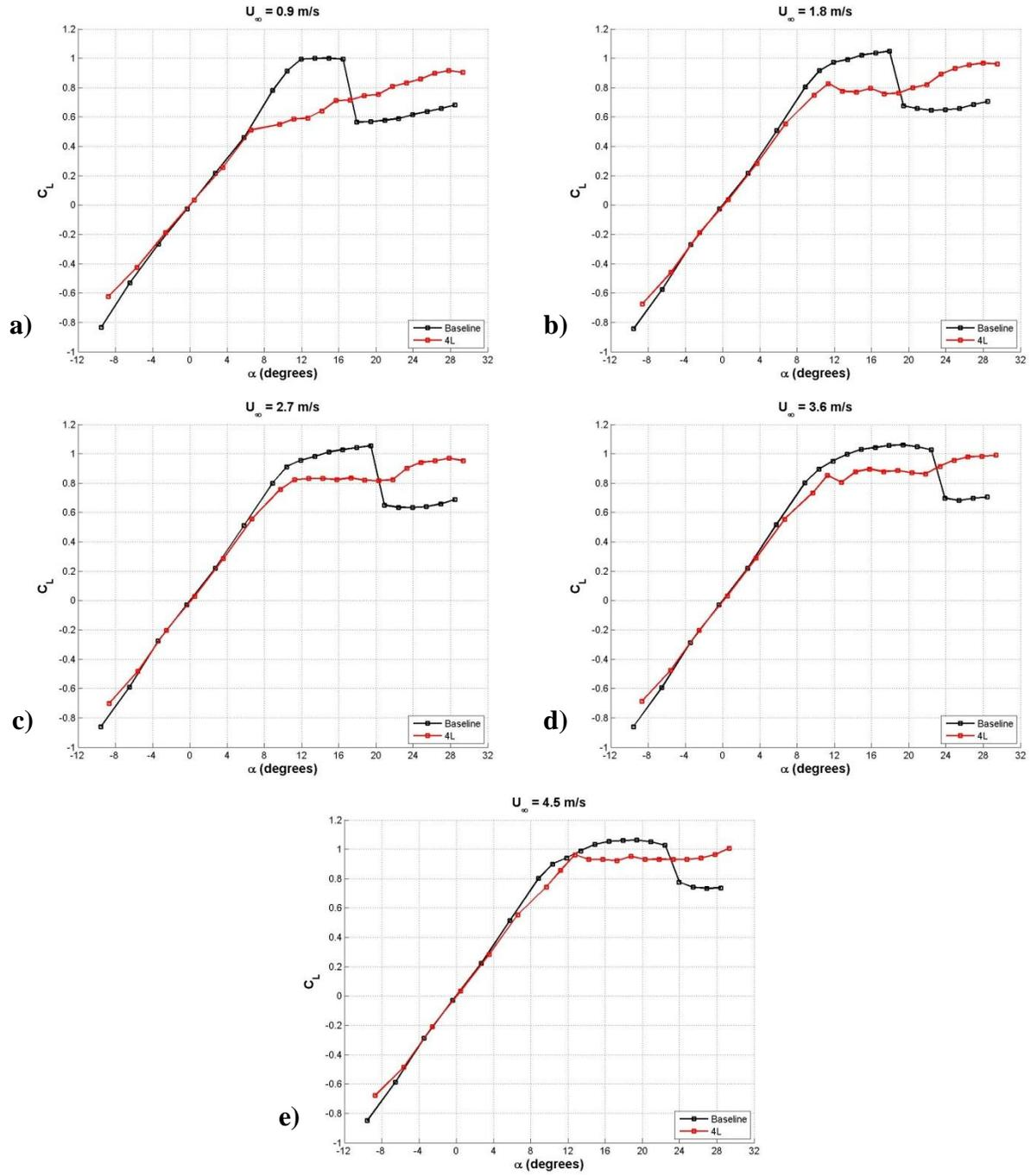
**Figure 20: Infinite-span planform lift coefficient. a)  $Re_c = 9.0 \times 10^4$ , b)  $Re_c = 1.8 \times 10^5$ , c)  $Re_c = 2.7 \times 10^5$ , d)  $Re_c = 3.6 \times 10^5$ , e)  $Re_c = 4.5 \times 10^5$ .**
