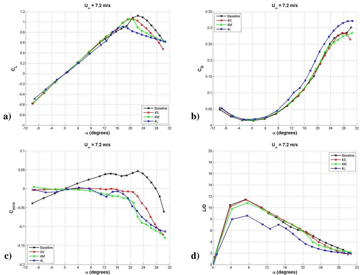
**Figure 94: Effect of protuberance amplitude on the load characteristics of cavitating hydrofoils with a protuberance wavelength of  $\lambda = 0.50c$ ; a) lift coefficient, b) drag coefficient, c) quarter chord moment coefficient, d) lift-to-drag ratio.**
