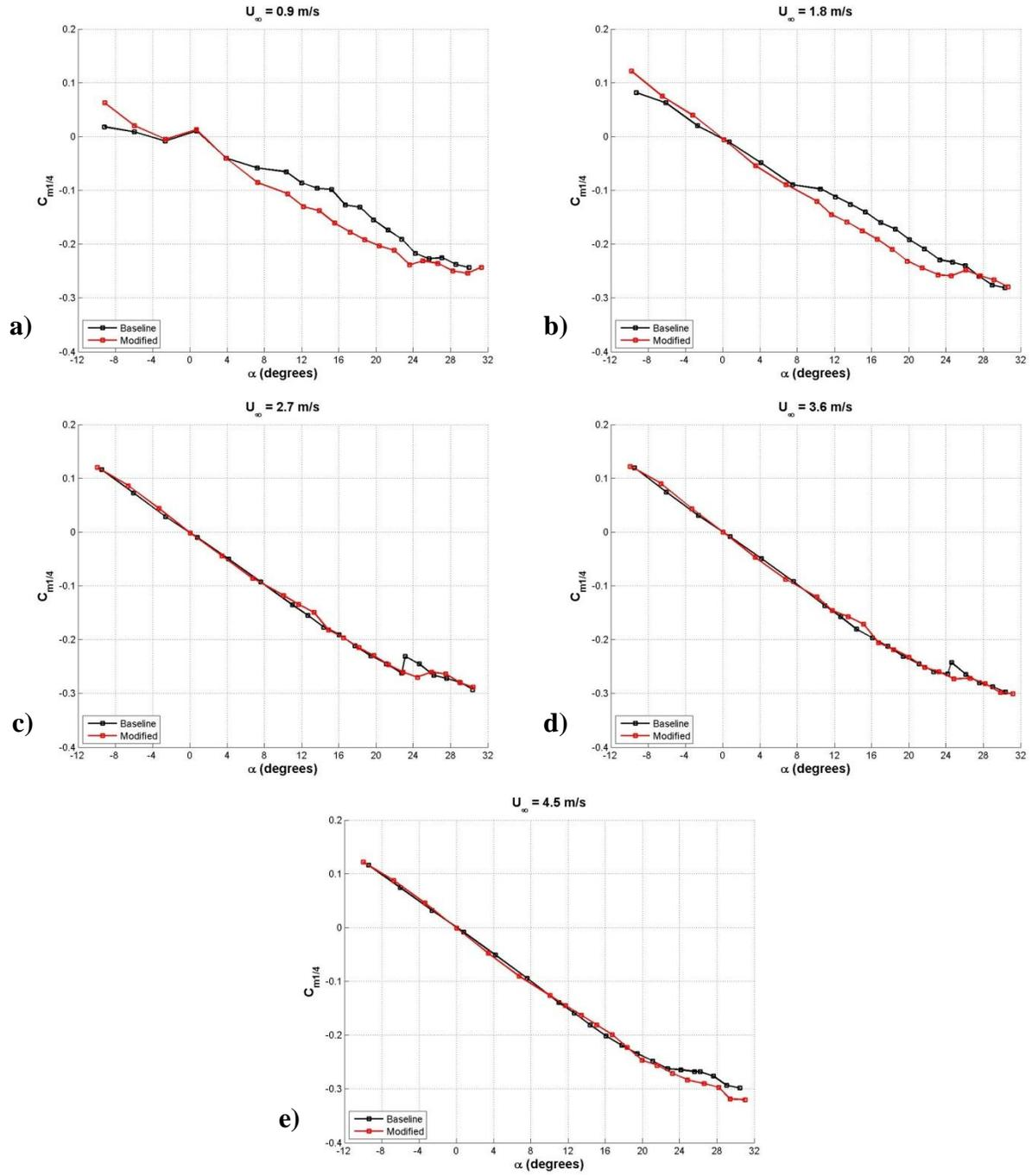
Figure 53: Swept planform quarter chord moment coefficient. a)  $Re_c = 9.0 \times 10^4$ , b)  $Re_c = 1.8 \times 10^5$ , c)  $Re_c = 2.7 \times 10^5$ , d)  $Re_c = 3.6 \times 10^5$ , e)  $Re_c = 4.5 \times 10^5$ .
