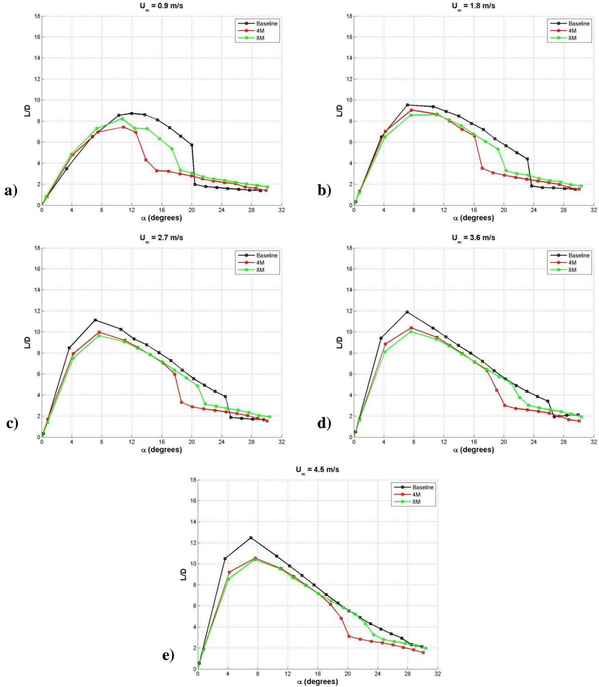
**Figure 44: Effect of protuberance wavelength on the lift-to-drag ratio of finite-span rectangular planform hydrofoils,  $A = 0.050c$ . a)  $Re_c = 9.0 \times 10^4$ , b)  $Re_c = 1.8 \times 10^5$ , c)  $Re_c = 2.7 \times 10^5$ , d)  $Re_c = 3.6 \times 10^5$ , e)  $Re_c = 4.5 \times 10^5$ .**
