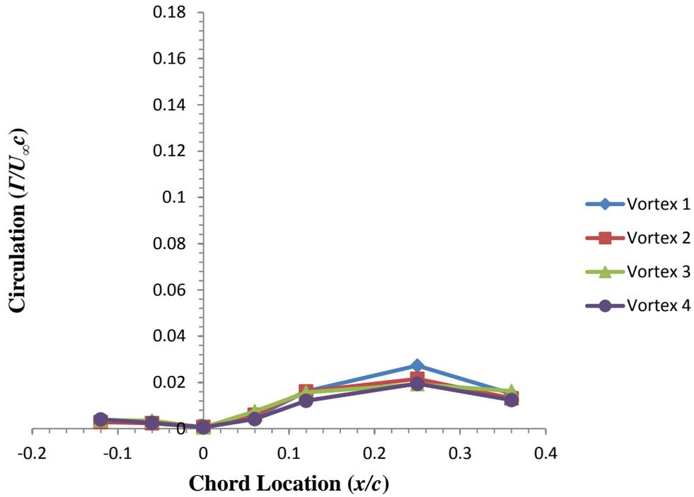
Figure 73:  $\Gamma$  as a function of chordwise spatial location for  $\alpha = 6^\circ$ .  $U_\infty = 0.15$  m/s.
