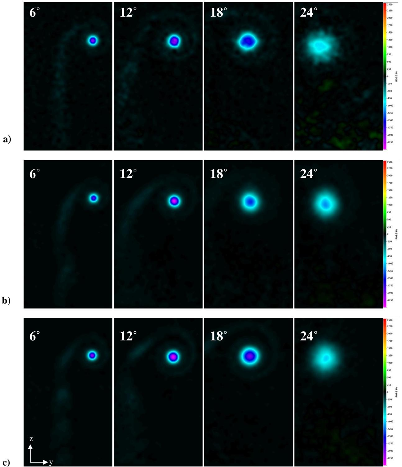
Figure 81: Streamwise vorticity contours of the tip vortex on finite-span rectangular hydrofoils 3.00c downstream of baseline hydrofoil leading edge.  $U_\infty = 4.5$  m/s. a) Baseline b) 4L c) 8M.
