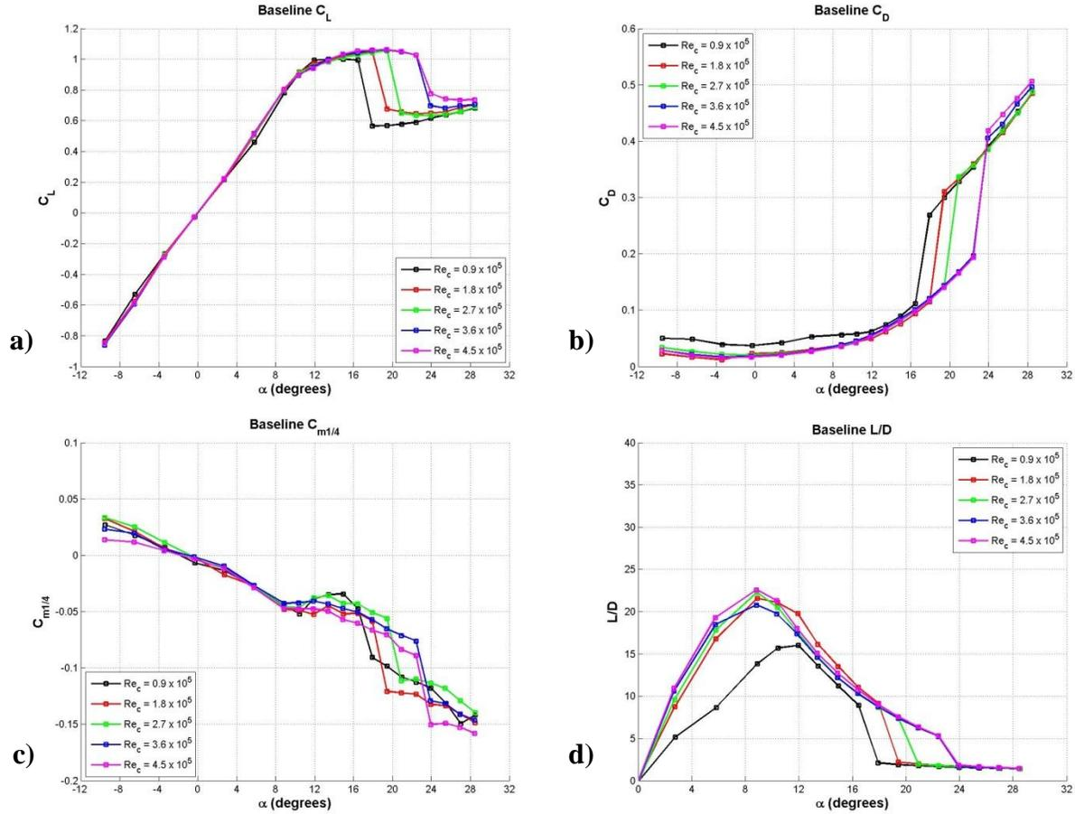
**Figure 17: Full-span baseline hydrofoil load characteristics at multiple Reynolds numbers. a) lift coefficient, b) drag coefficient, c) quarter chord moment coefficient, d) L/D ratio.**
