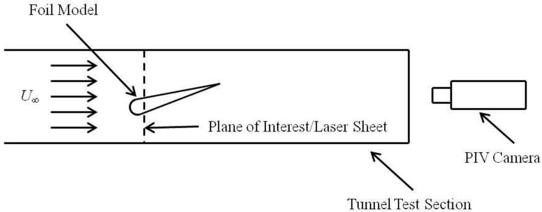
**Figure 14: Schematic of full-span low-speed PIV system and water tunnel.**
