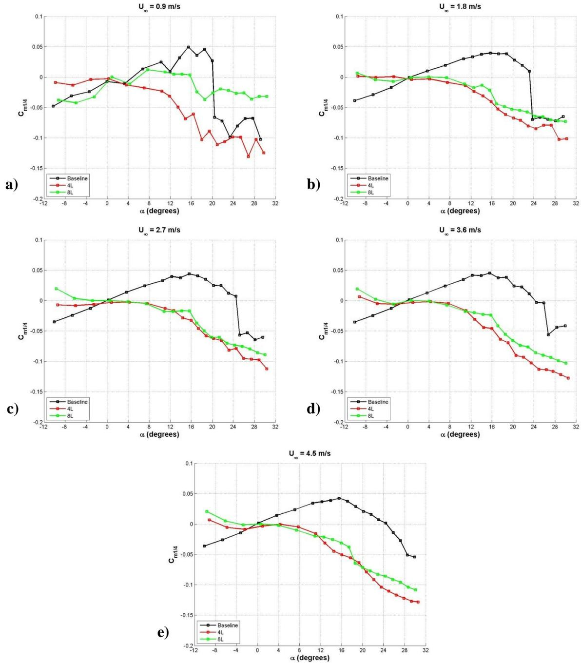
**Figure 47: Effect of protuberance wavelength on the quarter chord moment coefficient of finite-span rectangular planform hydrofoils,  $A = 0.120c$ . a)  $Re_c = 9.0 \times 10^4$ , b)  $Re_c = 1.8 \times 10^5$ , c)  $Re_c = 2.7 \times 10^5$ , d)  $Re_c = 3.6 \times 10^5$ , e)  $Re_c = 4.5 \times 10^5$ .**
