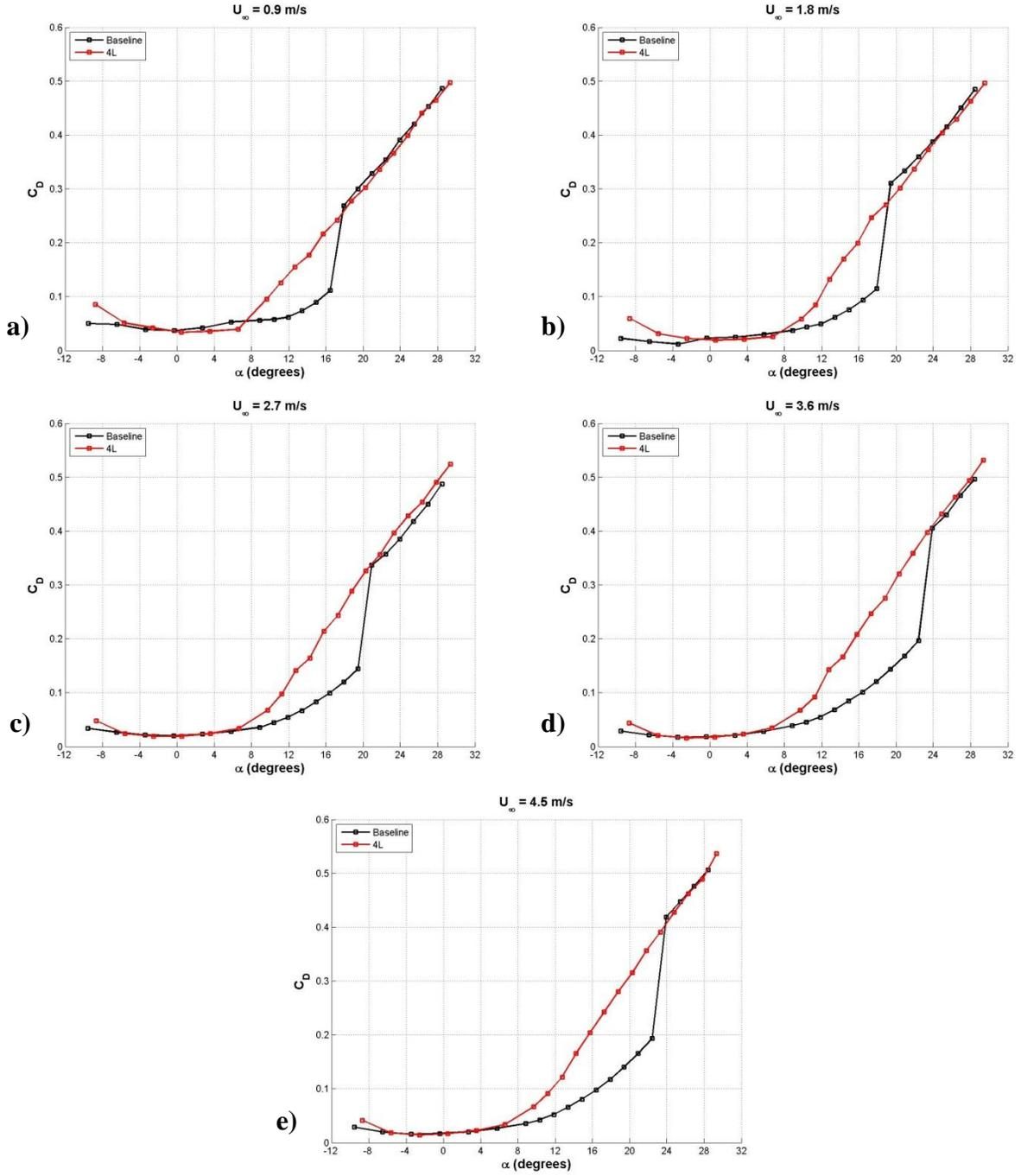
**Figure 21: Infinite-span planform drag coefficient. a)  $Re_c = 9.0 \times 10^4$ , b)  $Re_c = 1.8 \times 10^5$ , c)  $Re_c = 2.7 \times 10^5$ , d)  $Re_c = 3.6 \times 10^5$ , e)  $Re_c = 4.5 \times 10^5$ .**
