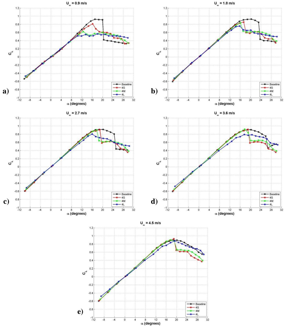
**Figure 29: Effect of protuberance amplitude on the lift coefficient of finite-span rectangular planform hydrofoils,  $\lambda = 0.50c$ . a)  $Re_c = 9.0 \times 10^4$ , b)  $Re_c = 1.8 \times 10^5$ , c)  $Re_c = 2.7 \times 10^5$ , d)  $Re_c = 3.6 \times 10^5$ , e)  $Re_c = 4.5 \times 10^5$ .**
