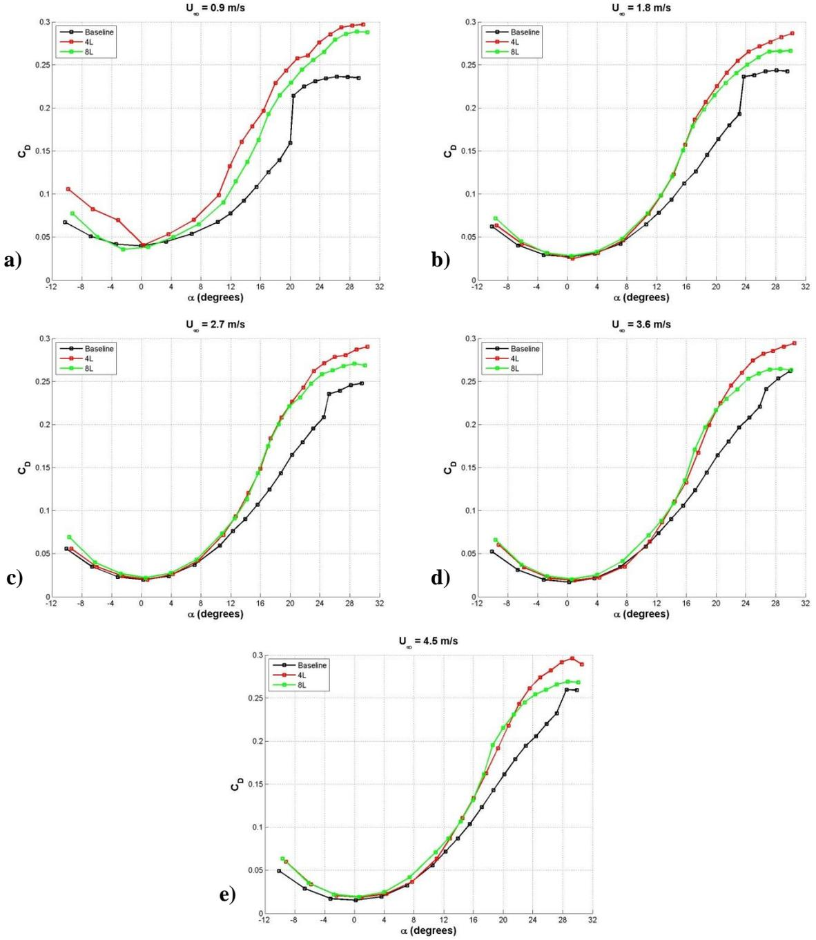
**Figure 46: Effect of protuberance wavelength on the drag coefficient of finite-span rectangular planform hydrofoils,  $A = 0.120c$ . a)  $Re_c = 9.0 \times 10^4$ , b)  $Re_c = 1.8 \times 10^5$ , c)  $Re_c = 2.7 \times 10^5$ , d)  $Re_c = 3.6 \times 10^5$ , e)  $Re_c = 4.5 \times 10^5$ .**
