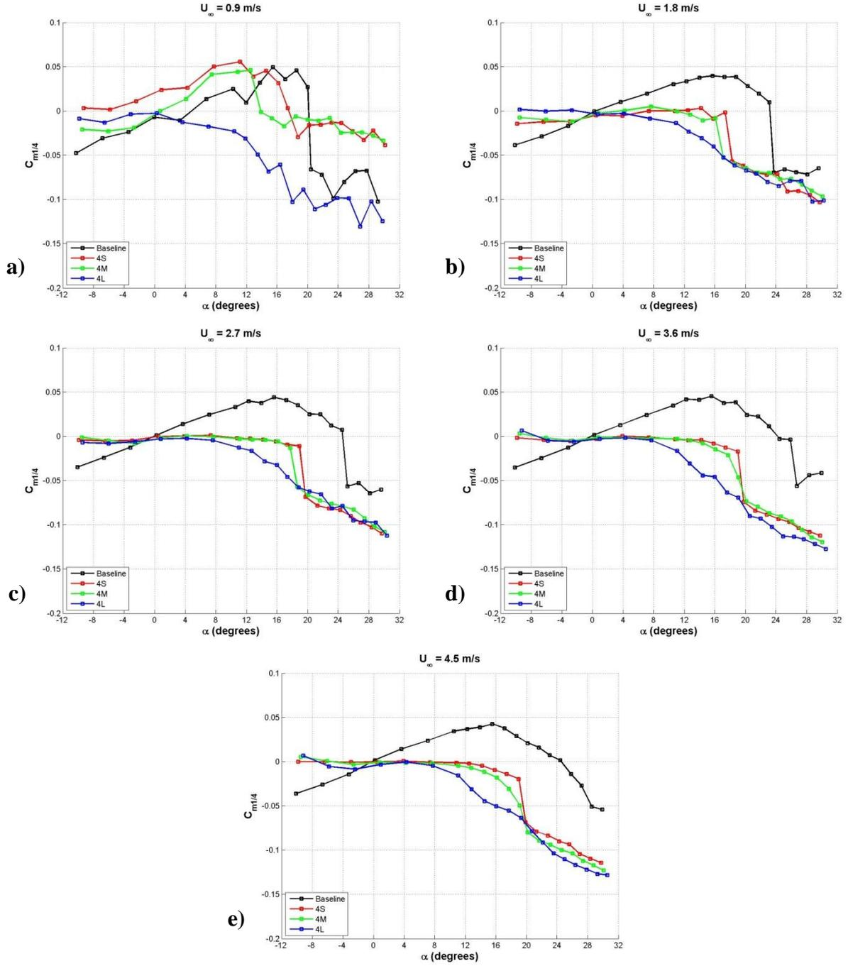
**Figure 31: Effect of protuberance amplitude on the quarter chord moment coefficient of finite-span rectangular planform hydrofoils,  $\lambda = 0.50c$ . a)  $Re_c = 9.0 \times 10^4$ , b)  $Re_c = 1.8 \times 10^5$ , c)  $Re_c = 2.7 \times 10^5$ , d)  $Re_c = 3.6 \times 10^5$ , e)  $Re_c = 4.5 \times 10^5$ .**
