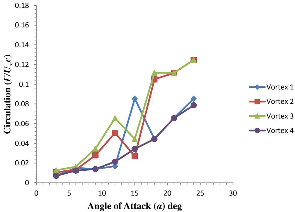
Figure 70:  $\Gamma$  as a function of  $\alpha$  at a chordwise spatial location of  $x/c = 0.36c$ .  $U_\infty = 0.15$  m/s.
