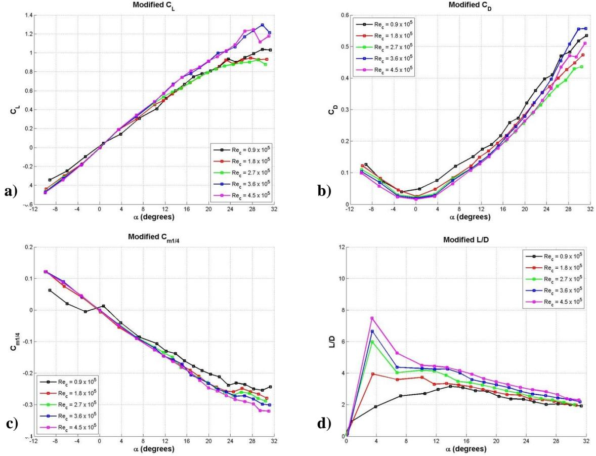
**Figure 50: Effect of Reynolds number on the swept planform modified hydrofoil load characteristics. a) lift coefficient, b) drag coefficient, c) quarter chord moment coefficient, d) L/D ratio.**
