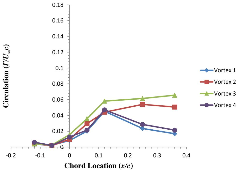
Figure 74:  $\Gamma$  as a function of chordwise spatial location for  $\alpha = 12^\circ$ .  $U_\infty = 0.15$  m/s.
