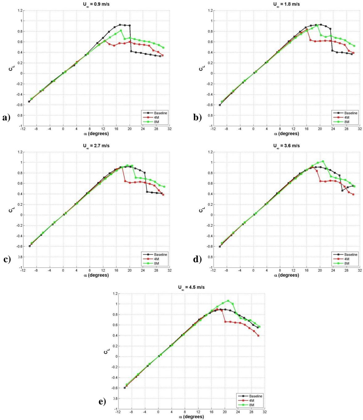
**Figure 41: Effect of protuberance wavelength on the lift coefficient of finite-span rectangular planform hydrofoils,  $A = 0.050c$ . a)  $Re_c = 9.0 \times 10^4$ , b)  $Re_c = 1.8 \times 10^5$ , c)  $Re_c = 2.7 \times 10^5$ , d)  $Re_c = 3.6 \times 10^5$ , e)  $Re_c = 4.5 \times 10^5$ .**
