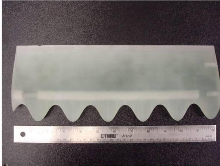
**Figure 7: 4L SLA hydrofoil used in low-speed PIV water tunnel experiments.**
