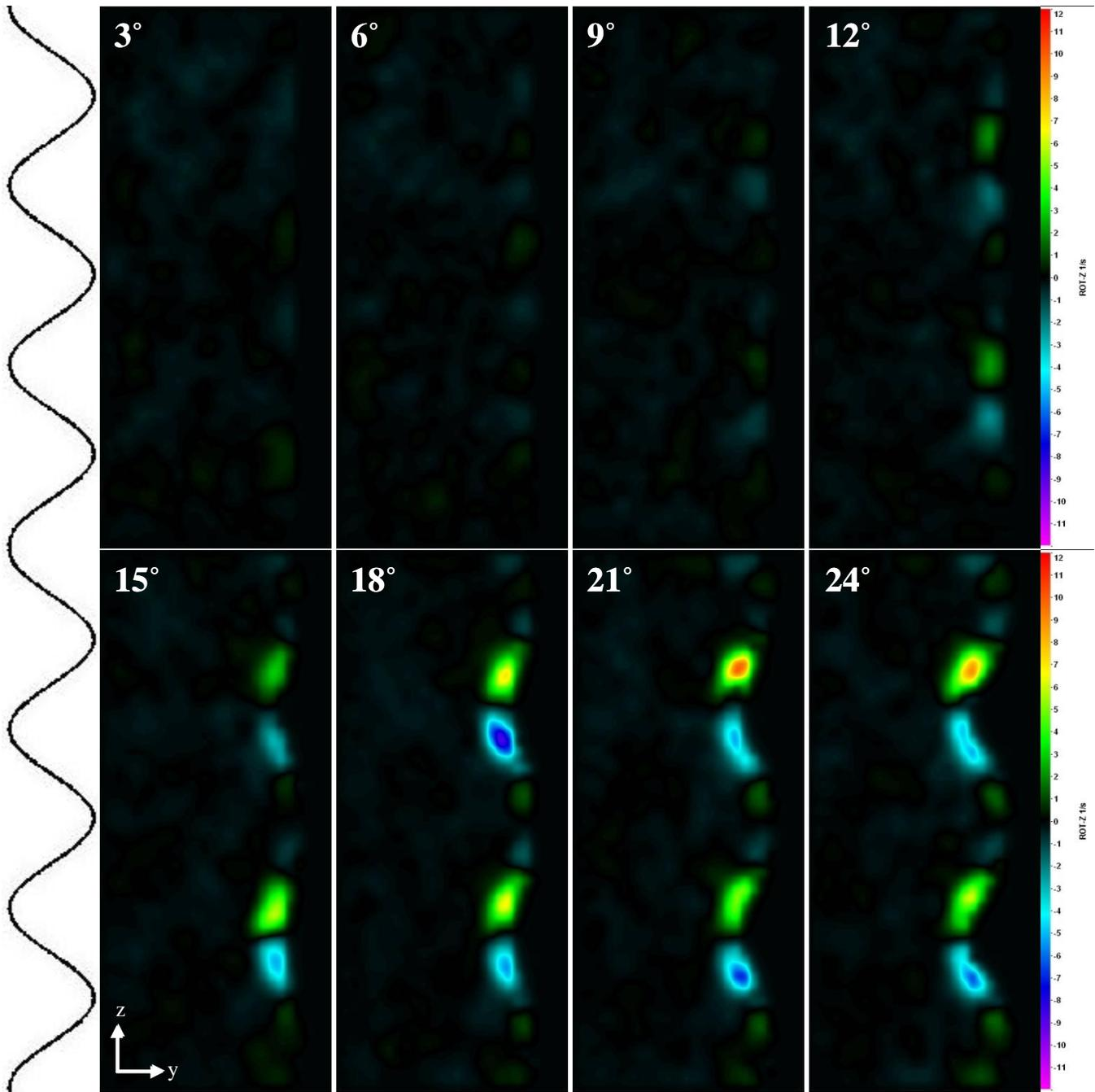
Figure 61: Streamwise vorticity,  $\omega$ , contours on 4L hydrofoil as a function of angle of attack at a chordwise spatial location of  $0c$ .
