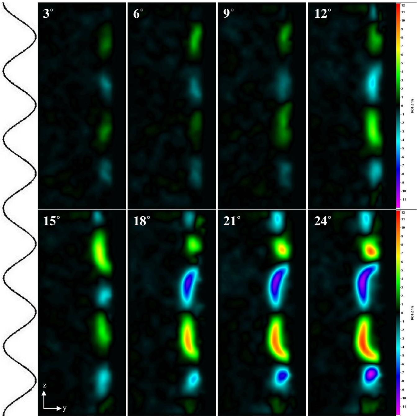
Figure 63: Streamwise vorticity,  $\omega$ , contours on 4L hydrofoil as a function of angle of attack at a chordwise spatial location of  $0.25c$ .
