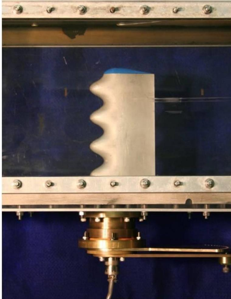
**Figure 11: 4L finite-span rectangular hydrofoil in water tunnel test section with yaw mechanism attached.**
