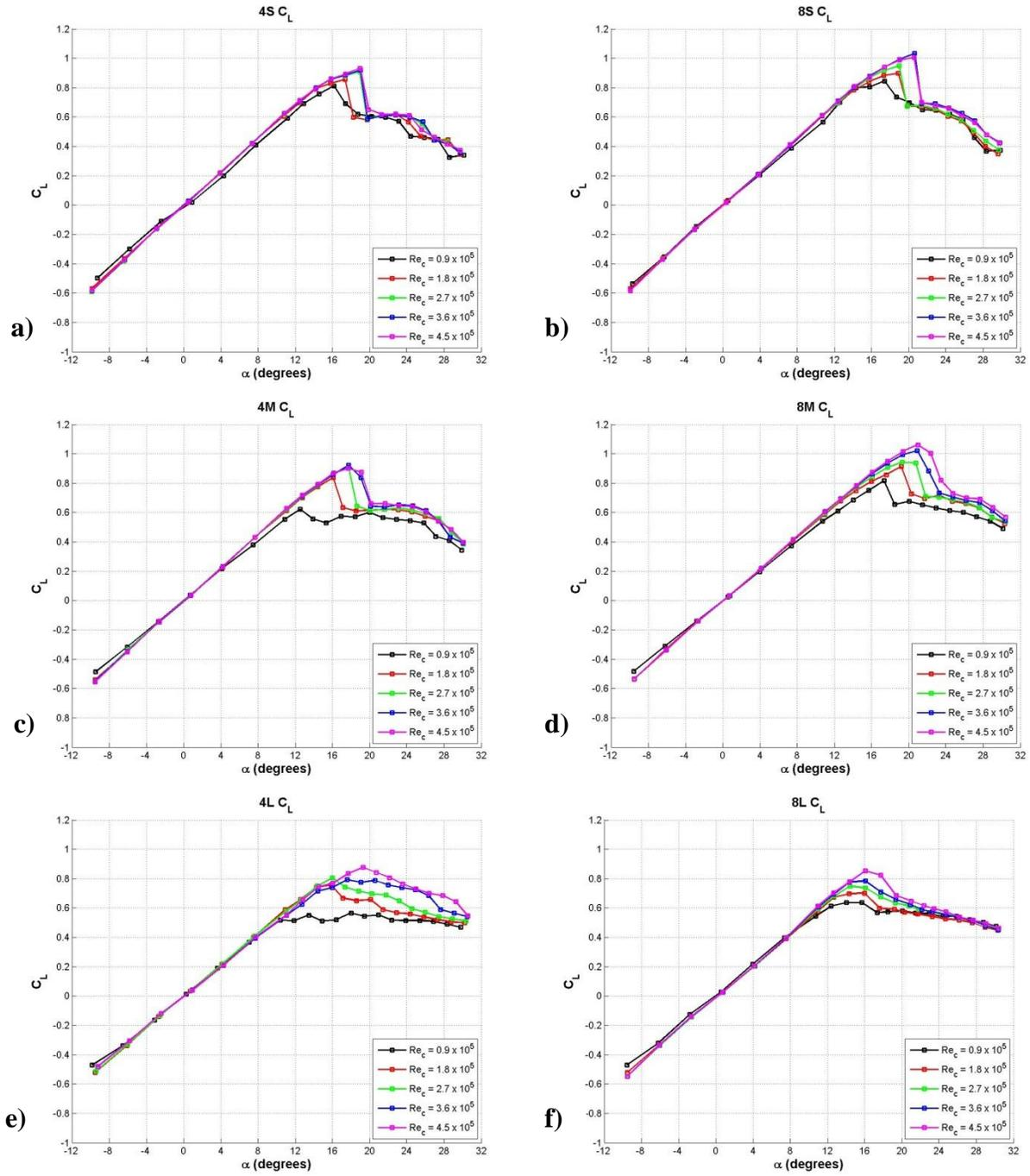
**Figure 25: Effect of Reynolds number on the lift coefficient of finite-span rectangular planform modified hydrofoils. a) 4S, b) 8S, c) 4M, d) 8M, e) 4L, f) 8L.**
