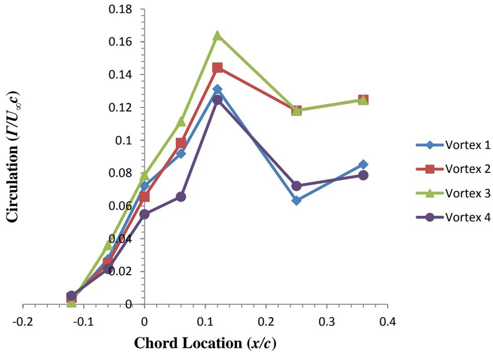
Figure 76:  $\Gamma$  as a function of chordwise spatial location for  $\alpha = 24^\circ$ .  $U_\infty = 0.15$  m/s.
