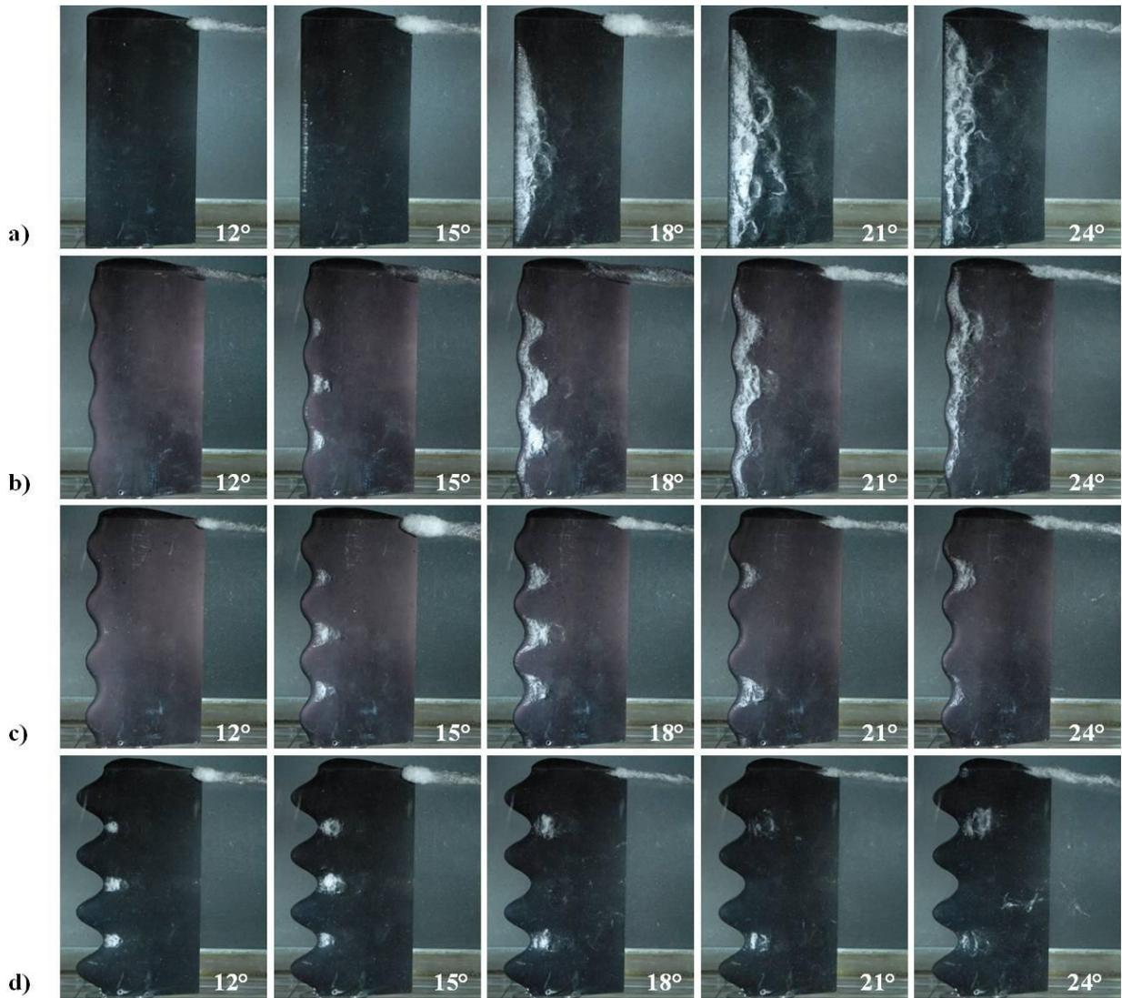
**Figure 91: Vaporous cavitation on the leading edge and tip vortex of finite-span rectangular hydrofoils; a) baseline, b) 4S, c) 4M, and d) 4L.**
