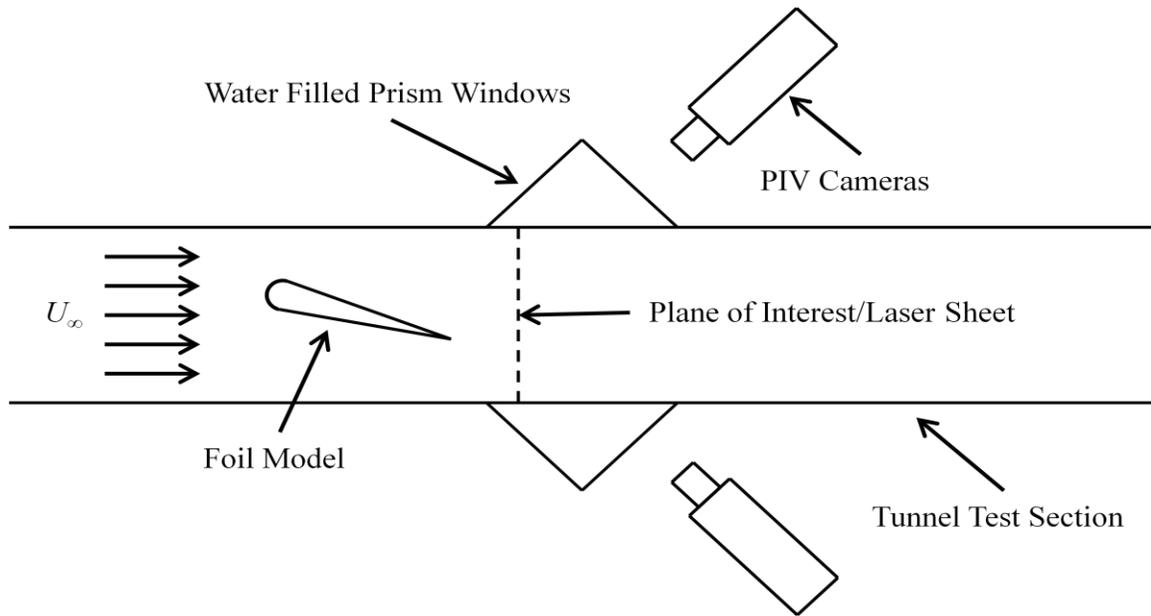
**Figure 16: Schematic of finite-span high-speed SPIV system and water tunnel used for tip vortex analysis.**
