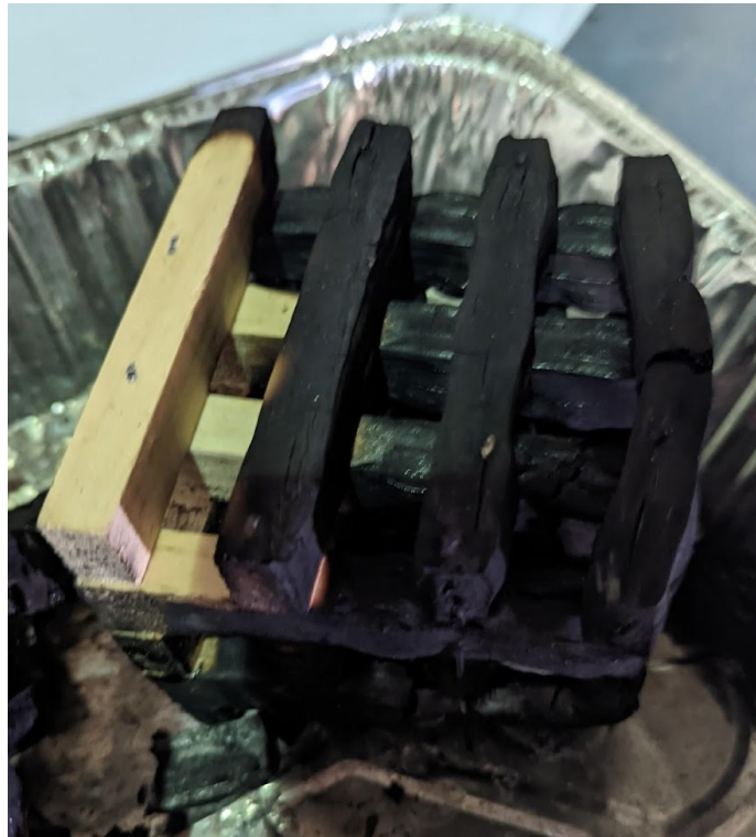
Figure 9. Fully extinct wood crib.
