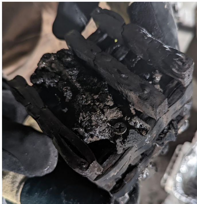
Figure 11. Fully extinct PVC crib.
