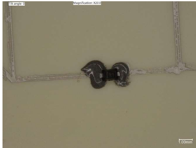
Figure 77: Surface Mount Diode Component as Seen Under Microscope
