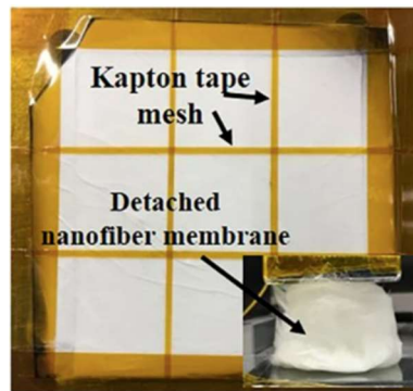
Figure 14: Nanofiber Membrane Attached at an Electrode using Kapton Tape
