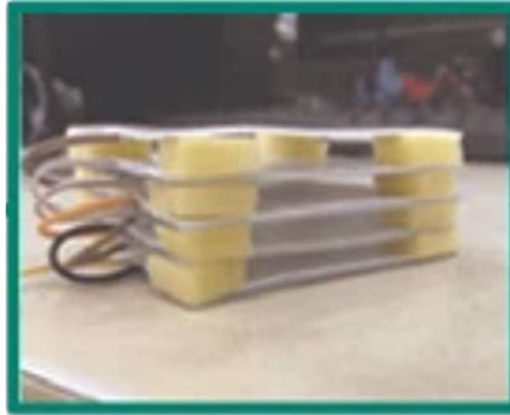
Figure 90: Spacing for TENG from Literature
