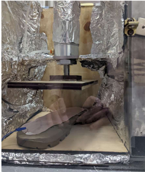
Figure 119: Midsole I Prototype Automated Testing
