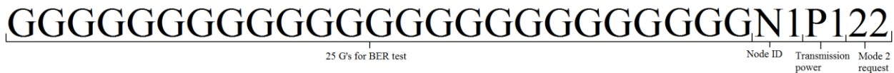
Figure 40: Each node sends 25 ASCII G's for a BER link test, its ASCII node ID, the transmit power level and the mode 2 request in each link assessment request payload.
