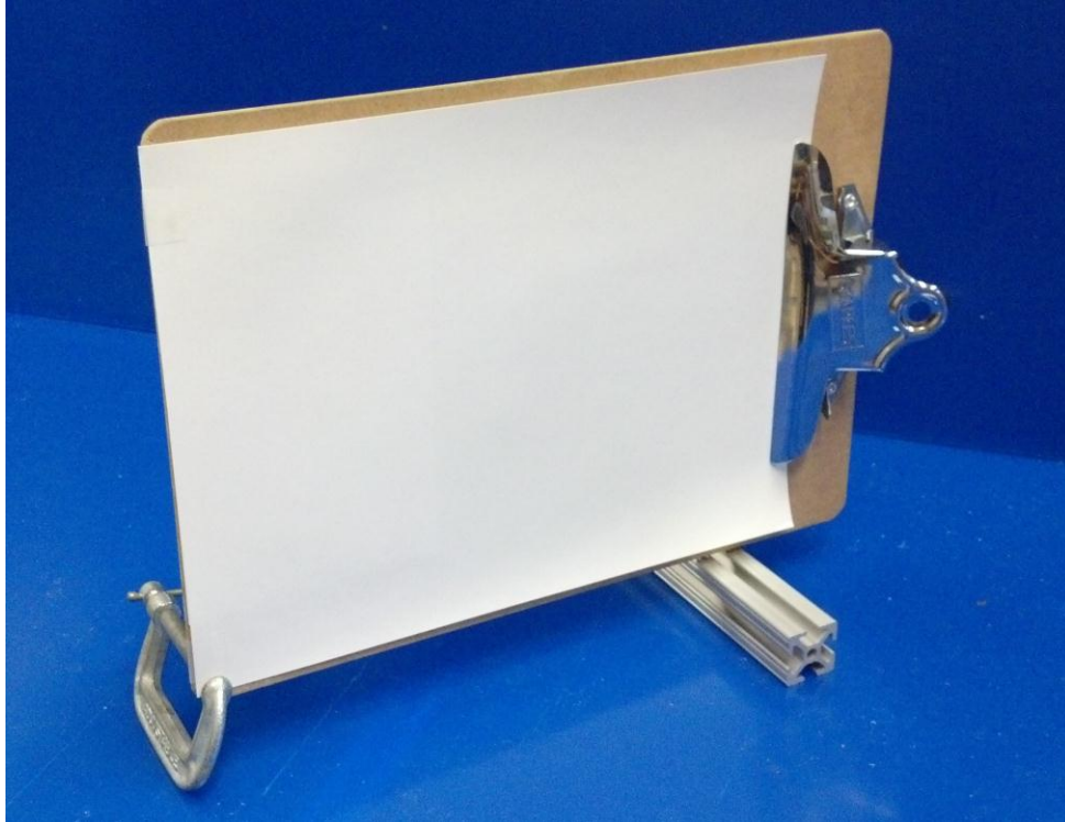
Figure 45: Screen used in z-type schlieren system
