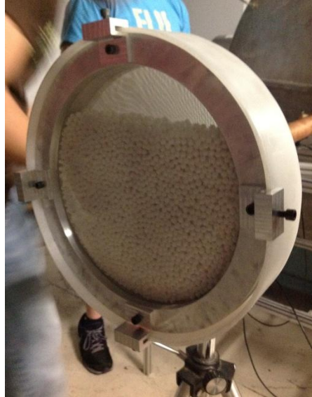
Figure 62: Assembled air drier showing flaw in desiccant bead packing
