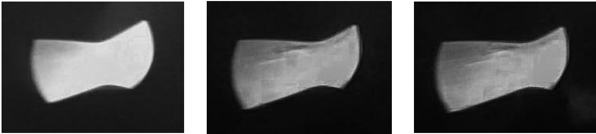
Figure 60: Schlieren results (a) before introducing flow, (b) and (c) during testing
