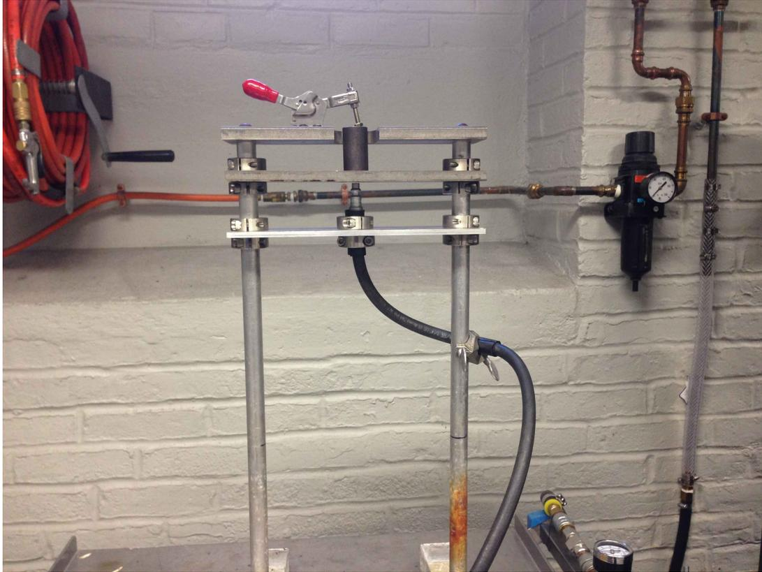
Figure 1.14 CHTE gas quench test device
