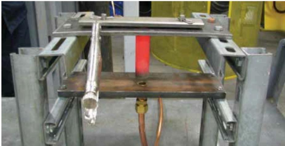
Figure 1.10 Solar Atmosphere Jominy gas quench test (room pressure)<sup>12</sup>
