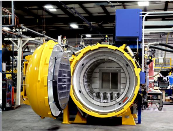
Figure 1.4 Solar Atmosphere gas quench system<sup>4</sup>
