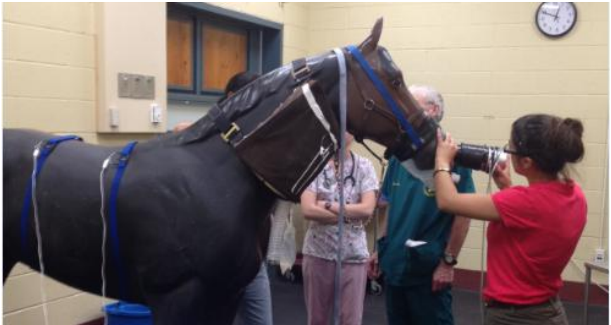
FIGURE 5: PLACEMENT OF RESPIRATORY INDUCTANCE BANDS ON ARTIFICIAL HORSE.
