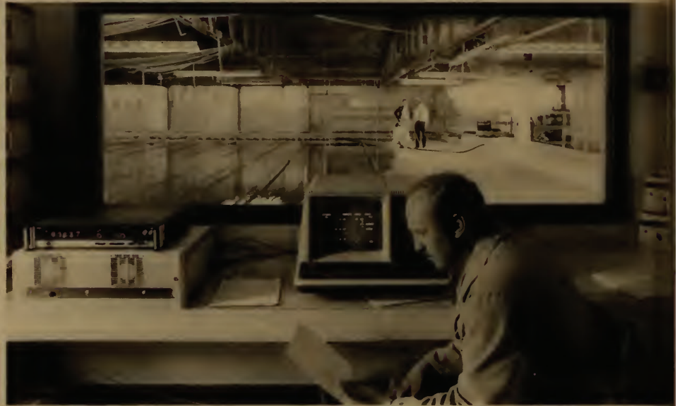
The instrument room, which overlooks the huge modeling area, is used for studies like the one of a Taiwan power system. From left are the minicomputer and digital voltmeter; the video terminal, which displays real-time temperatures in the model; and the automatic controllers for building atmosphere and sump water temperature.
