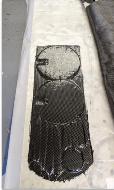
Figure 47 Fuselage Carbon Fiber Mold Post Vacuum
