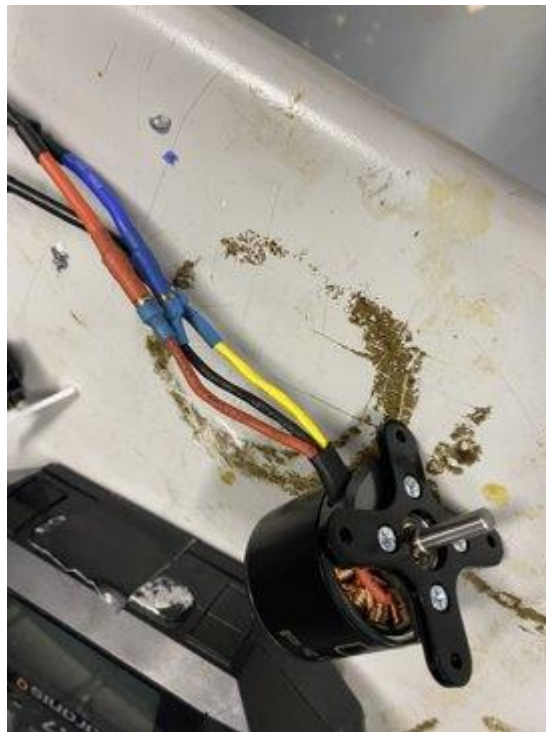
Figure 52 Motor Connected to ESC through Wire Connectors and Heat Shrink
