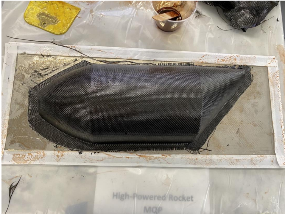
Figure 50 Carbon Fiber Layup of Fuselage Shell Before Treatment
