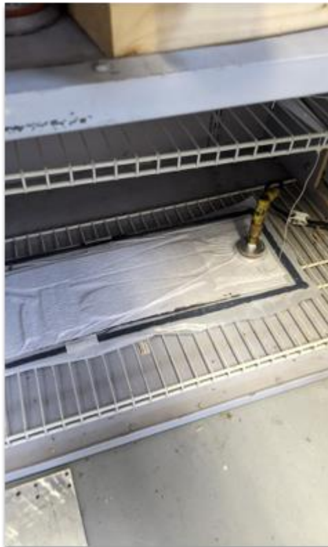
Figure 47 Fuselage Carbon Fiber Mold Post Vacuum
