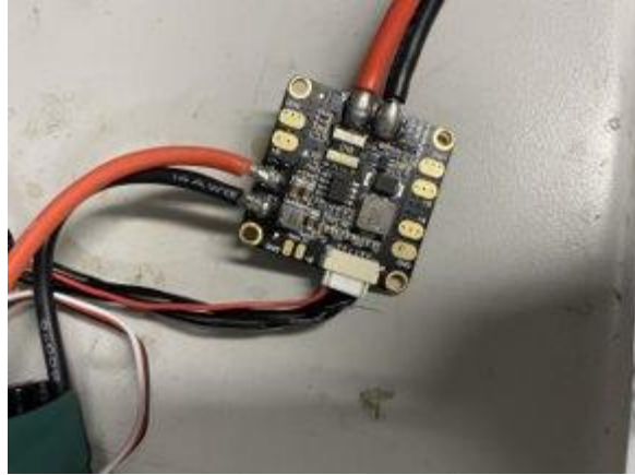
Figure 51 Soldered Power Module Connected to ESC, Flight Controller, and Battery
