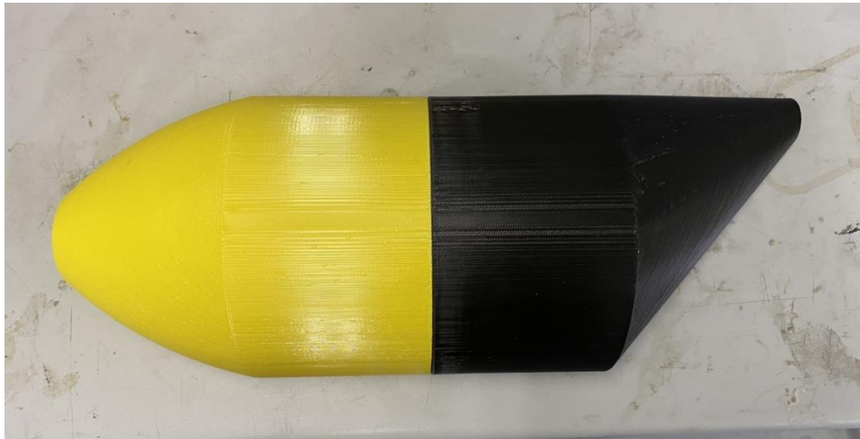
Figure 49 3-D Printed Structure Used to Shape Fuselage Mold
