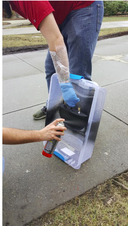
Figure 18: Applying rubberized sealant to the wing
