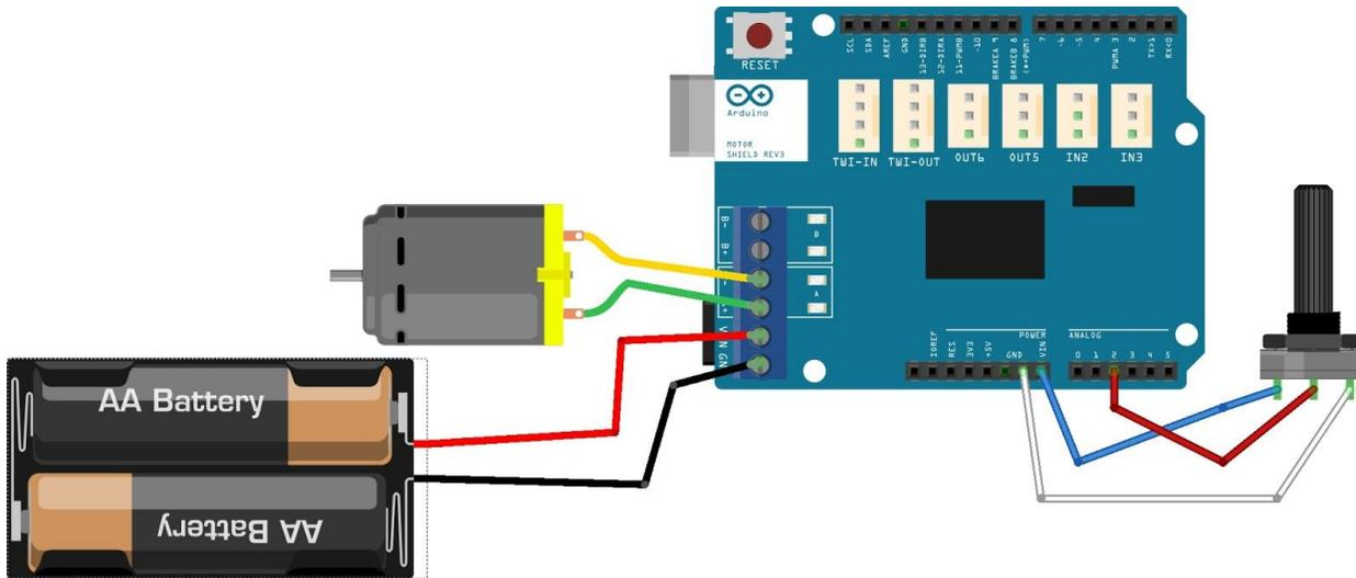
Figure 18: Diagram of the connection with the stronger motor, using an attached power source
