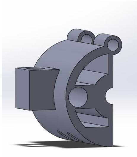
*Figure 54: Outer side of the needle clamp*
