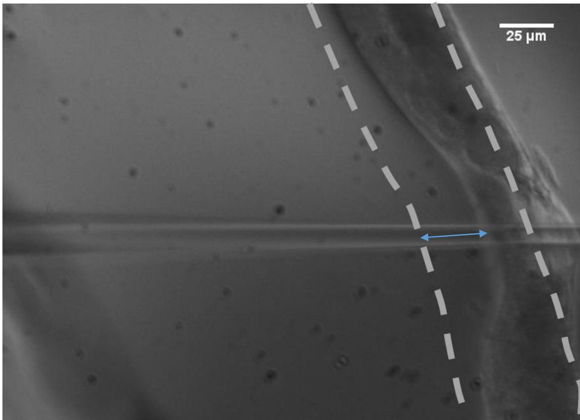
Figure 48: Injection without Vibration, with the blue line representing the deformation measurement
