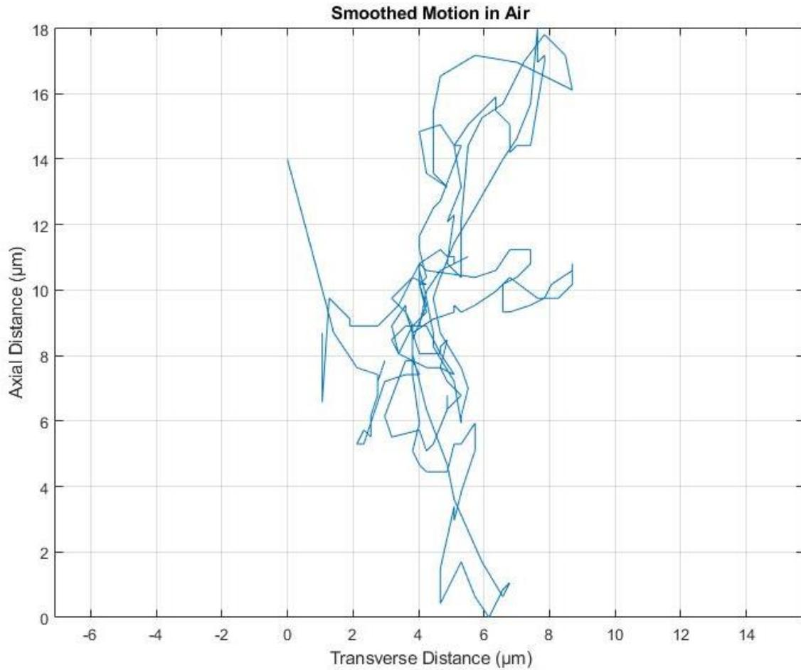
Figure 43: Two hundred points tracked and then put through a moving average filter
