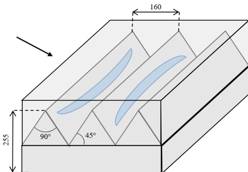
Figure 38: Cross section of hydrogel system, with the arrow representing direction of the needle and the units in  $\mu\text{m}$
