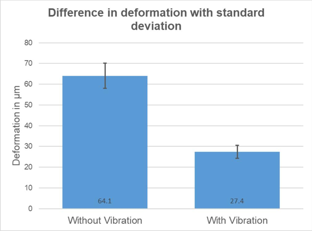
Figure 50: Deformation difference, between with and without vibration
