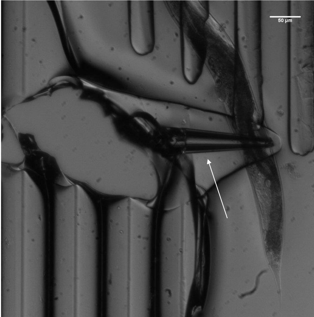
Figure 27: Cross-linked microstructure with encapsulated *C. elegans*, with broken needle tip shown by the white arrow
