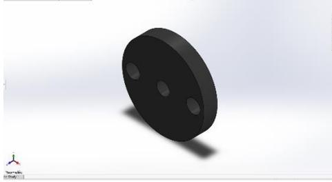
Figure 55: Vibration dampening pad, two in the final design
