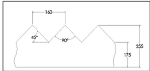
Figure 35: Cross section of final mold used, dimensions in  $\mu\text{m}$
