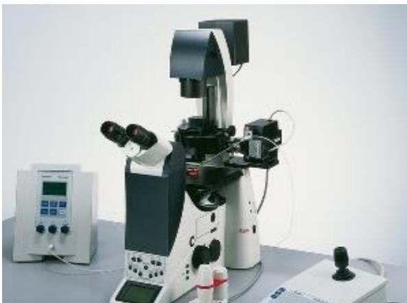
Figure 10: Patchman<sup>TM</sup> NP 2 micromanipulator and FemtoJet that was used for testing [19]
