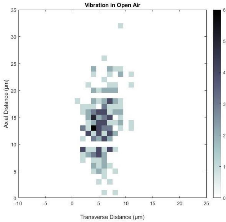
Figure 46: Heat map of the motion of the needle in open air, using two hundred tracked points and darker colors representing higher number of occurrences
