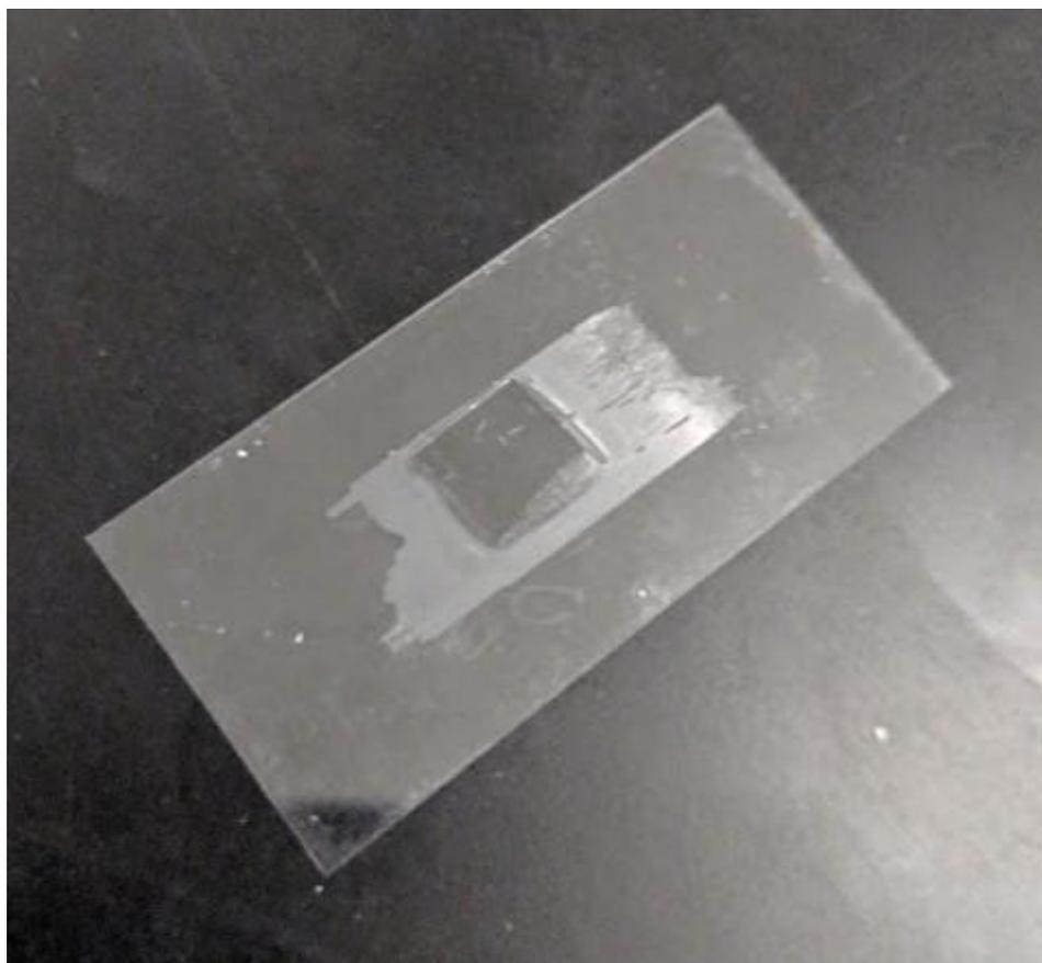
*Figure 33: Hydrogel containment created using square PDMS spacer*
