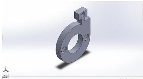
Figure 56: End cap for the case
