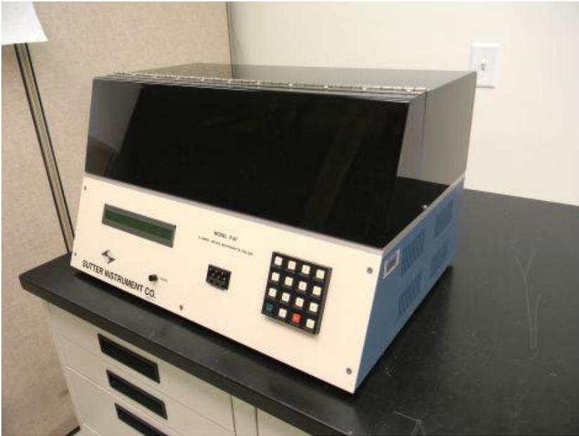
Figure 5: Micropipette Puller
