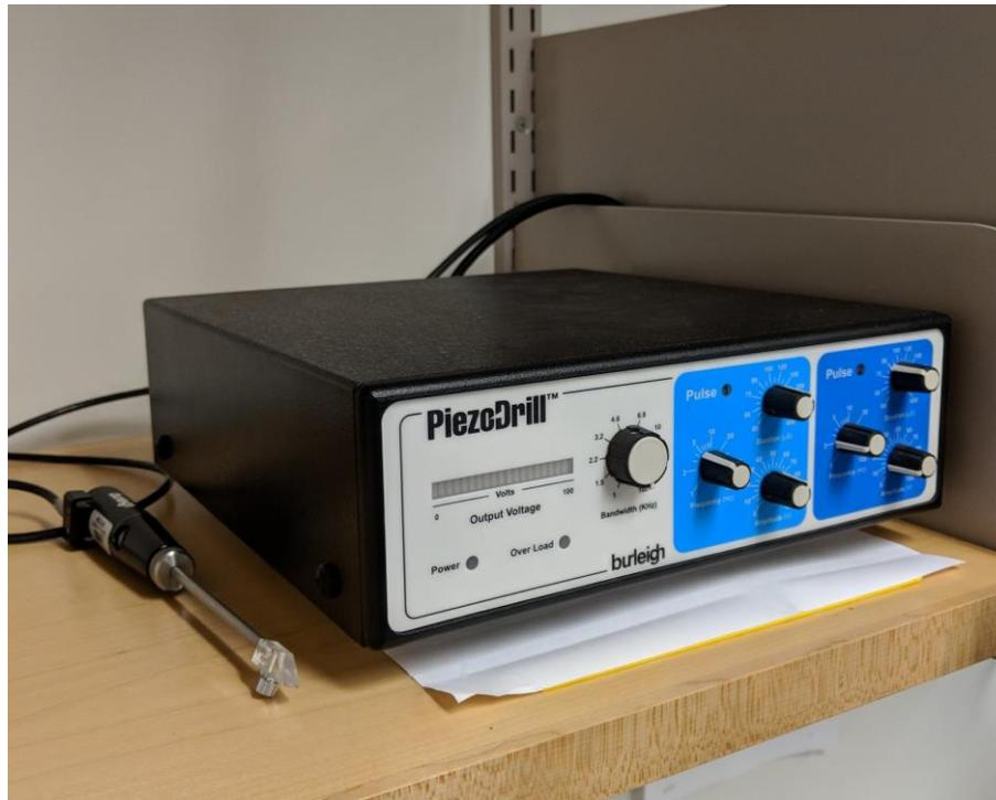
*Figure 9: The PiezoDrill, and example of the piezo impact drive*
