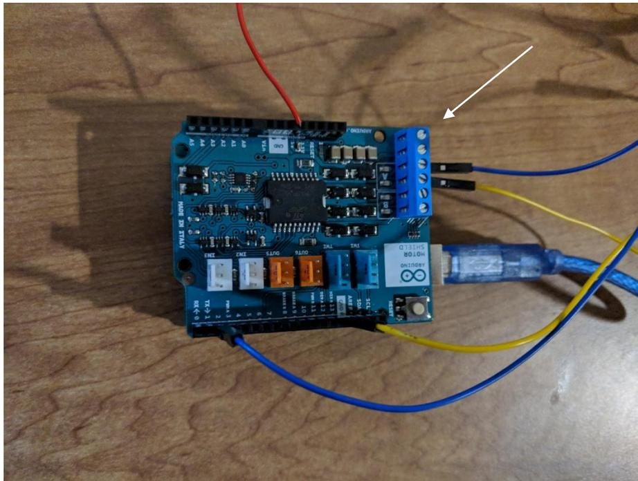
Figure 20: Control system without box, with the white arrow pointing to the connected motor
