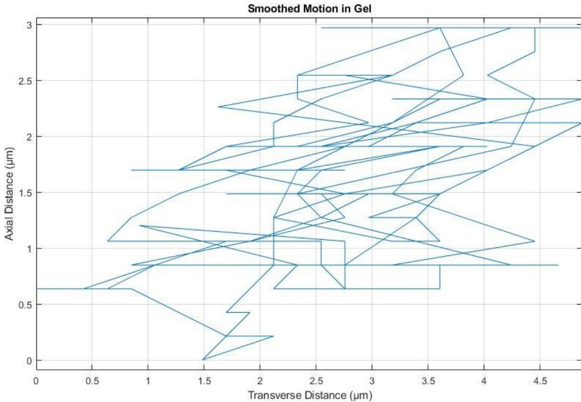
Figure 45: Motion of the needle while embedded in hydrogel tracked for two hundred points
