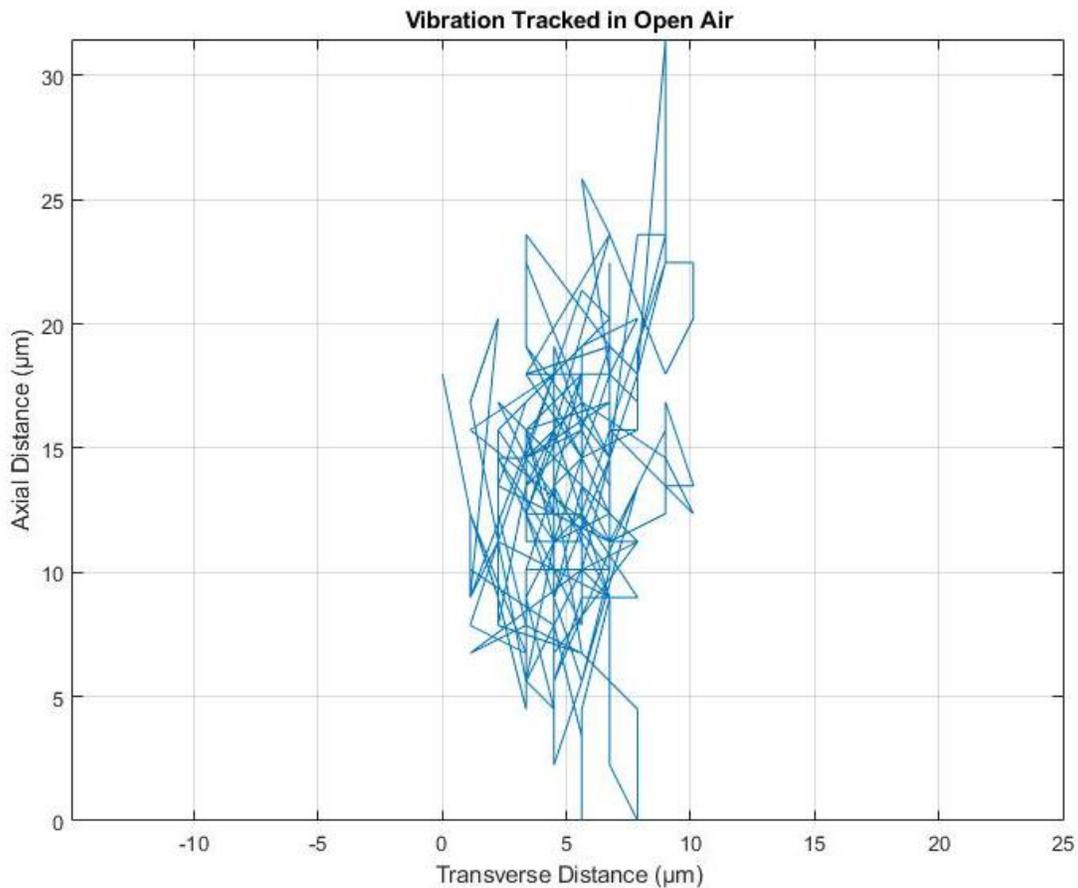
Figure 42: Vibration in open air tracked for two hundred points, with the needle coming from the left side of the image
