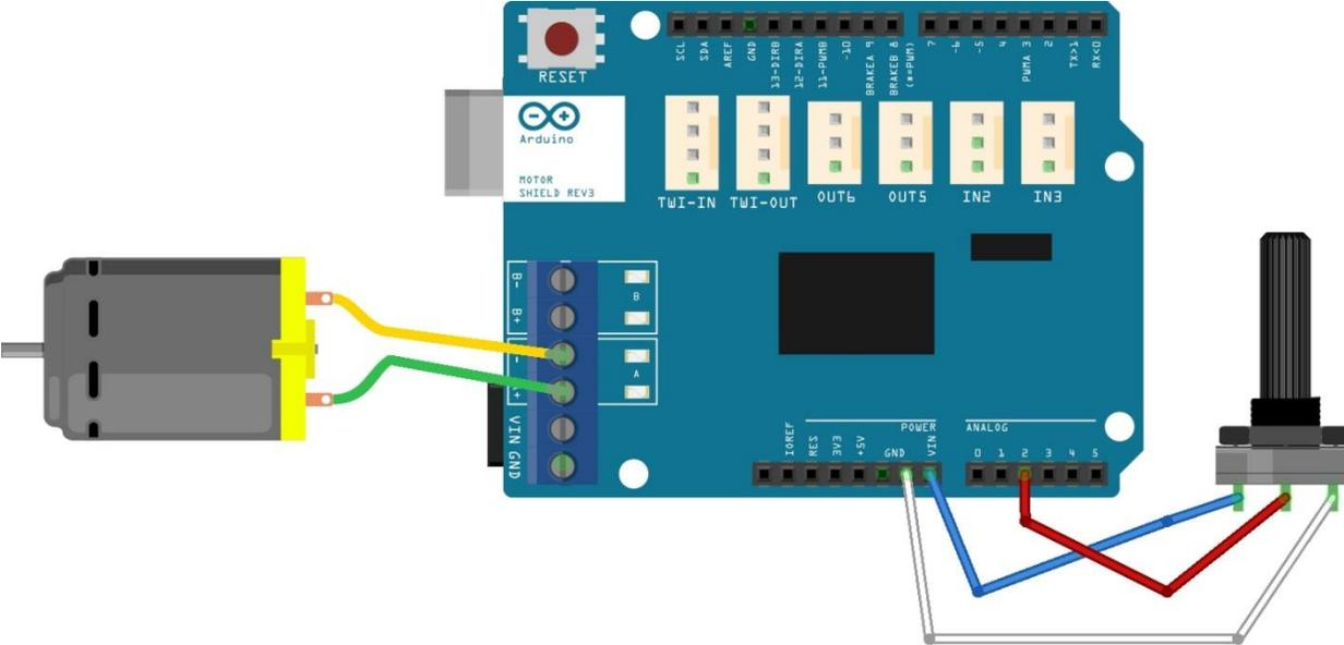
Figure 17: Diagram of the attached motor with potentiometer to vary the power
