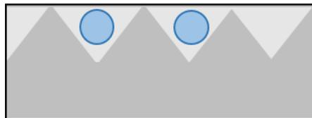
Figure 26: Example cross section, with the dark grey representing agarose and the light grey representing hydrogel
