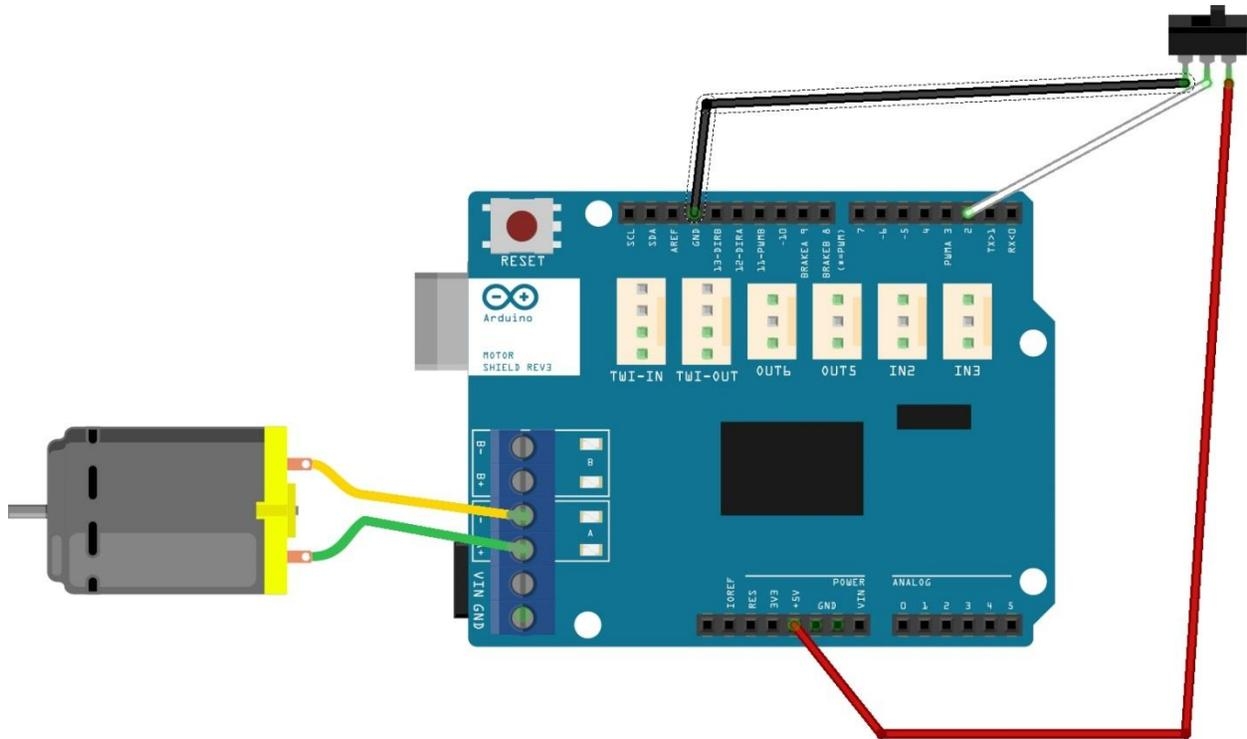
Figure 22: Schematic of the final design for the induced vibration, the motor representing the vibration motor and the switch representing the foot pedal
