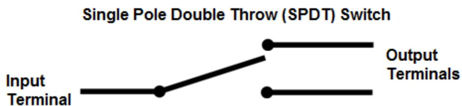
Figure 21: Example of single pole double throw switch [21]
