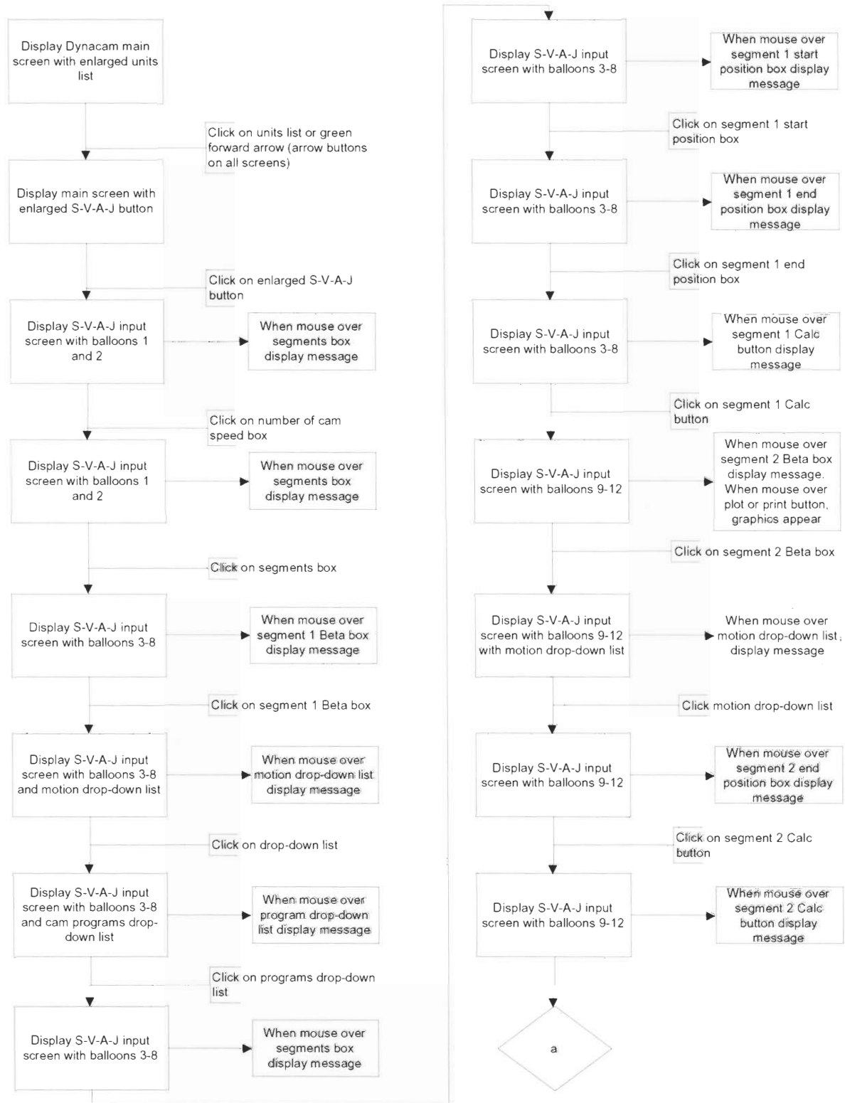
Figure 9 Part 1: Flow Chart for S-V-A-J Input
