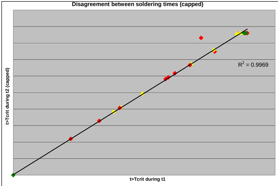
Figure 55: Plot comparing the time the mold is above 453.5C during the period MAGMA calculates the die solder module results (3-91s), capped at the dwell time; and the time the casting is in contact with the mold (filling + dwell time).
