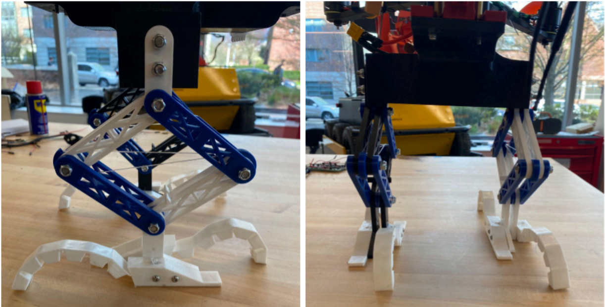
Figure 23: The final grasping mechanism, attached to the drone body. The left image shows a side view of the system, the right image shows the front view of the grasping mechanisms and lower drone body.
