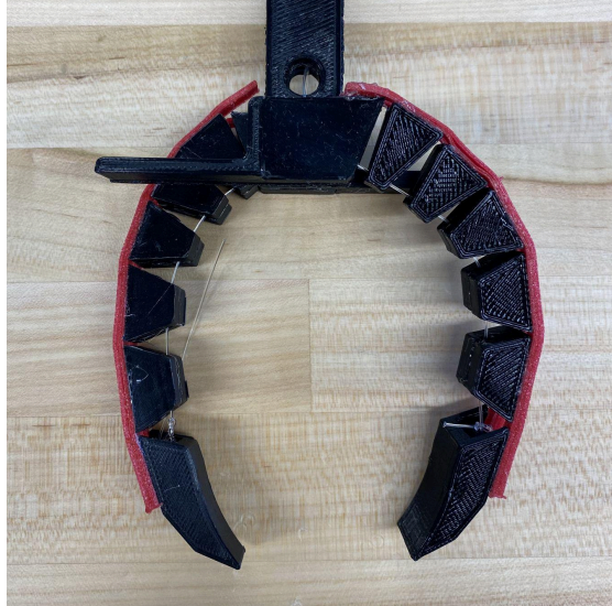
Figure 17: Initial prototype grasping mechanism talons made up of separate pieces of PLA and TPU compliant rails glued together with flexible adhesive.
