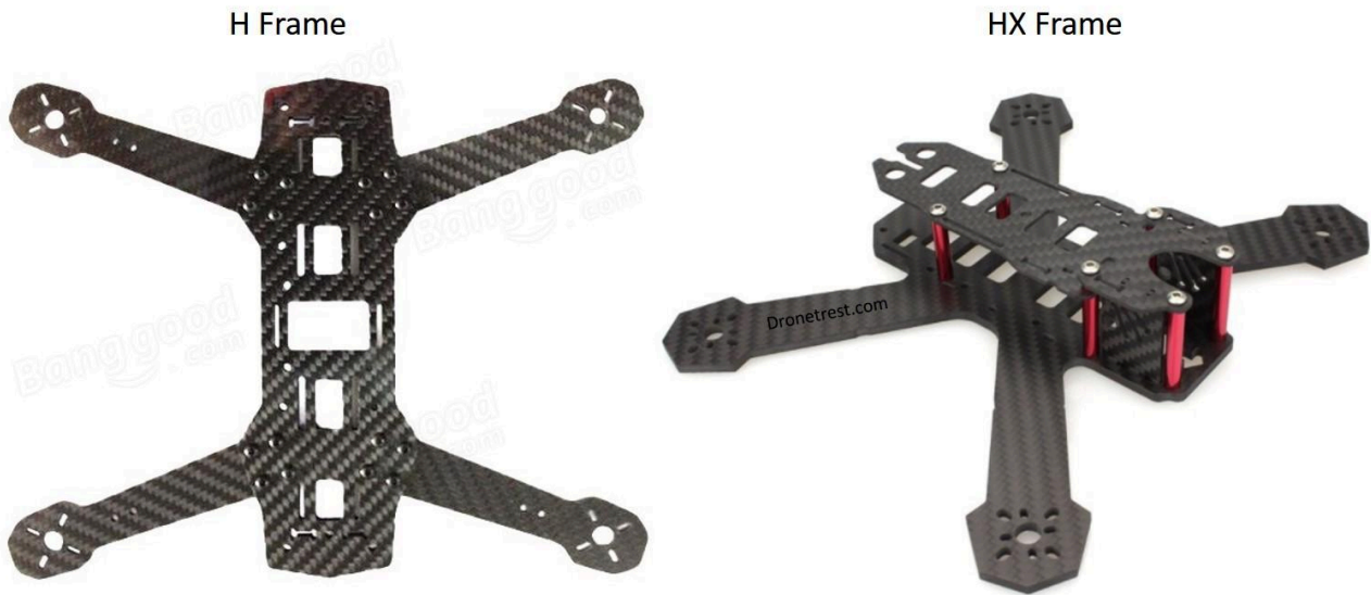
Figure 2: A comparison of H-frames vs HX-frames (Unmanned Tech, 2018)
