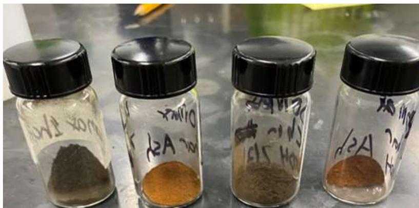
*Figure 5: Hydrochar Left to Right; Unmodified, Unmodified Ash, KOH Activated, KOH Activated Ash*
