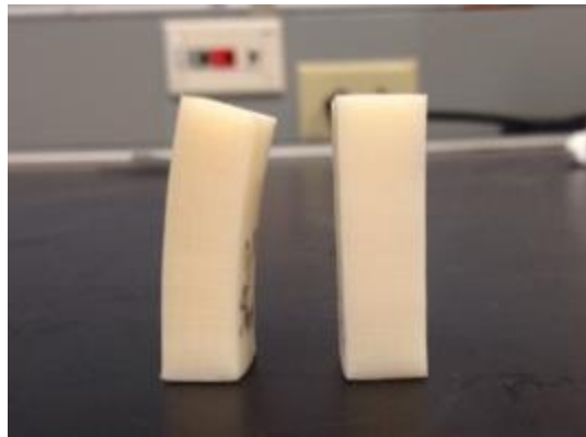
Figure 10: A sample annealed without a firebrick (left) and with a firebrick (right)
