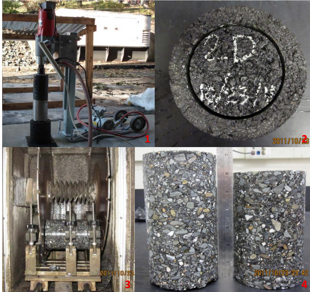
Figure 4. Coring and Cutting Process
