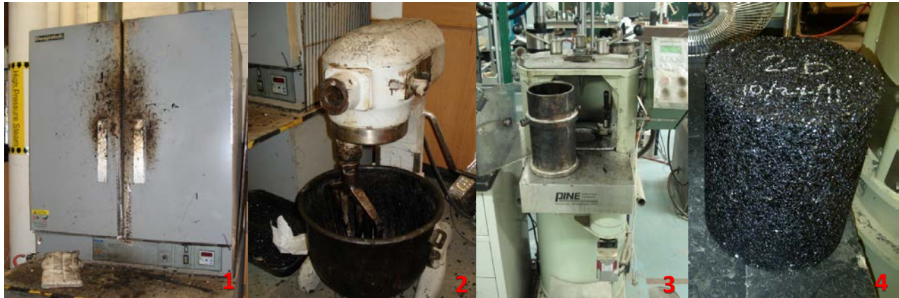
Figure 3. Warm Mixing and Compaction Process
