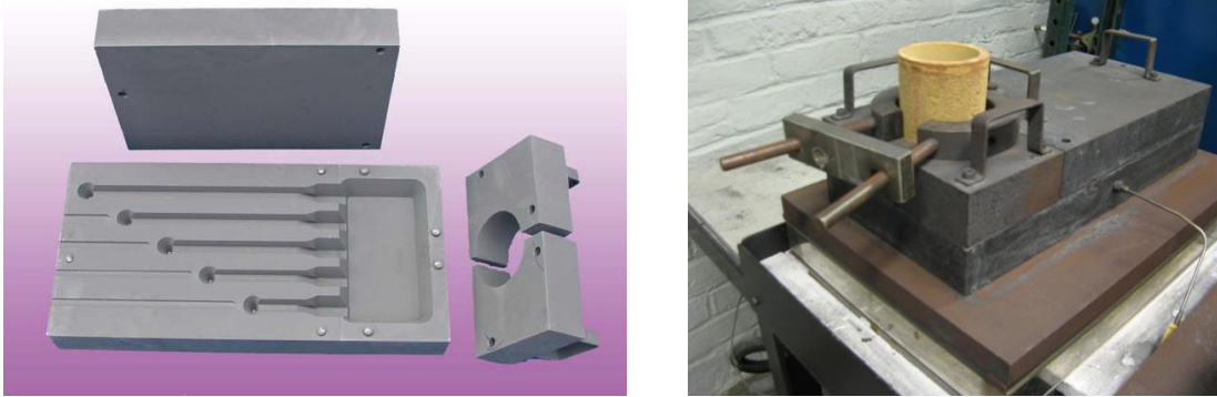
Figure 9: N-Tec hot tearing mold (a) and setup (b)*.
