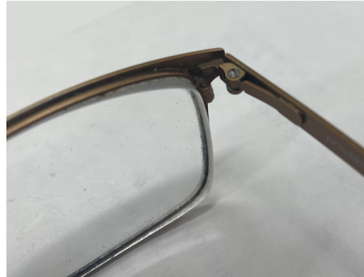
Figure 5: Close up of sprung hinge mechanism
