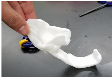
Figure 23: Prototype made of the fixed bent elbow attachment and J-shape ground interface with thermoform plastic. The thermoform was molded directly on Baxter to ensure accurate dimensions.
