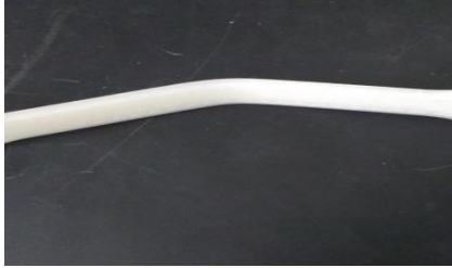
Figure 34: This image shows the plastic deformation of a nylon copolymer samples.
