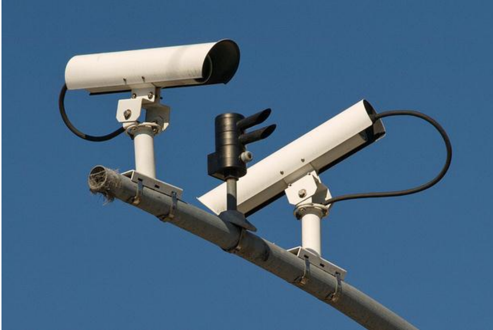
Figure 29: Opticom Receiver and detector on to traffic lights
