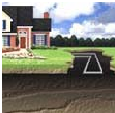
Figure 15 - A horizontal loop - (Alliant Energy)
