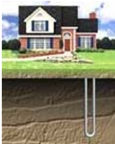
Figure 17 - A Vertical Loop - Alliant Energy
