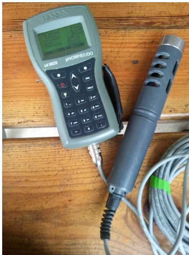
Figure 2: The HANNA HI 9828 multi-parameter probe
