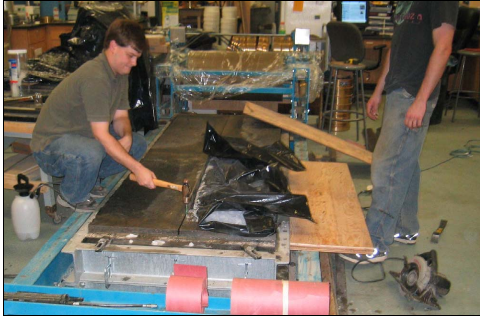
Figure 6.3 – Cutting, spreading, and movement of pavement slabs
