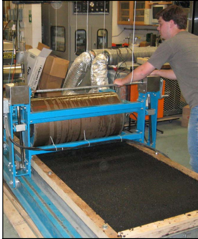
Figure 6.2 – Compaction of a pavement slab
