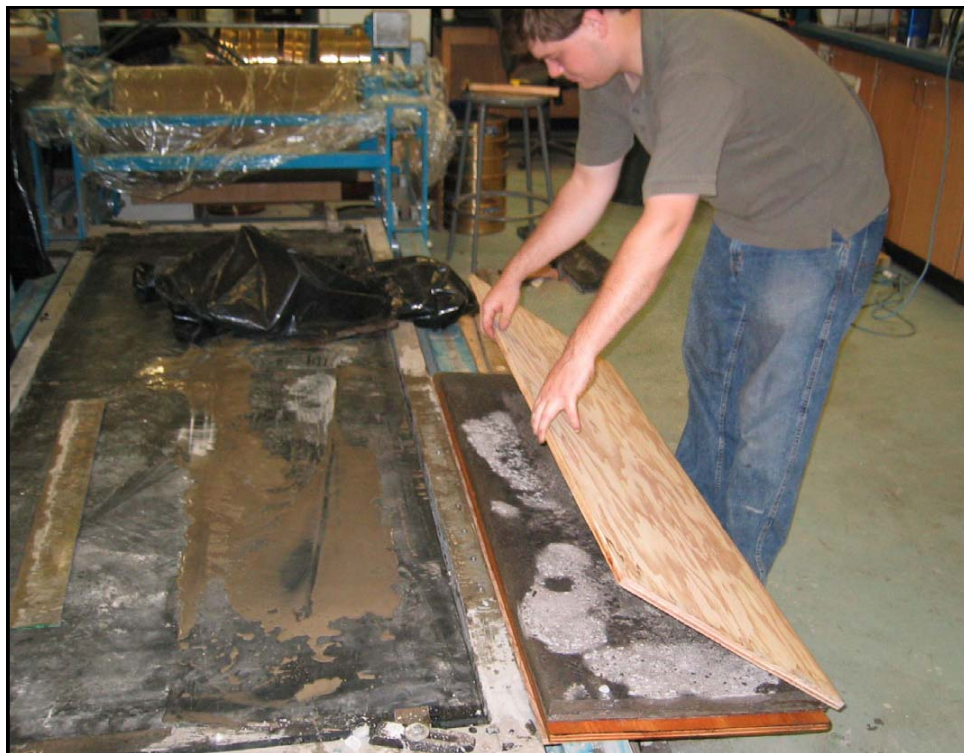
Figure 6.4 – Sandwiching pavement slab for transport, instrumentation, and storage
