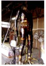
Burns to the lower extremities, visible on a tested firefighter's suit (above), register as torso burns via copper slug skin calorimeters on the mannequin (left). The suit is made from polybenzimidazole (PBI), a material used in most firefighters' suits. "Part of the reason for the extent of these burns," says Jay Kramarczyk '04, lab assistant in WPI's burn chamber, "is that the scenario the suit is exposed
