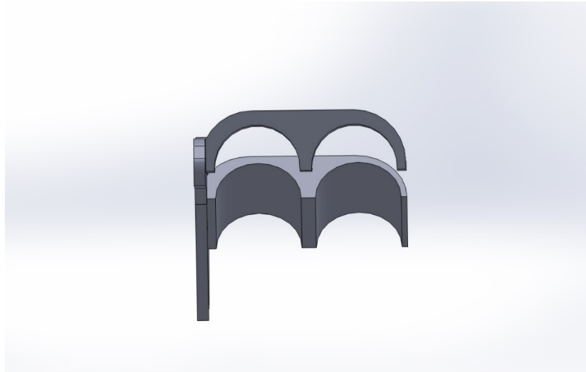
Figure 23 Front View of Finger Supports
