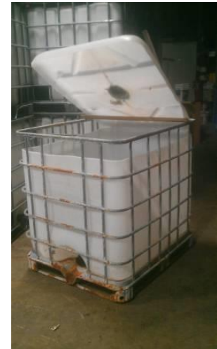
Figure 4. The IBC Tote was recommended to be used as a fish tank
