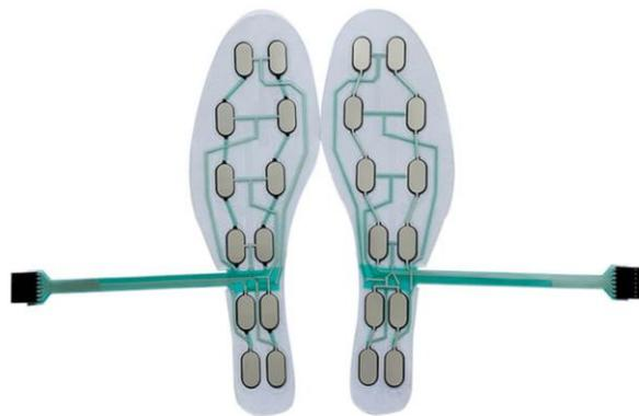
Figure 2.4: Foot Pressure Sensor
