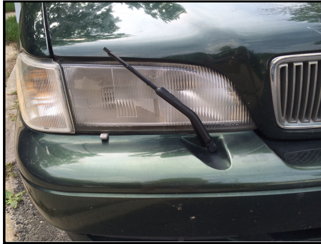
Figure 7: Volvo headlight wipers (Graz, 2015).
