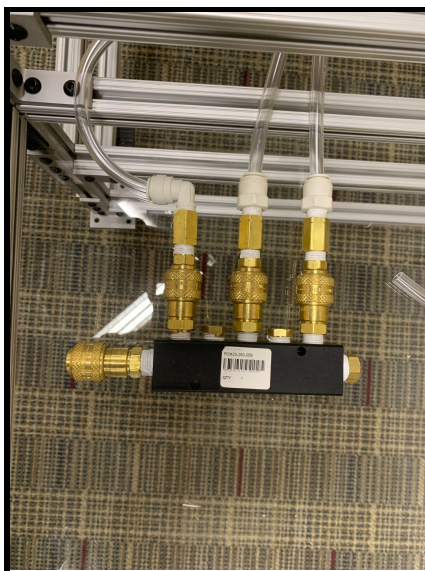
Figure 54: Pressure Manifold for Venturi and Prototype.
