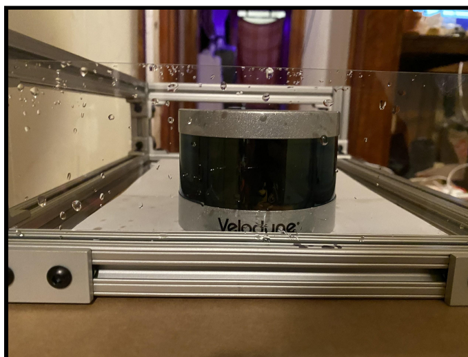
Figure 16: Test 2, Set up of Some Droplets on Glass.
