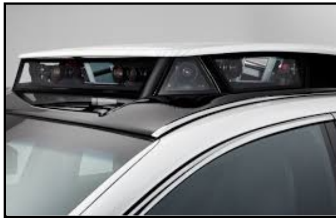
Figure 11: Sensor Position on Car (Hanson J, Bourgoise R, 2019).
