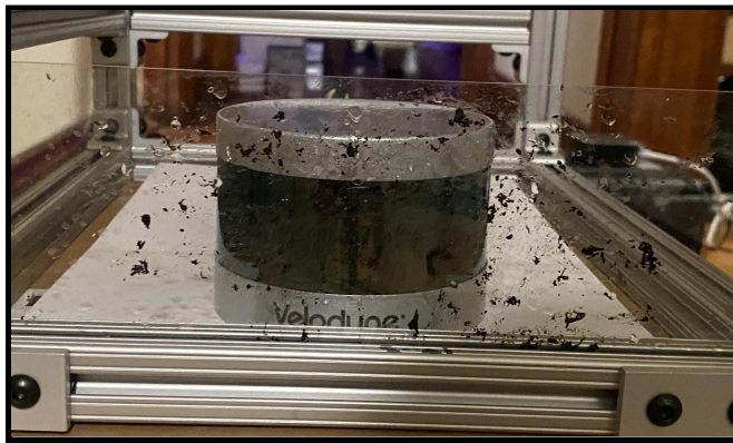
Figure 20: Trial 4, Set up of Dirt on Glass.
