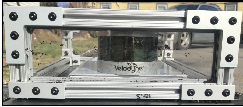
Figure 22: Trial 5, Set up of Dirt Smeared onto Glass.
