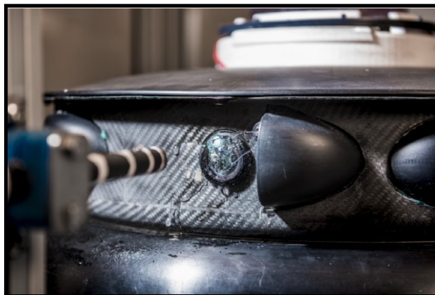
Figure 6: Ford's High-Velocity Bug Shooter (Company, F.M, 2019).
