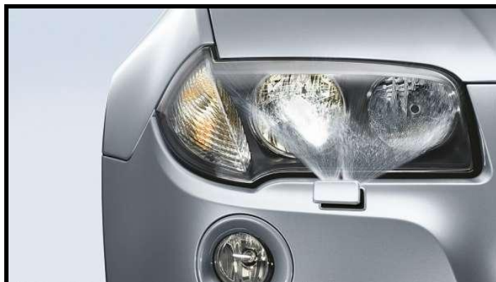
Figure 117: BMW's Retractable Headlight Cleaner (Dunn, 2020).
