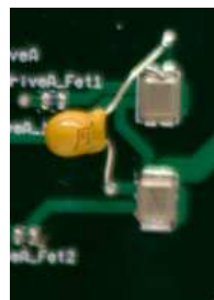
Figure 5.9: Addition of Tantalum Bypass Capacitor at MOSFET
