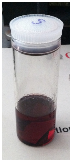
Figure 35: Gold slides in porphyrin solution, post MUA solution
