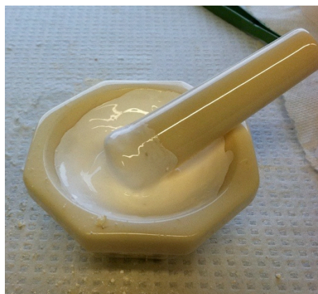
Figure 30: Mixture of titanium dioxide and 1% acetic acid solution.
