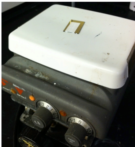
Figure 32: Grätzel Cell on hot plate, prepared to be sintered
