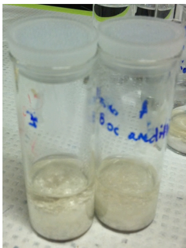
Figure 36: Gold slides in cleaning solution post dithiol attachment
