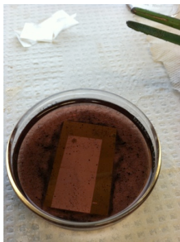
Figure 33: Grätzel Cell in porphyrin solution.
