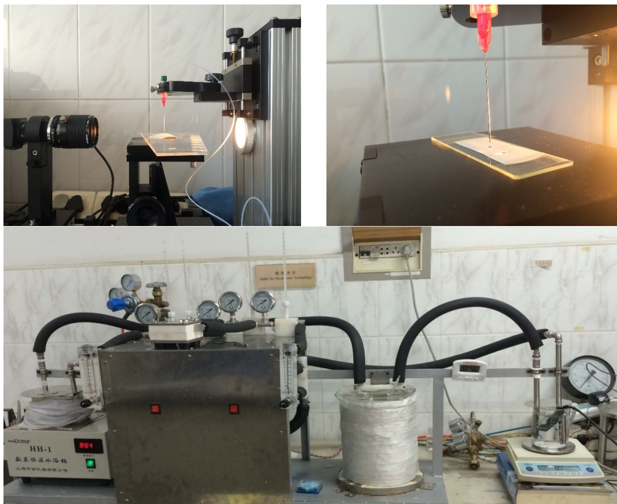
Figure 7A. Goniometer measuring the contact angle of modified and virgin membranes. B. Direct contact membrane distillation configuration.
