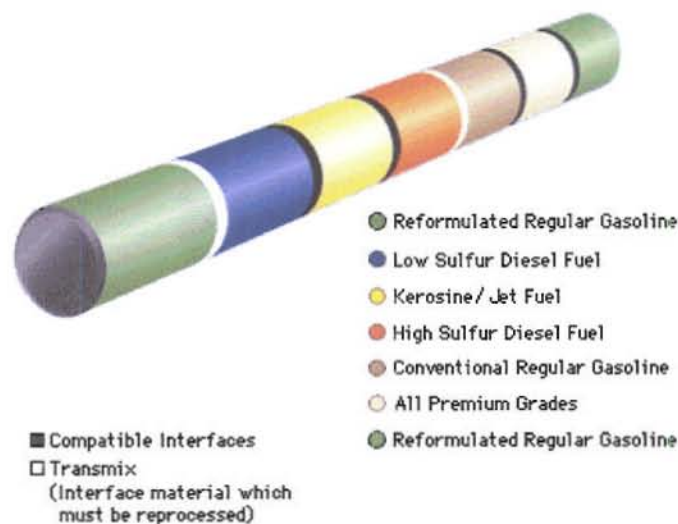
Figure VI: Transmission of Petroleum Products through Pipelines (Source: Colonial Pipeline Frequently Asked Questions ) 56
