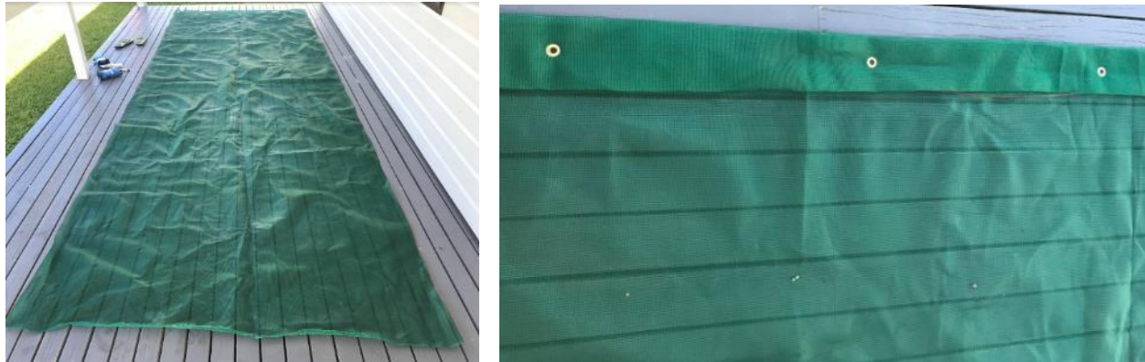
Figure 59: Mesh before and after grommet addition
