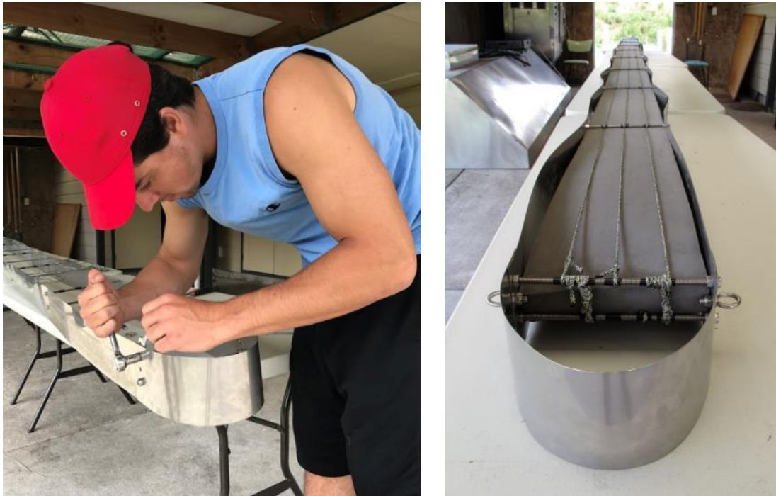
Figure 58: Addition of the nosepiece and extra nylon
