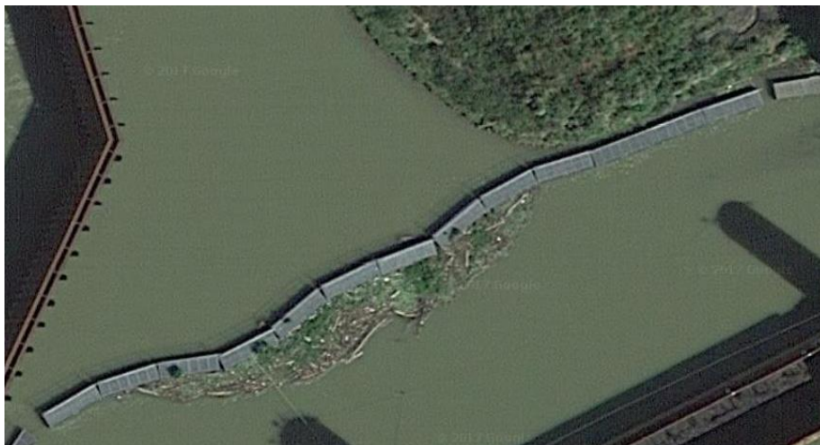
Figure 21: Aerial view of full-scale floating boom in action at Clifty Creek Power Plant (Google Maps, 2017)
