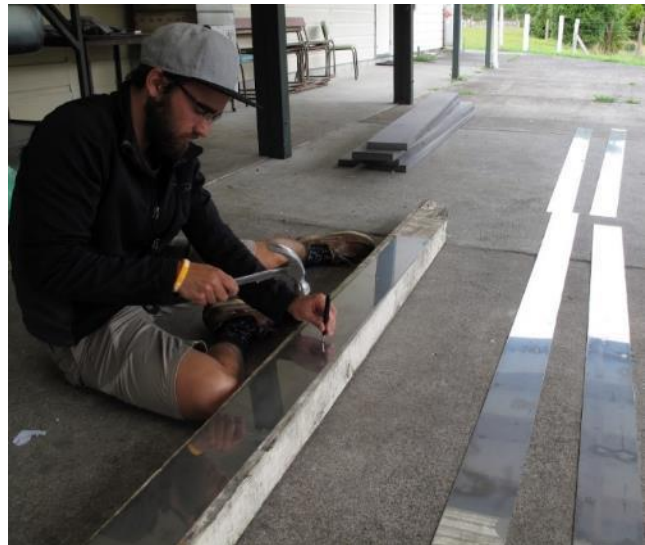
Figure 49: Aaron prick-punching the sheet metal
