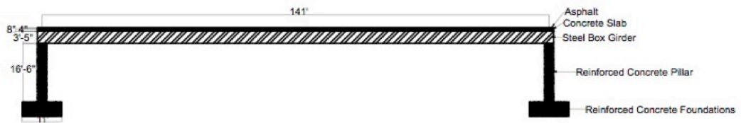
Figure 19: Single span, steel box girder bridge (Case #2).
