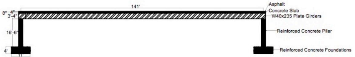
Figure 18: Single span, steel plate girder bridge (Case #1).
