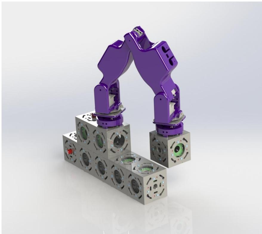
Figure 14. SMAC 3.0 system consisting of the new smart blocks and RAINSTORM inchworm.
