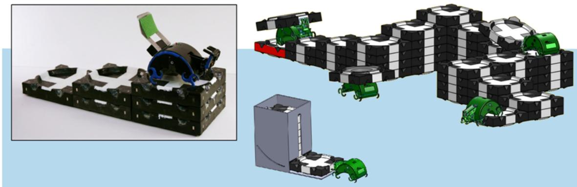
Figure 1. A small TERMES structure and robot (left) and simulated construction of a larger structure by multiple robots (right).
