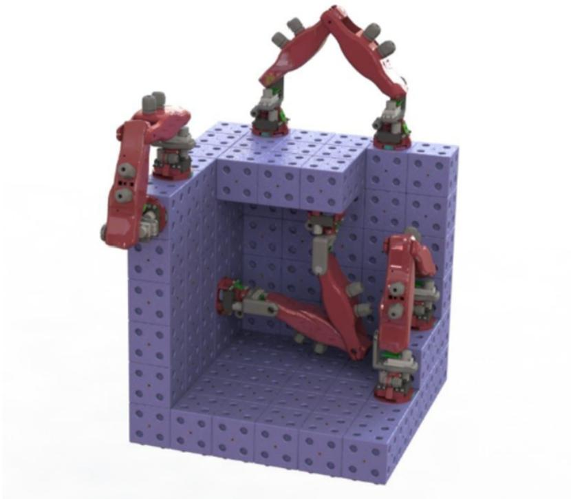
Figure 8. Simulation of multiple inchworm robots traversing multiple planes while building a structure. [9]
