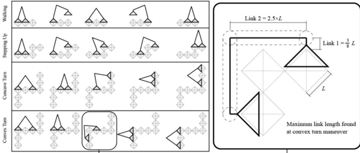
Figure 3. Robot positioning variations based on DOF functional requirements for BILL-E.
