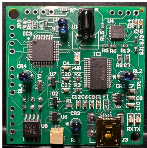
Figure 24. Custom 328p microcontroller board.
