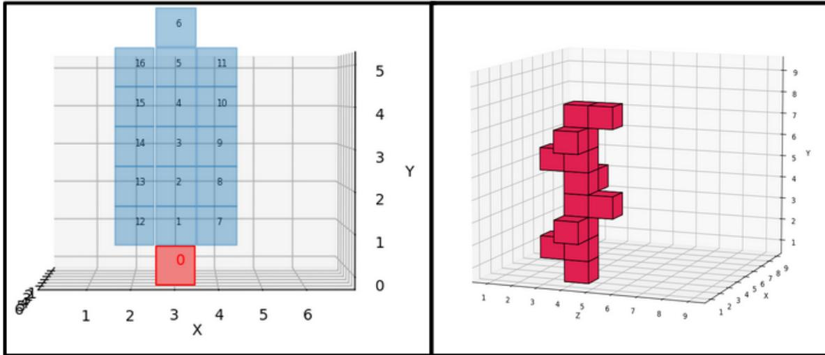
Figure 31. Left: Structure failing weight validation with 16 blocks all supported by one block. Right: A passing structure with 14 held on one block.
