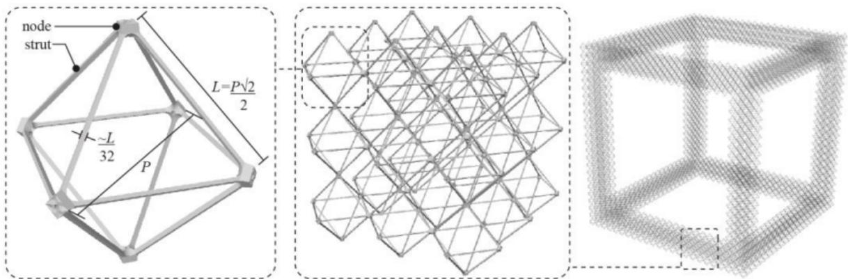
Figure 2. A cubic lattice structure composition and geometry
