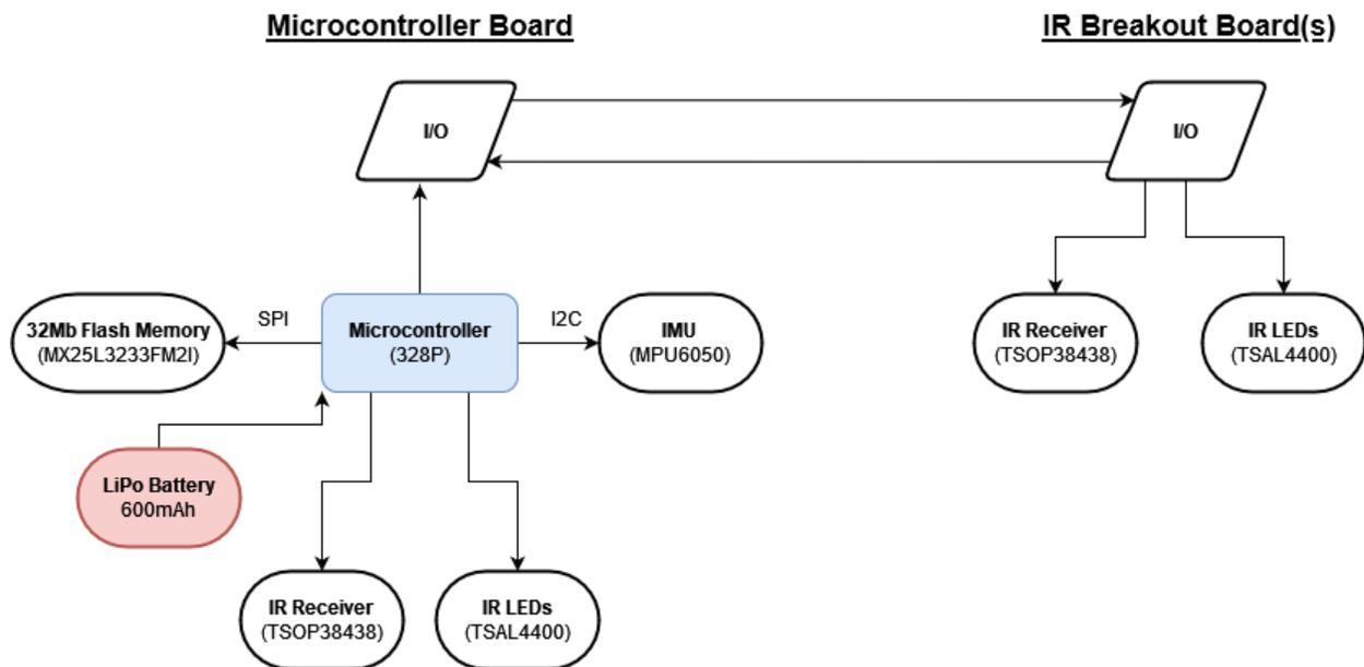
Figure 25. Block diagram of a smart block's electronics.
