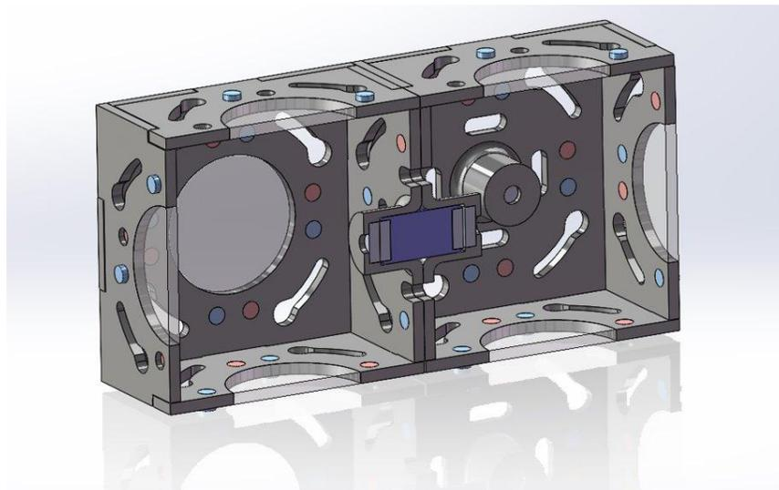
Figure 18. Hybrid Block Design, section view.
