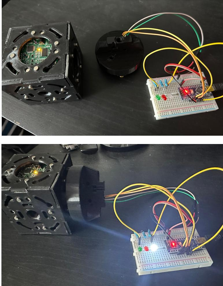
Figure 28. Before (top) and after (bottom) connecting the EE tool to the “correct” face of a block.
