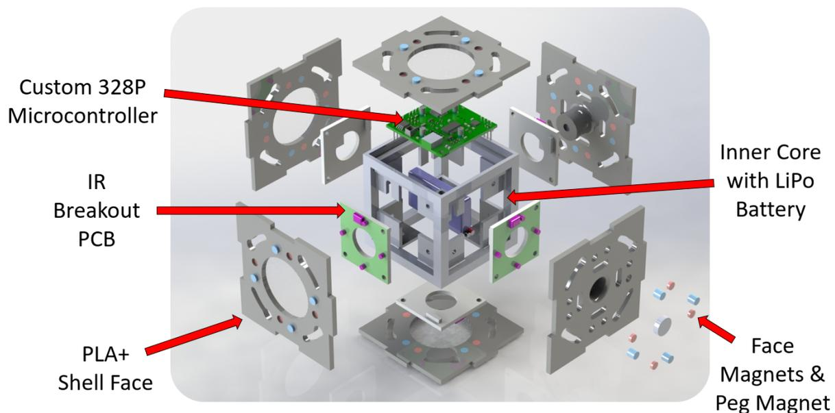
Figure 20. Exploded assembly of final block design and its components.
