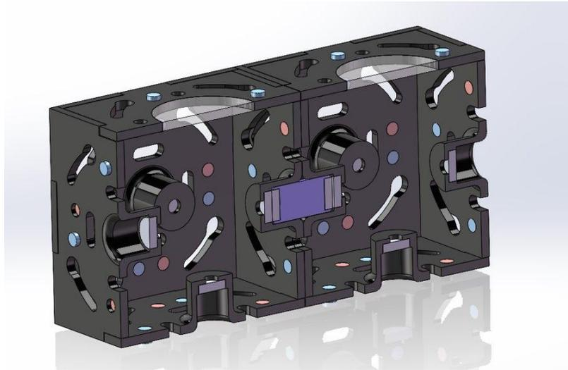
Figure 17. Removable Peg Design, section view.
