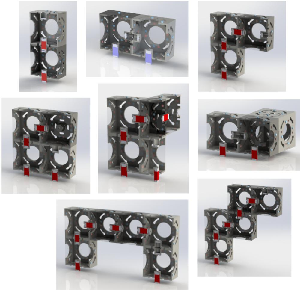
Figure 19. Basic substructures with strong-link configurations colored in red. From left to right: Simple Top, Simple Side, Vertical Corner, Vertical Corner 2, Vertical Corner 3, Ground Corner, Overhang, Doorway, Inverted Staircase.
