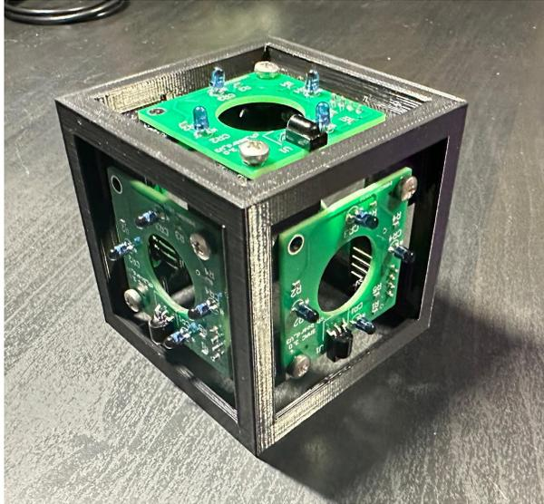
Figure 23. Smart block inner core with breakout boards attached.
