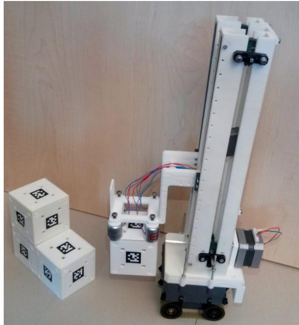
Figure 5. BeBot robot manipulation a SRoCS block.
