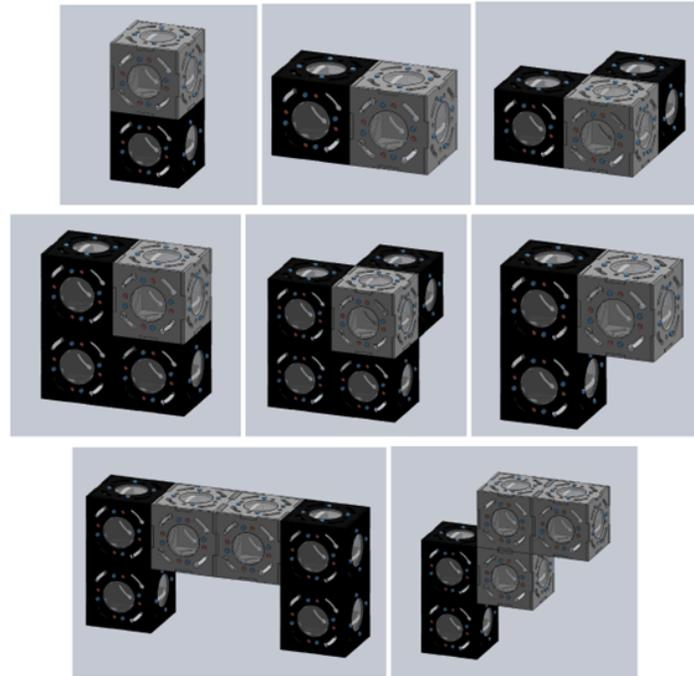
Figure 11. Some of the potential structures that are possible with the magnet connections
