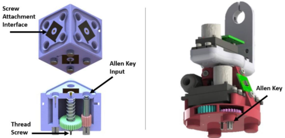
Figure 9. CAD model of the proposed block design with 5 female sides and a single male side seen on the bottom of the left image [9]
