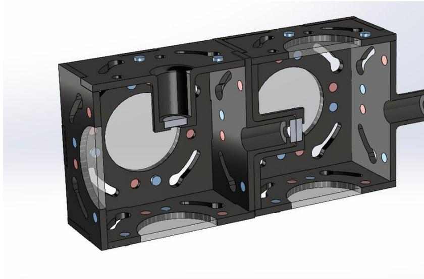
Figure 16. Permanent Peg Design; 90° block (left) and 180° block (right), section view.
