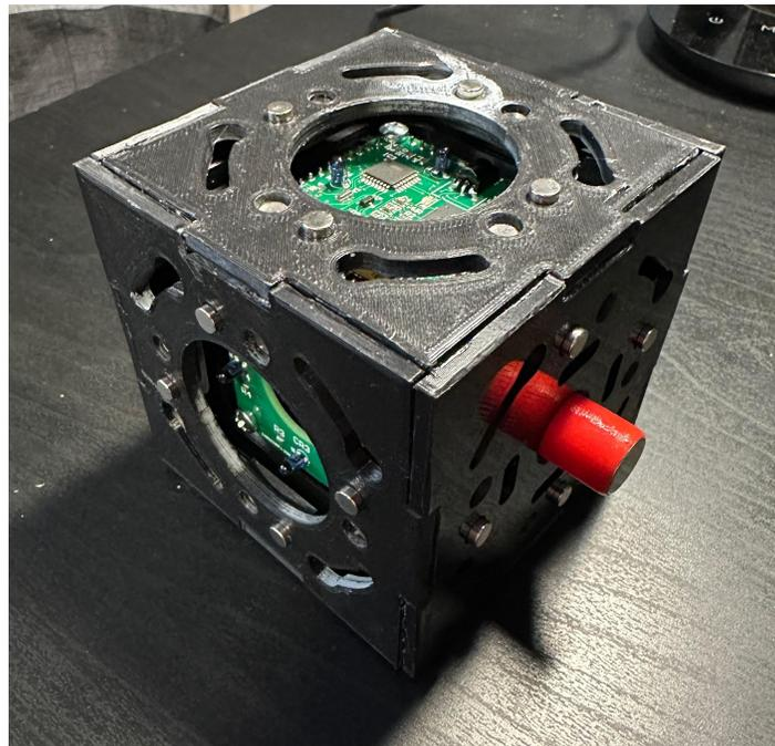
Figure 15. SMAC 3.0 smart block fully assembled, with a peg inserted.
