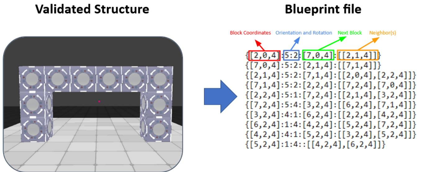
Figure 36. Validated block structure with corresponding blueprint.
