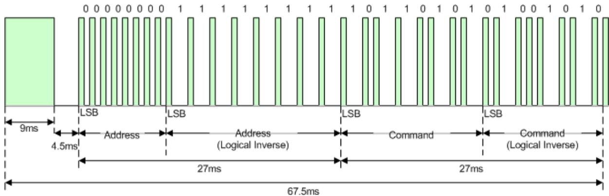
Figure 21. Message frame for the NEC protocol, courtesy of Altium Ltd. [11]
