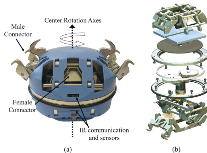
Figure 7. The ATRON self-reconfigurable robotic module and its exploded mechanical assembly.
