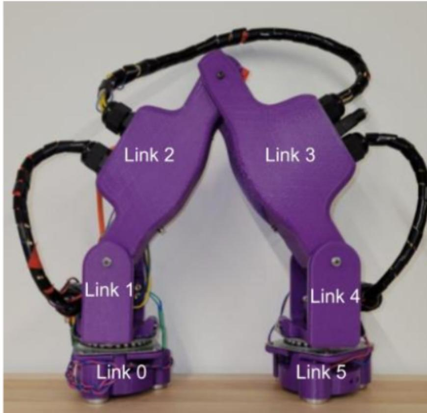
Figure 13. RAINSTORM altered linkage design with labeled links [10]
