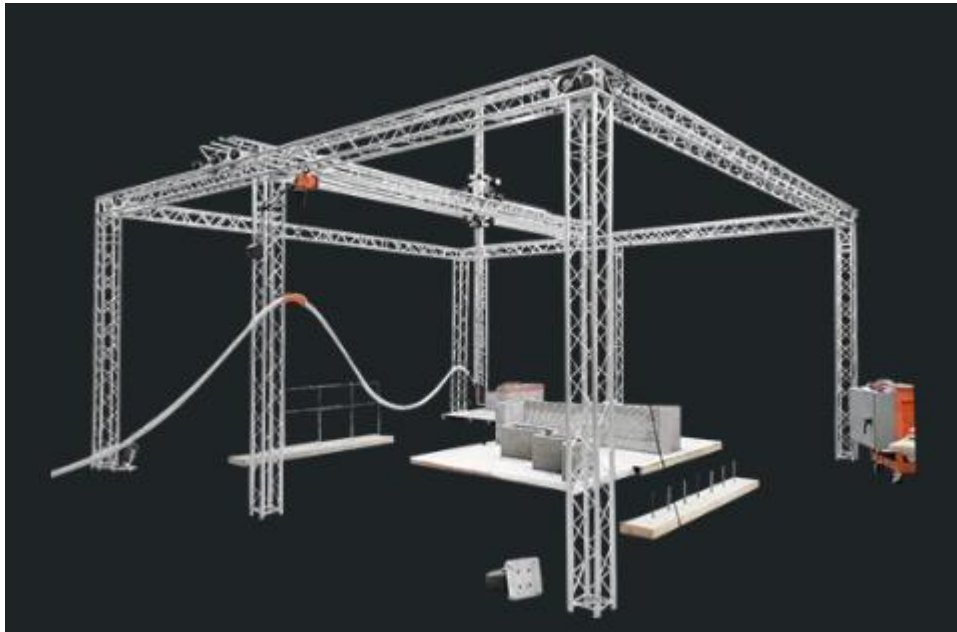
Figure 1: Mudbot gantry style concrete 3-D printer
