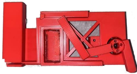
Figure 30: Final Iteration of the Brick Placer Mechanism
